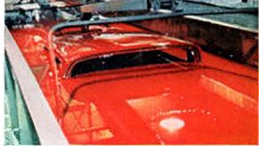
Greatest rust fighter is Rambler's Deep-Dip rustproofing-with entire body immersed right up to the roof in rustproofing compound for longer protection against rust. That's Rambler Excellence.
