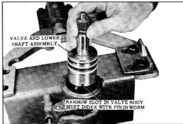
Fig. 4-65 Installing Valve and Lower Shaft Assembly
