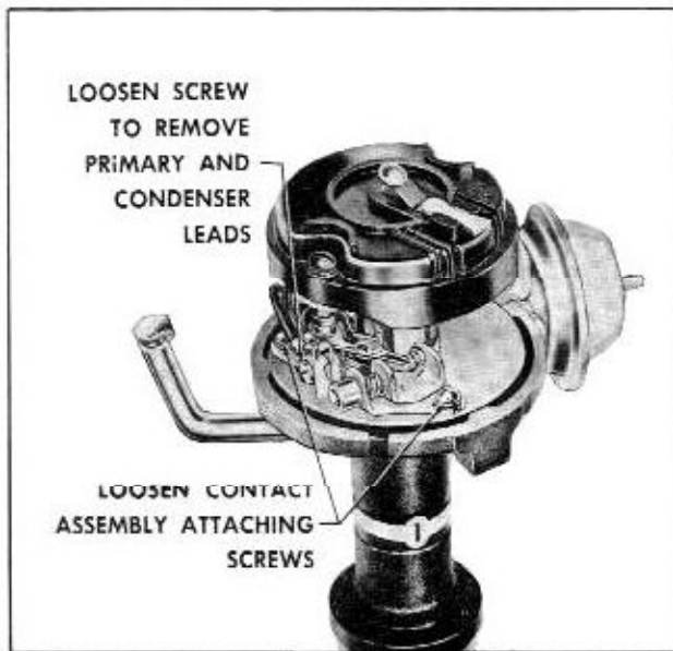
Fig. 13-61 Removing Contact Point Set
