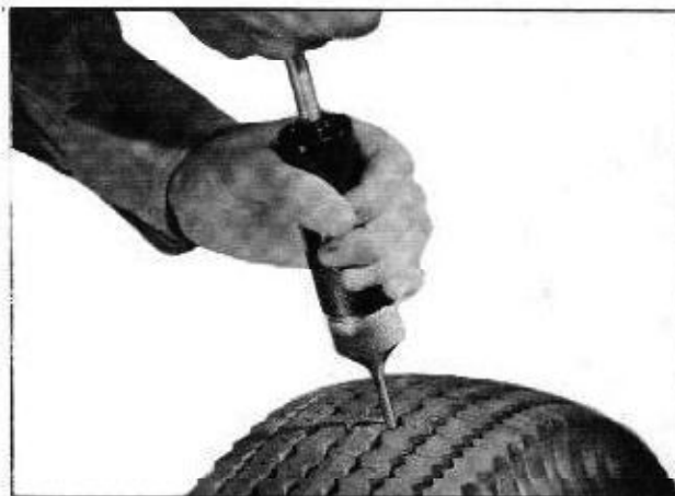
Fig. 5-29 Using Sealer Gun
