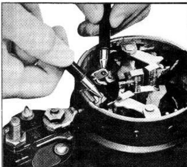
Fig. 13-49 Checking Shunt Coil for Open
