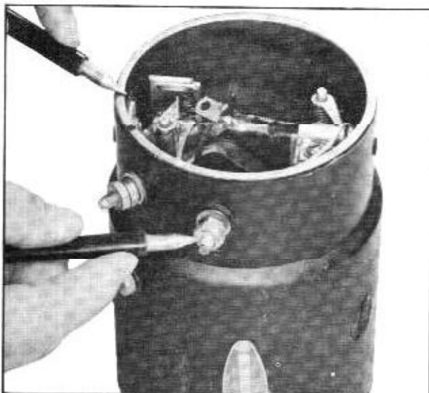
Fig. 13-32 Checking Field Coils for Ground
