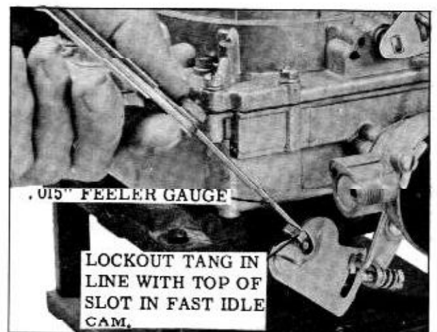
Fig. 8-127 Secondary Throttle Lock-Out Adjustment
