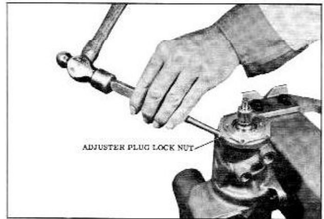
Fig. 4-44 Loosening Lock Nut
