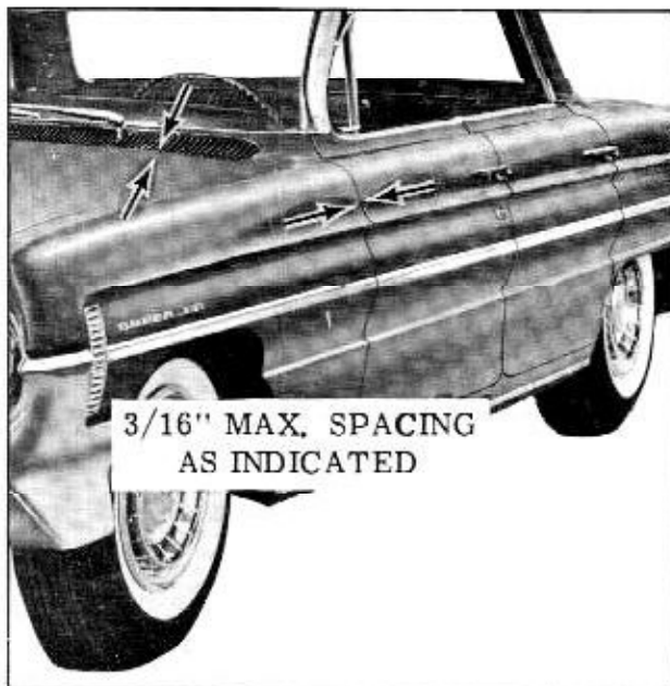
Fig. 16-2 Sheet Metal Clearances
