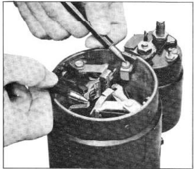
Fig. 13-47 Checking Field Coil for Open
