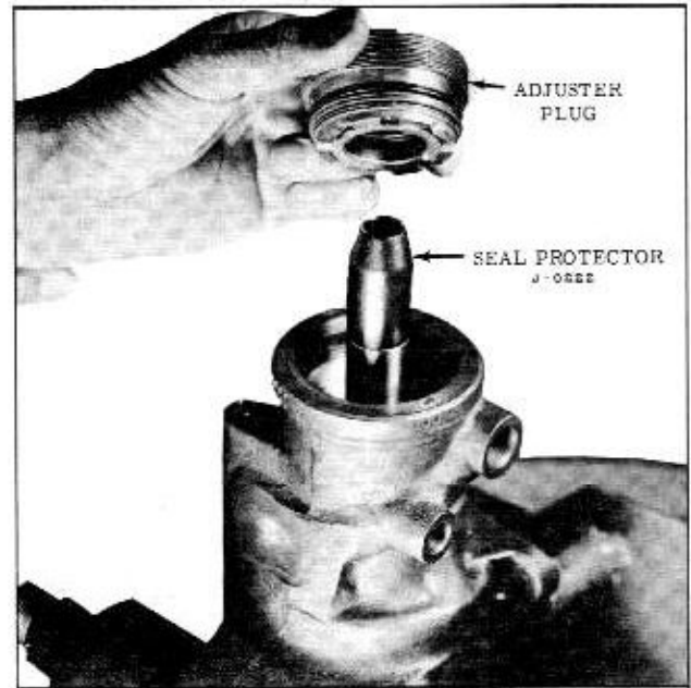
Fig. 4-67 Installing Adjuster Plug
