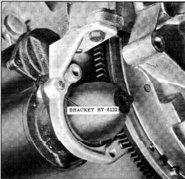
Fig. 8-75 Starter Bracket Installation
