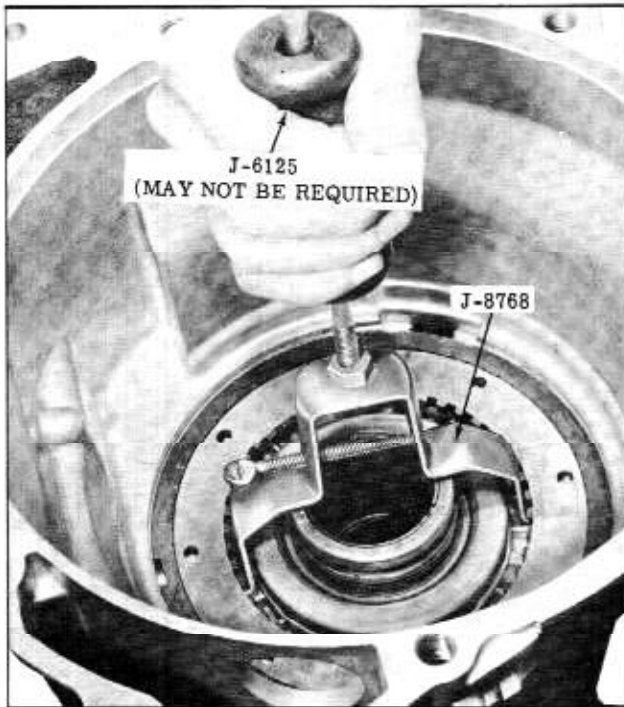
Figure 3-53 Removing Reverse Cone
