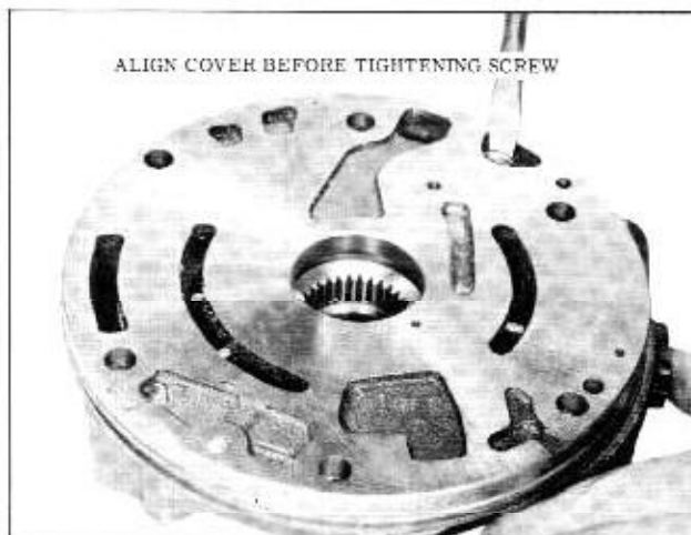
Fig. 3-66 Installing Pump Cover
