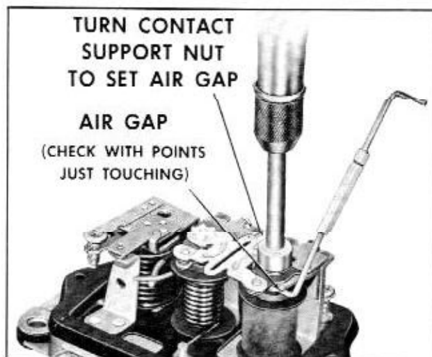
Fig. 13-39 Adjusting Voltage Regulator Air Gap (35 Amp.)
