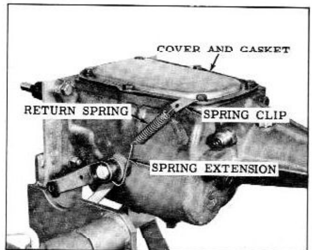
Fig. 11-7 Return Spring Assembly
