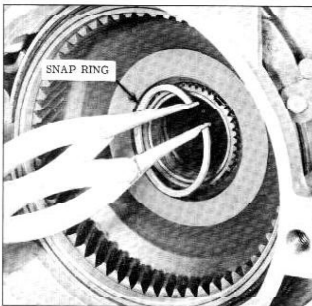
Fig. 3-105 Installing Internal Gear Snap Ring
