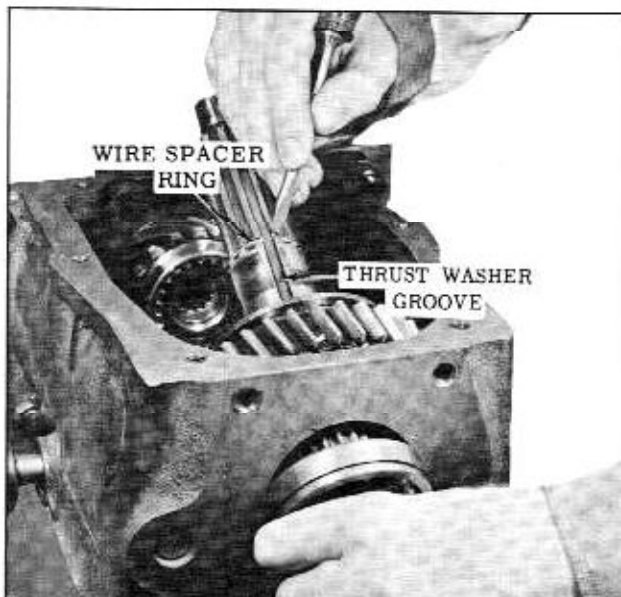
Fig. 11-31 Lining Up Wire Spacer Ring
