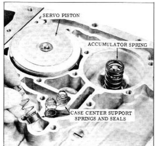
Fig. 3-129 Installing Seals and Springs
