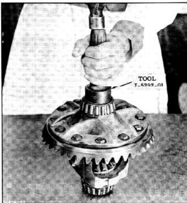
Fig. 6-26 Installing Side Bearings
