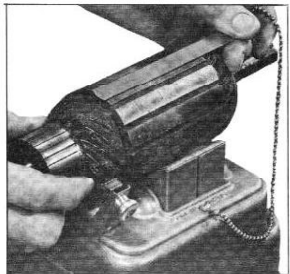
Fig. 13-29 Checking Armature for Short
