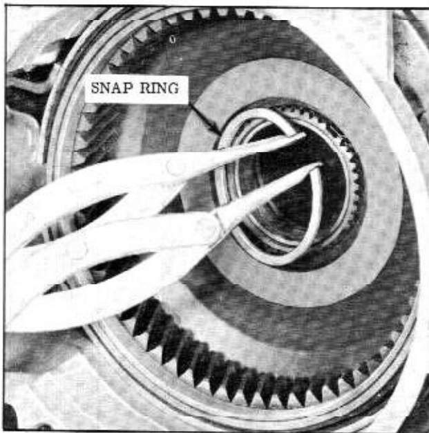
Figure 3-49 Removing Internal Gear Snap Ring
