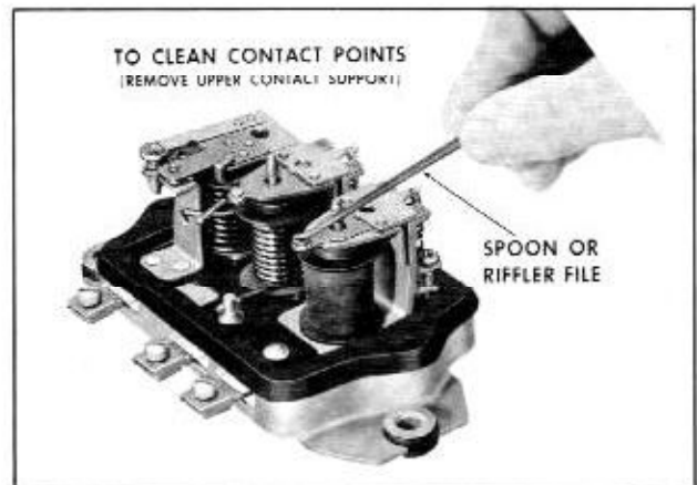
Fig. 13-35 Cleaning Contact Points
