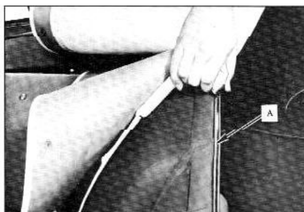
Fig. 17-108 Sliding Boot into Retainer
