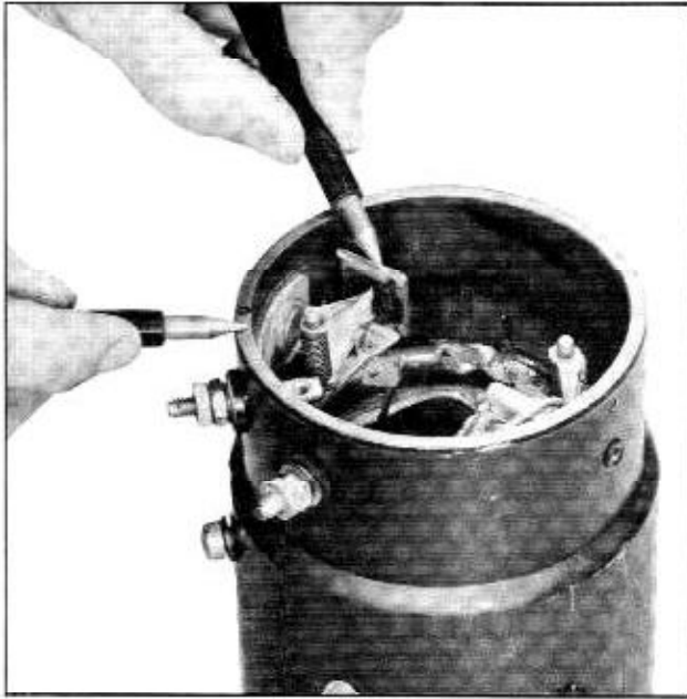
Fig. 13-34 Check Brush Holder for Ground
