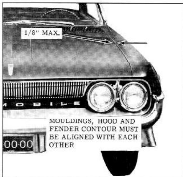
Fig. 16-3 Hood to Fender Clearances
