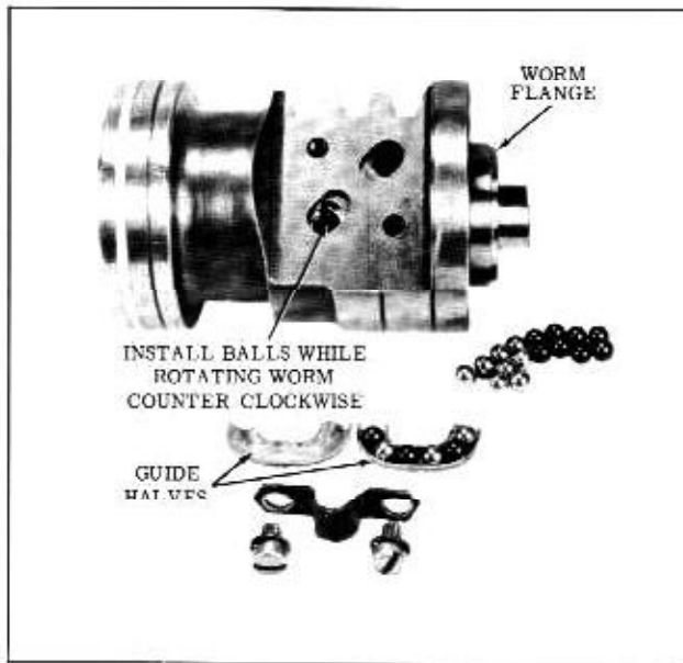
Fig. 4-91 Installing Balls in Rack Piston
