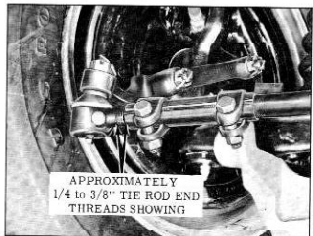
Fig. 4-47 Installing New Tie Rod End
