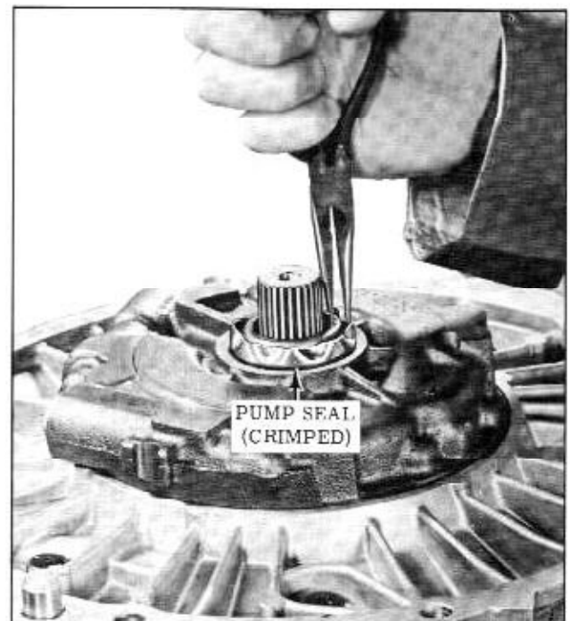
Fig. 3-40 Removing Pump Seal
