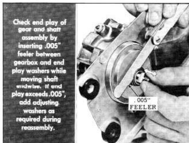
Fig. 13-122 Gear Shaft End Play
