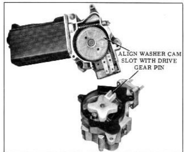
Fig. 13-123 Alignment of Cam Slot
