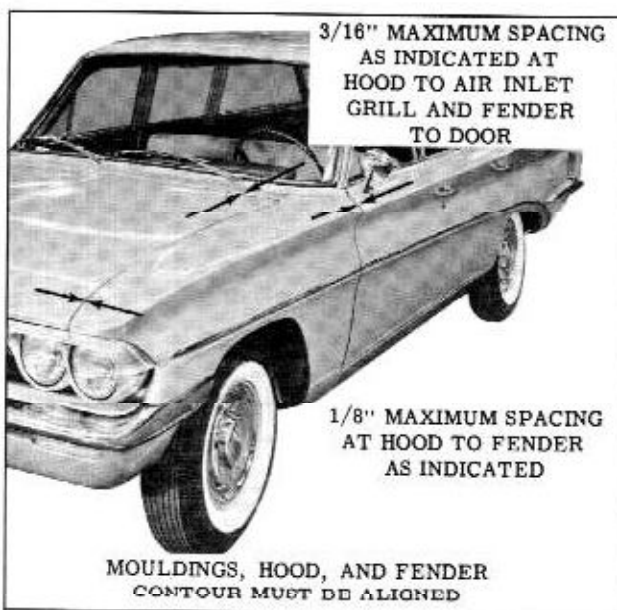
Fig. 11-3 Hood and Fender Clearances
