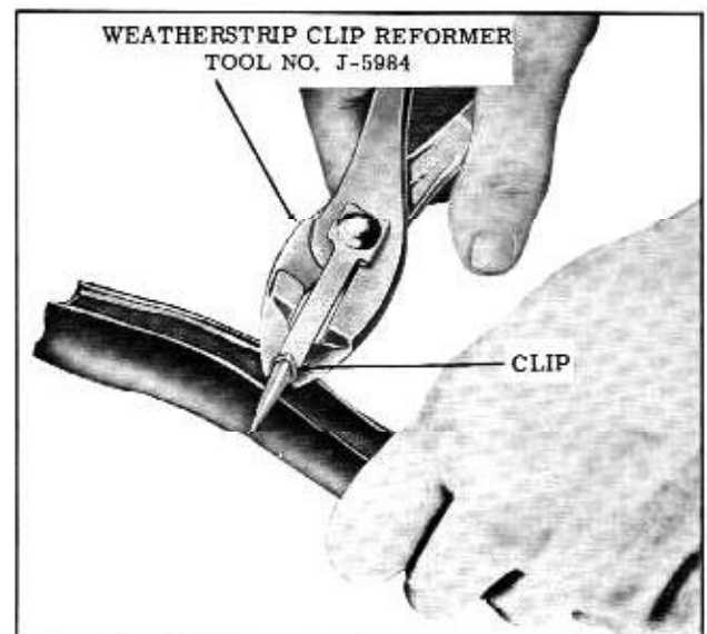
Fig. 15-57 Reforming Weatherstrip Clips with Tool J-5984
