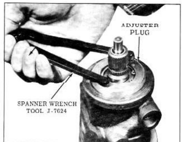
Fig. 4-77 Removing Adjuster Plug
