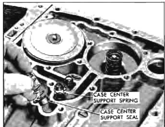
Fig. 129 Installing Case Center Support Seals and Springs
