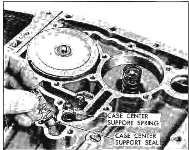
Fig. 44 Removing Case Center Support Seals
