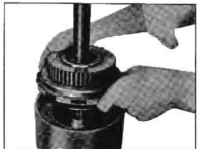
Fig. 72 Removing Rear Clutch Cylinder and Sprag Assembly
