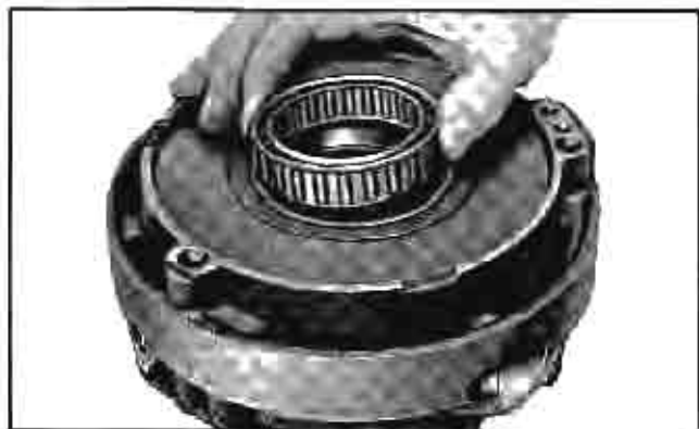
Fig. 116 Installing Front Sprag in Hub of Pump Body
