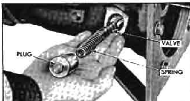
Fig. 162 Installing Pressure Regulator
