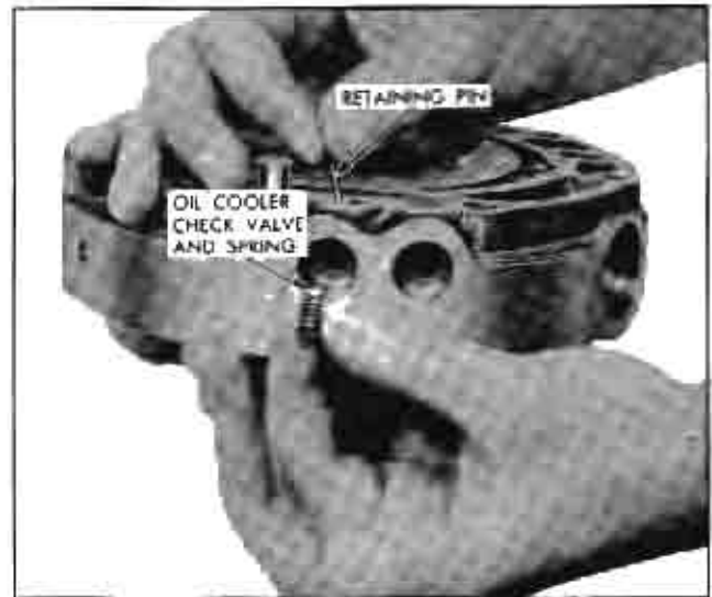
Fig. 114 Installing Oil Cooler Check Ball
