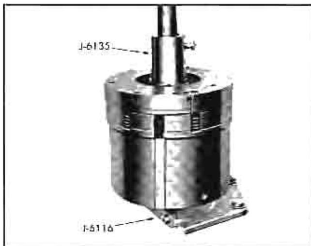
Fig. 100 Installing Rear Unit Clutch Retainer
