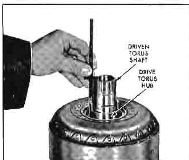
Fig. 163 Measuring Wear of Coupling Thrust Washer
