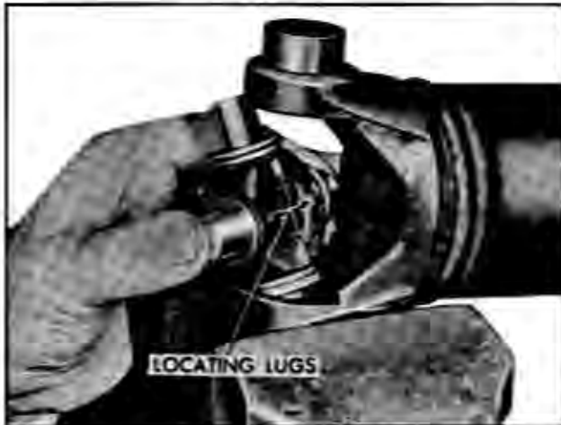
Fig. 4A-8 Correct Installation of Journal to Yoke
