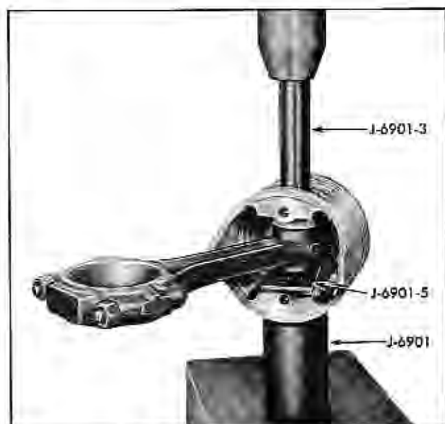
Fig. 6-68 Piston Positioned in Arbor Press for Removal of Pin
