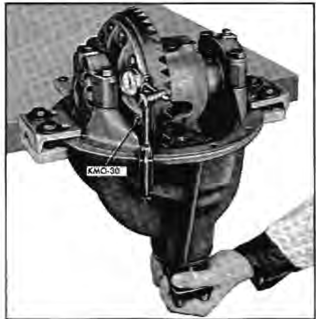
Fig. 4-60 Checking Ring Gear Run-out with KMO-30 Set
