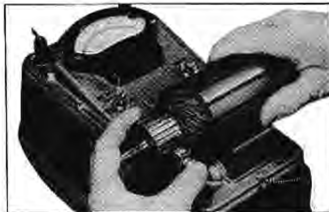
Fig. 11-13 Bar-to-Bar Test for Open Armature
