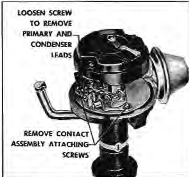
Fig. 11-59 Distributor Contact Details
