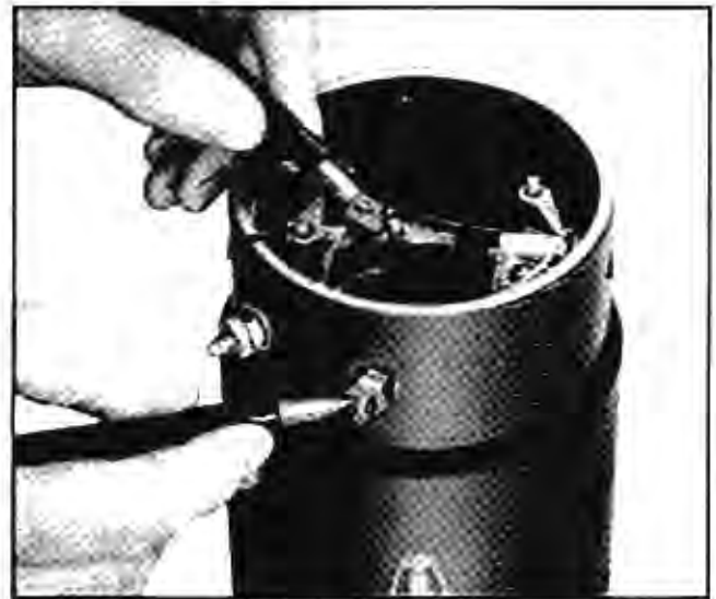
Fig. 11-15 Testing Field Coils for Open Circuit
