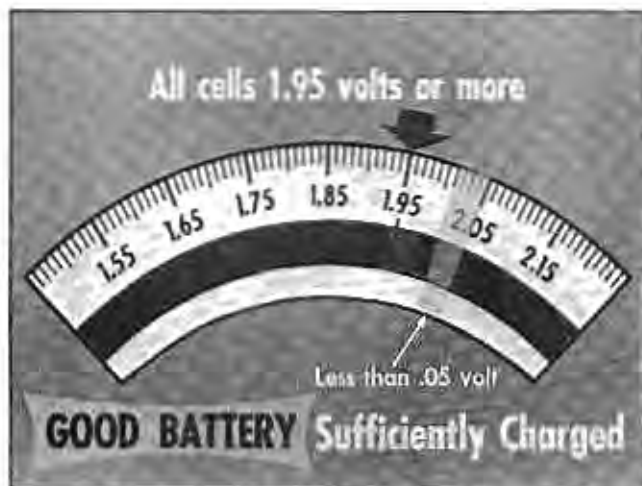
Fig. 11-5 Good Battery—All Cells 1.95 Volts or More
