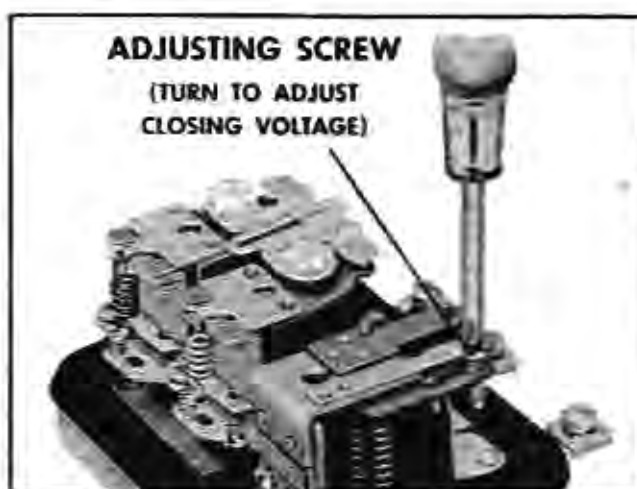
Fig. 11-29 Adjusting Closing Voltage
