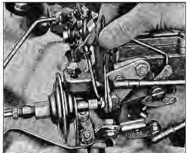
Fig. 6B-3 Using Drill to Measure Throttle Return Check Setting (Four Barrel)
