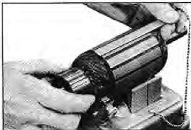
Fig. 11-12 Testing Armature for Shorts
