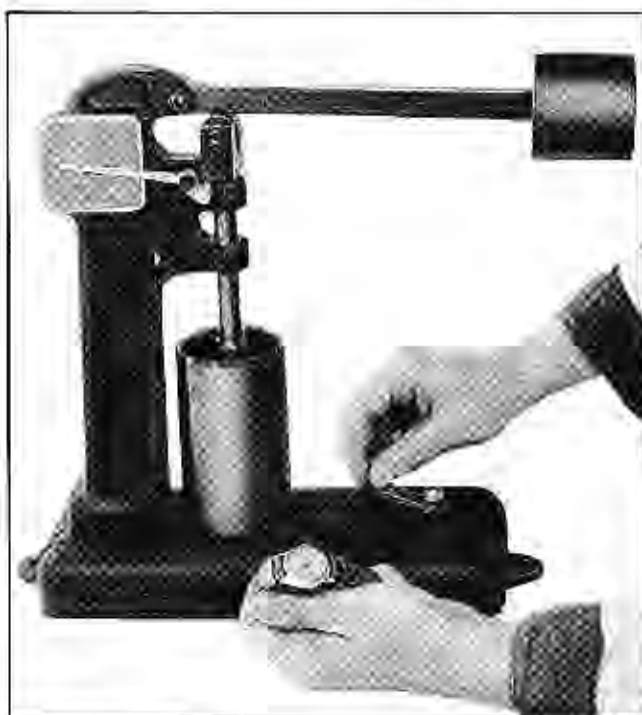
Fig. 6-28 Testing Leak-Down Rate
