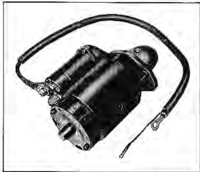
Fig. 11-52 Wires and Cables Connected to Solenoid
