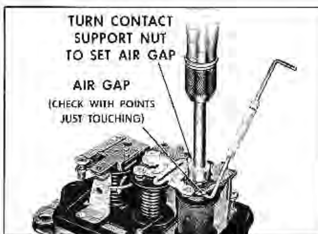
Fig. 11-39 Adjusting Voltage Regulator Air Gap—Single Contact Standard Regulator
