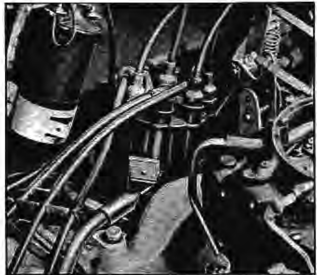
Fig. 11-56 Adjusting Dwell Angle
