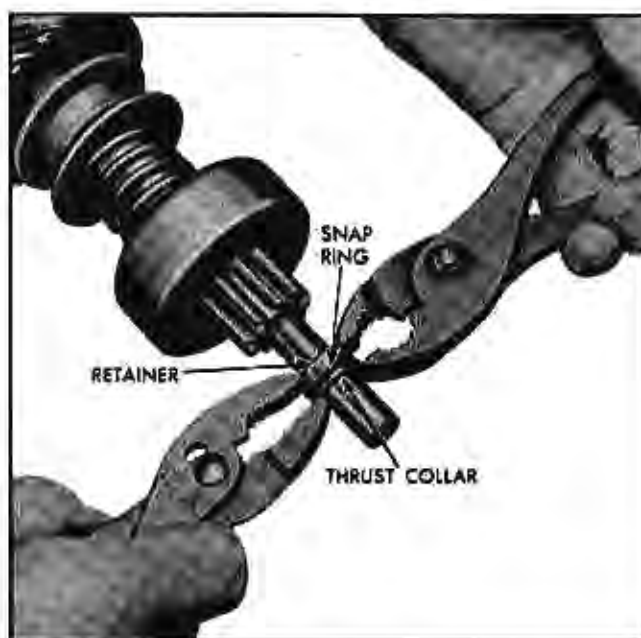
Fig. 11-50 Forcing Retainer Over Snap Ring
