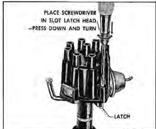
Fig. 11-58 Removing Distributor Cap
