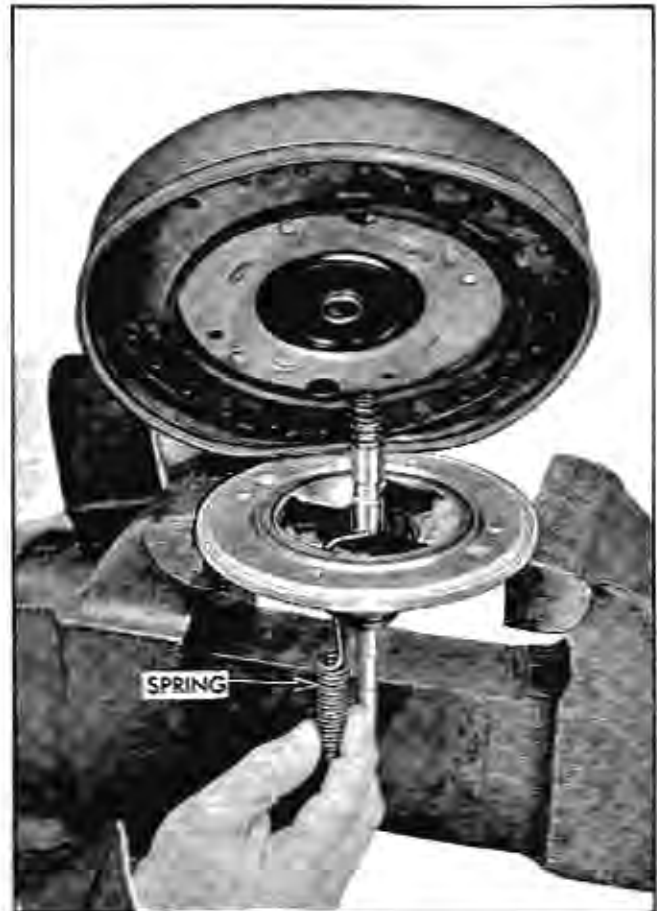
Fig. 5-M-19 Installing Rolling Diaphragm with Aid of Tool
