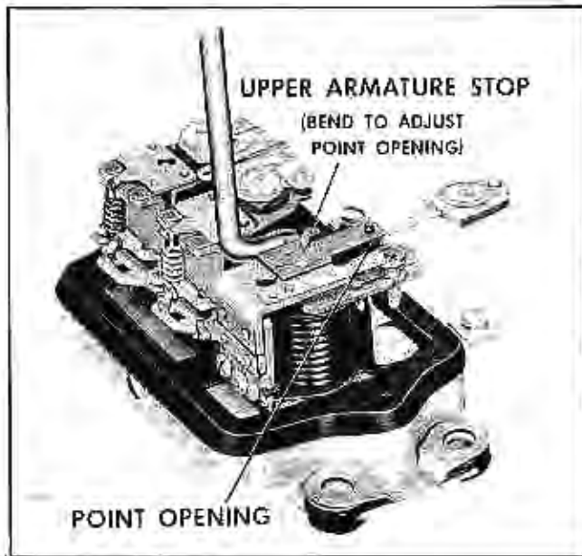
Fig. 11-38 Adjusting Cutout Relay Point Opening
