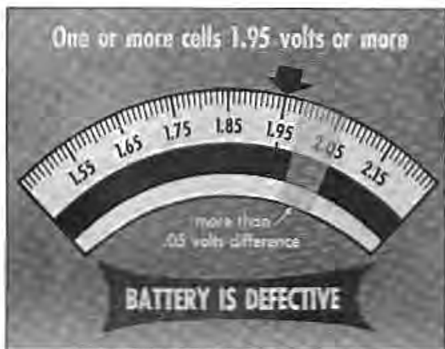
Fig. 11-7 Defective Battery—More than 0.05 Volts Difference
