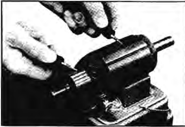
Fig. 11-14 Testing Armature for Ground
