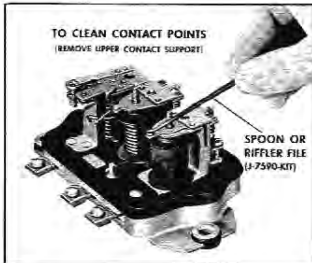
Fig. 11-35 Cleaning Regulator Contact Points
