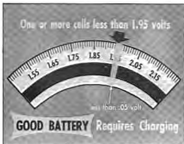
Fig. 11-6 Good Battery—Requires Charging
