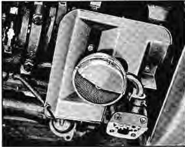
Fig. 6A-5 Oil Pump and Intake
