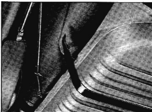
Fig. 8-1 Fuel Tank Retained at Front
