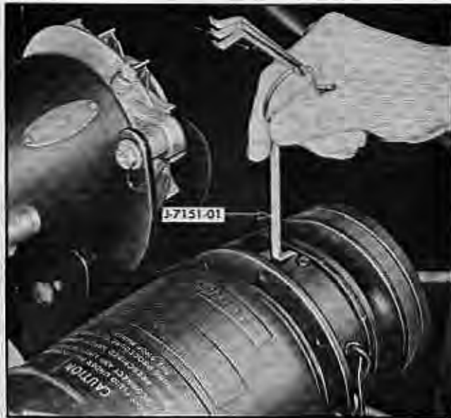
Fig. 6-60 Checking Air Gap
