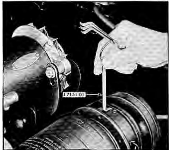
Fig. 6-67 Checking Air Gap
