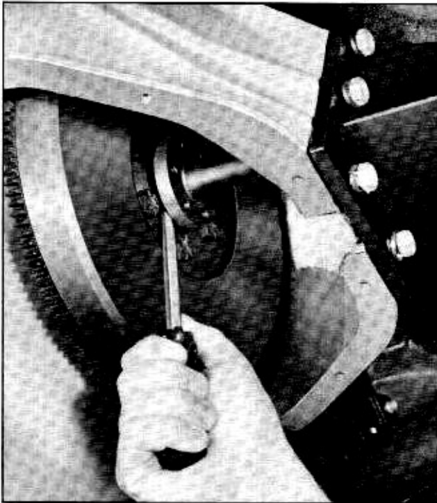
Fig. 4-17 Removing Propeller Shaft From Flywheel
