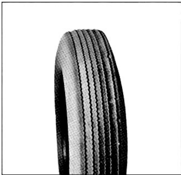
Fig. 3A-7 Toe-in or Toe-out Misalignment Wear
