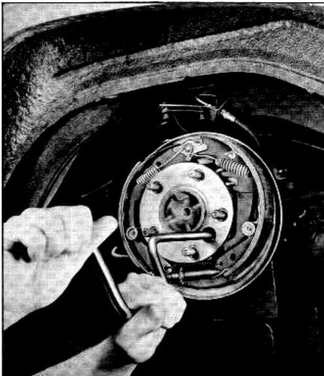
Fig. 4-4 Removing Nuts From Axle Shaft Bearing Retainer
