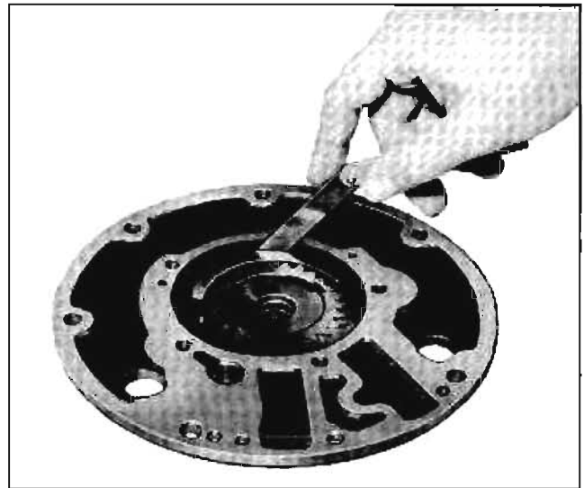
Fig. 7A-58 Checking Gear to Crescent Clearance
