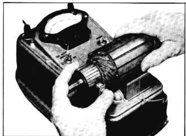
Fig. 11-9 Bar to Bar Test for Open Armature
