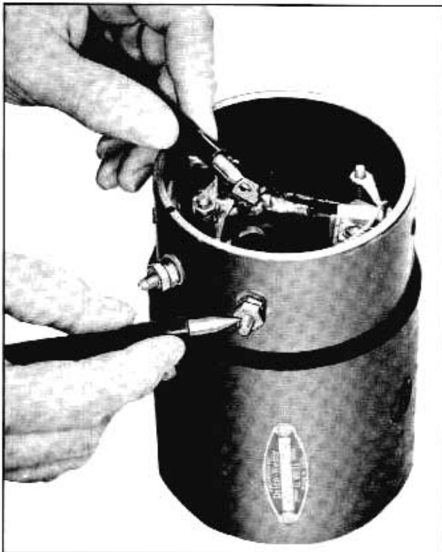
Fig. 11-11 Testing Field Coils for Open Circuit
