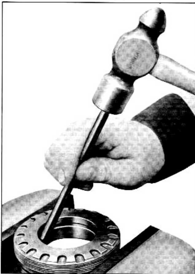
Fig. 4-49 Removing Front Pinion Bearing Outer Race (Automatic)
