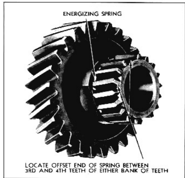
Fig. 7-37 Position of Energizing Spring
