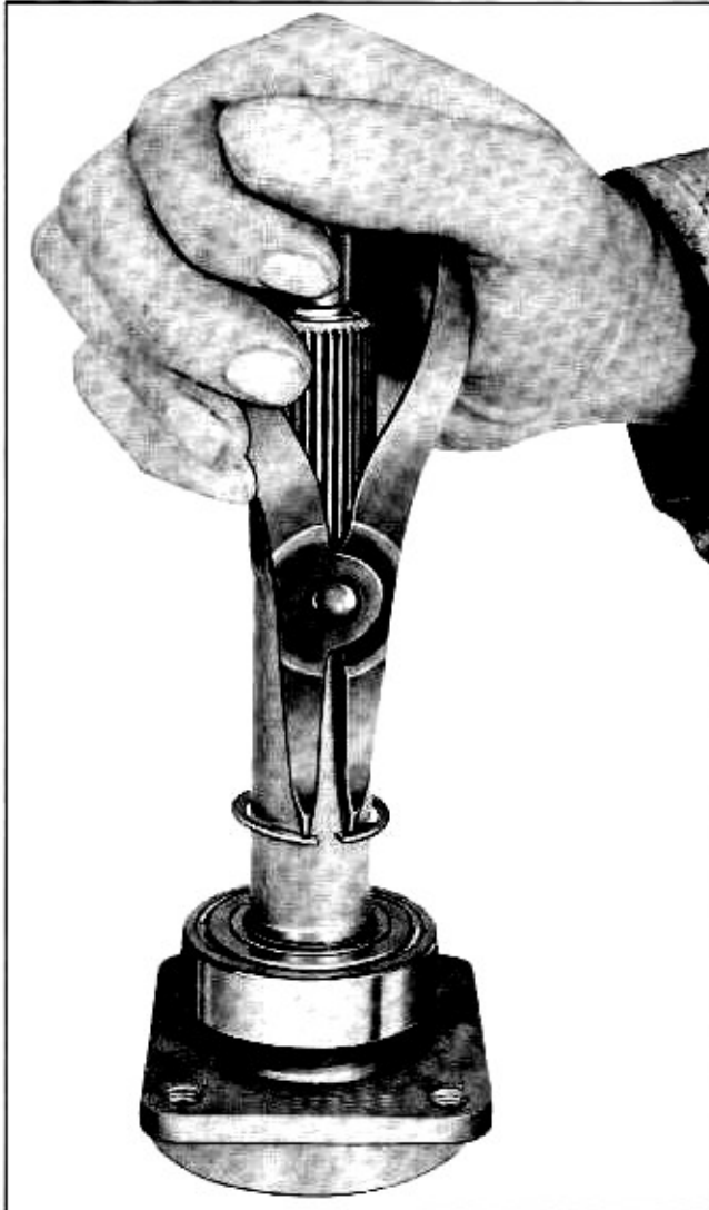
Fig. 6D-8 Removing Drive Shaft Bearing Retainer
