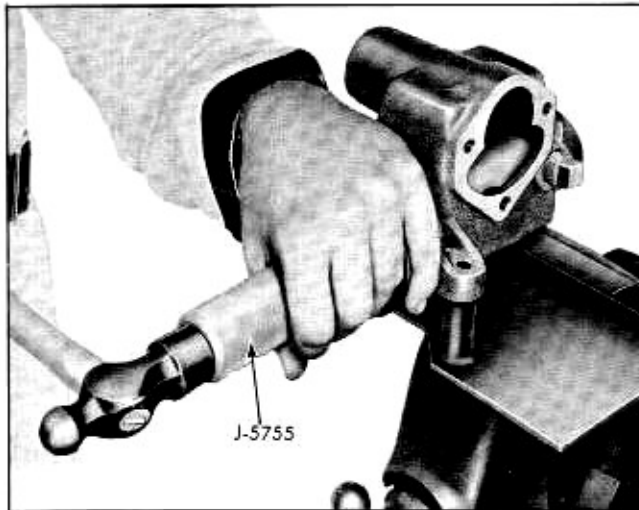
Fig. 9-27 Installing Upper Bearing Cup
