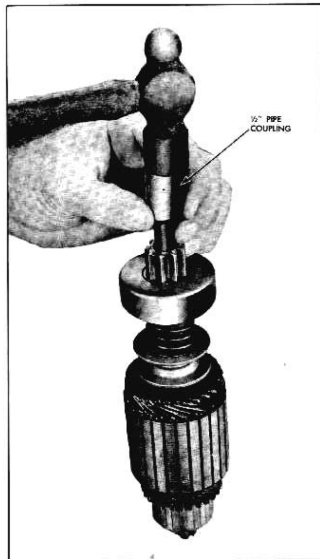
Fig. 11-33 Driving Retainer Off Snap Ring
