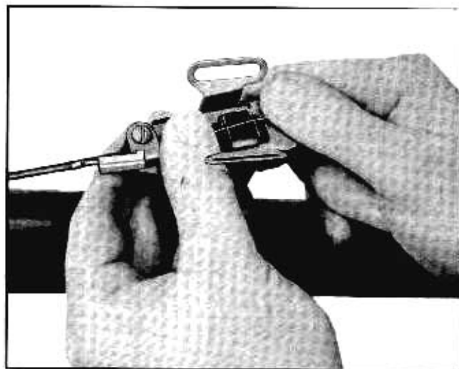
Fig. 11-89 Removing Control Cable from Switch
