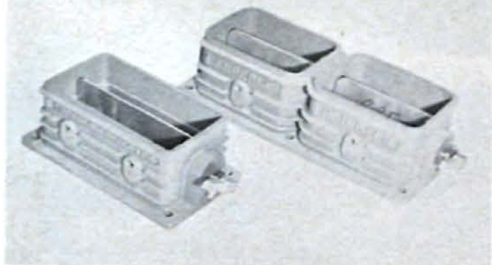
Enderle injector throttle body housings. Small one is for 4-71, other is for 6-71.
