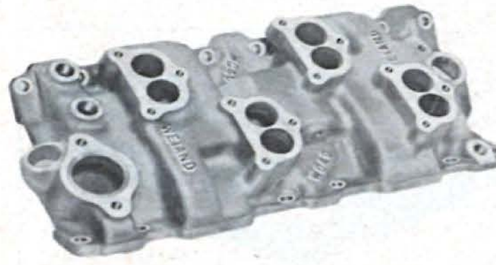
Weiand four-carburetor manifold is 180-degree type, uses two-throat carburetors.
