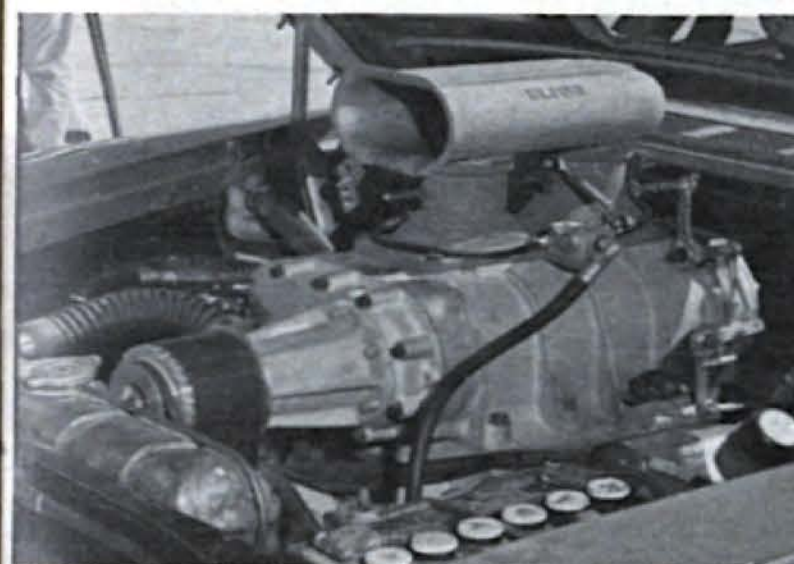
An injector makes a neat installation on a blower; also, it can pass plenty of air.
