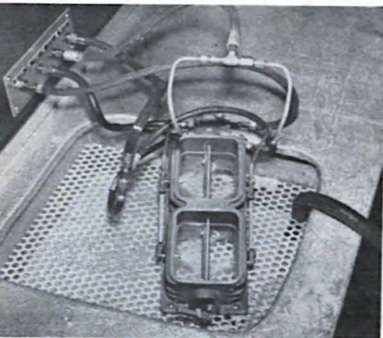
Enderle GMC blower fuel injector undergoing calibration tests on the flow bench.
