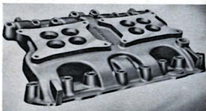
Offenhauser manifold for Dodge V8 is typical of dual four-throat manifolds.
