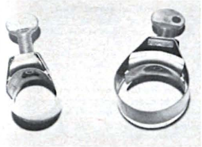
Above are screw-type clamps that can be used on fuel, air hoses instead of clamps of the spring type. At right are special fittings for connecting hoses to 97, 48 carbs.
