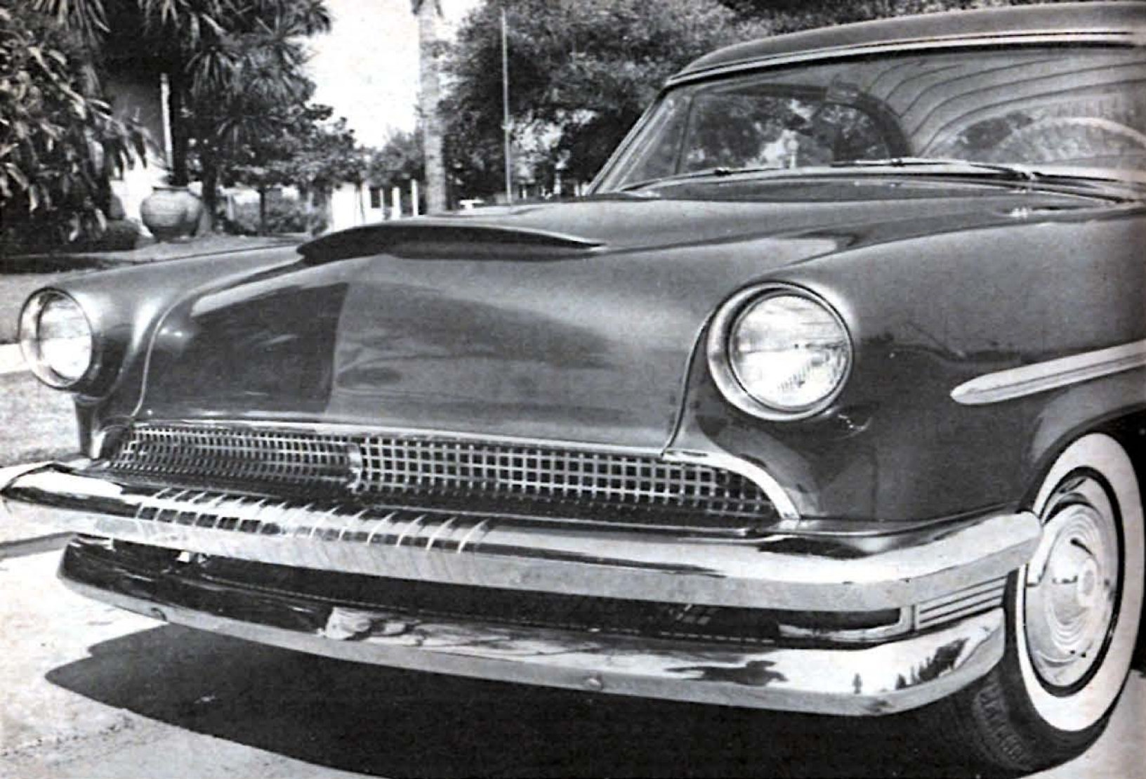
This 1954 Mercury has expanded square-mesh grille center installed between the upper bumper bar and the shell unit. The mesh hole size is \frac{5}{8} of an inch. Note how the customizer has shaped the grille center slightly into a concave curve. Fit is good.
