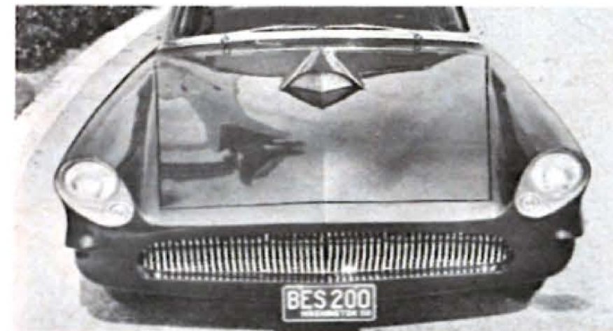
This 1953 Studebaker has sheet metal broken down from 18-gauge cold-roll and made into a large grille shell opening and frenched into the front fenders. The center section is from a Kaiser, recessed about six inches.
