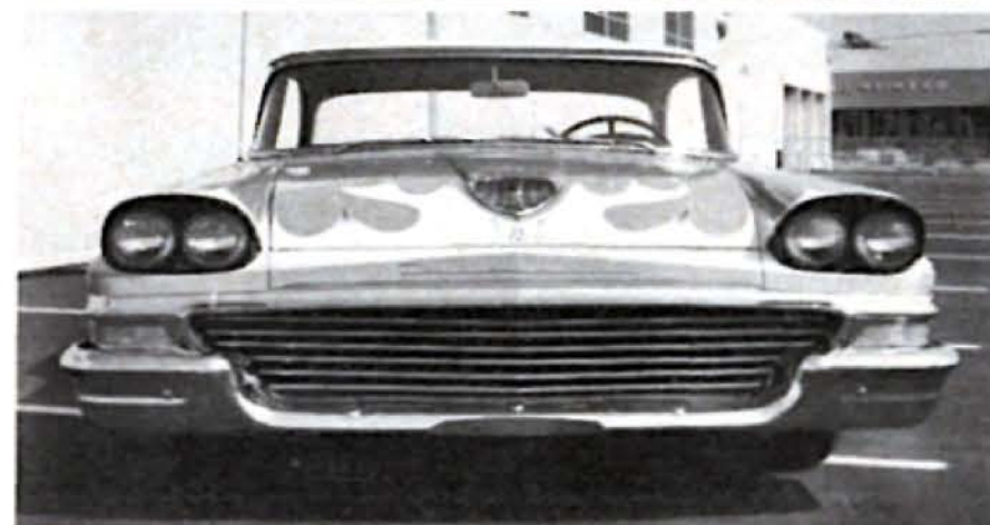
This 1958 Ford also features a stock custom grille kit consisting of horizontal tubes. No modifications of kit assembly was required for this installation.
