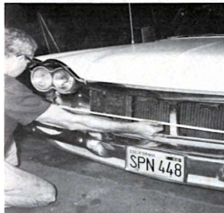
First step is to measure the grille shell opening after the removal of the stock or original grille center. This should be measured vertically as well as horizontally.
