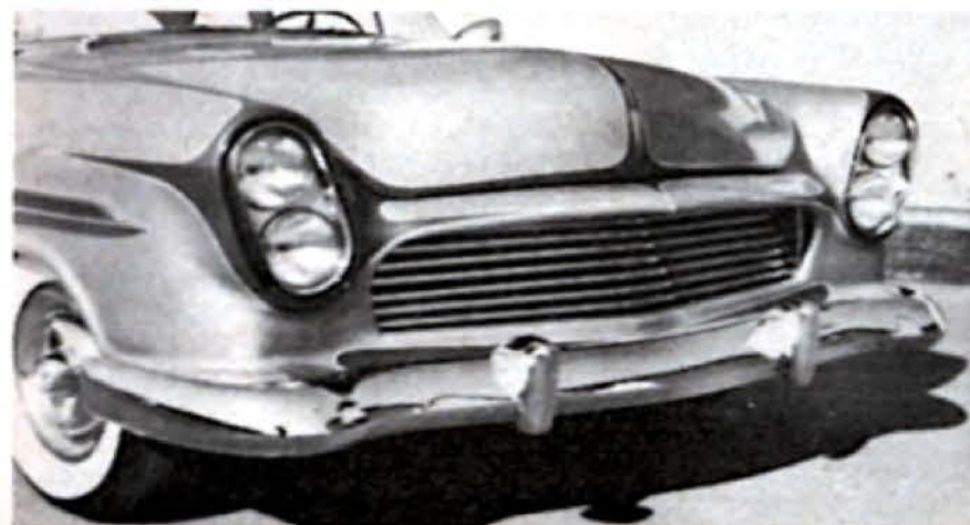
This 1954 Ford uses tubing, U-bends frenched onto the '53 grille shell. The metal has then been molded in completely with the front fenders and splash pan.
