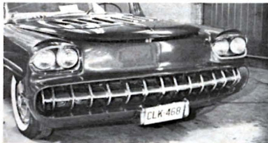
This unusual custom, a '56 Chevy, has four '54 Chevy grille centers with added blades. Note the rounded hood, unusually shaped headlight shells and airscoops in the fenders.
