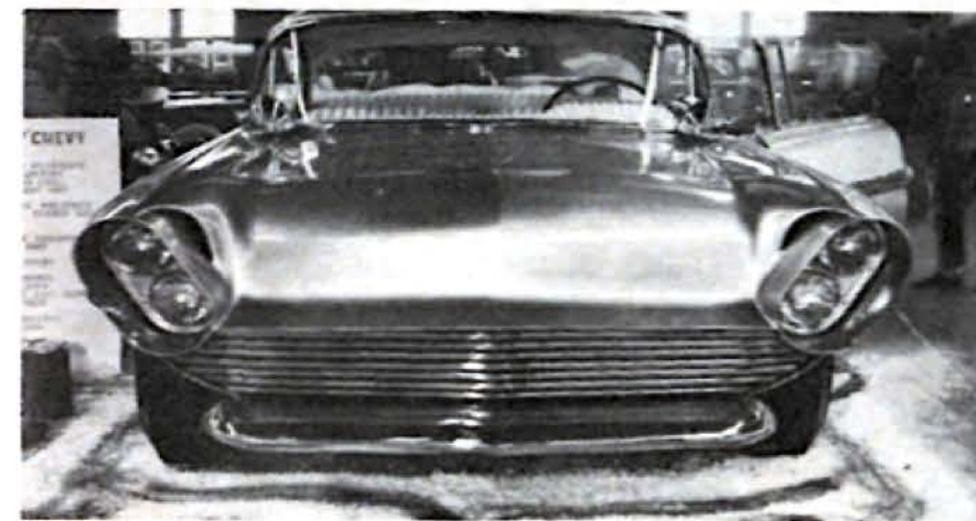
Here is a 1956 Chevrolet that has been nicely restyled with \frac{3}{4} -inch bar stock formed to fit an unusually shaped grille cavity. Note the scoop-type, narrowed bumper.
