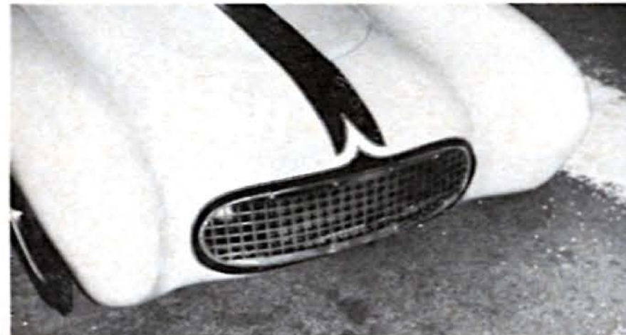
A waffle, checked-mesh-type design is quite popular with the sports car set. This expanded metal grille was taken from a Thunderbird, cut down, and inserted in this sports car special. Note outer chrome rim to which mesh is bolted.
