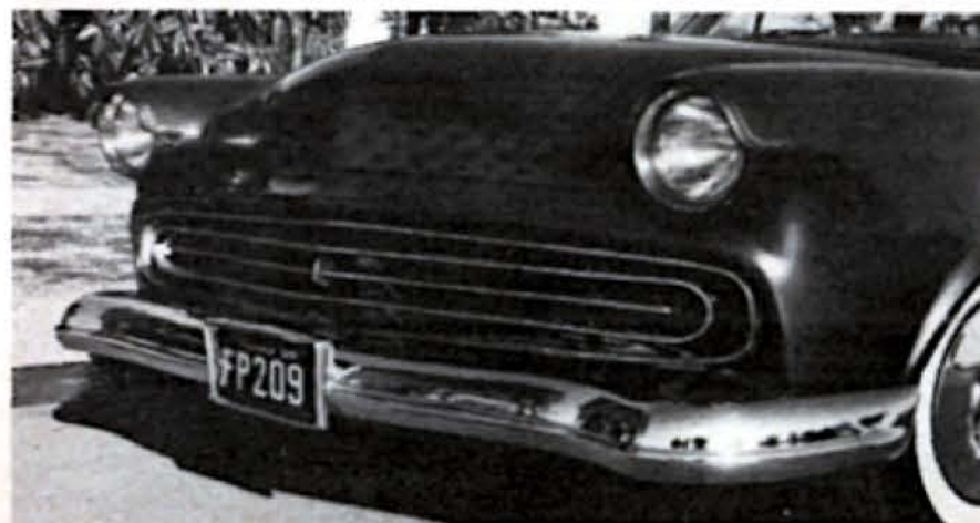
You can also modernize the older cars. This '53 Ford has good-looking front-end styling which features \frac{1}{4} -inch by 2-inch hot-rolled strap metal, contoured around the grille cavity.
