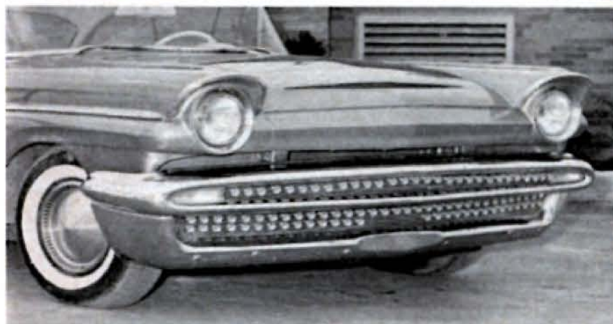
A complete bumper assembly from a 1957 DeSoto is installed in the front end of this 1957 Ford. Perforated mesh is used for backing and drawer pulls are installed.
