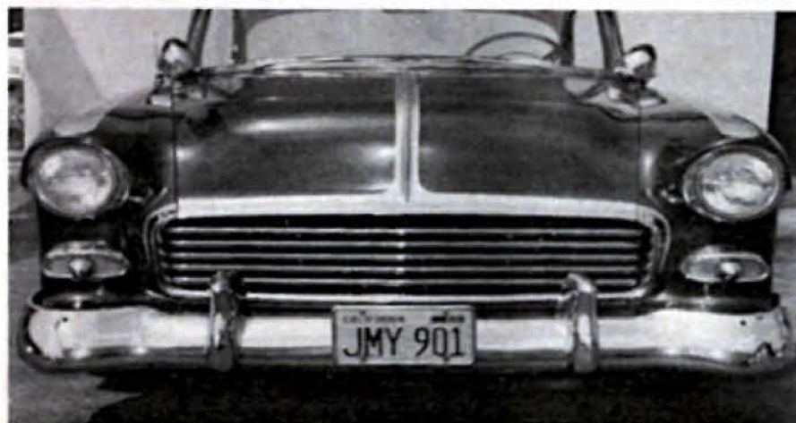
This is a half-tube grille inserted in a 1956 Chevrolet. It is available from California Custom Accessories or your local automotive accessory store for $19.95.
