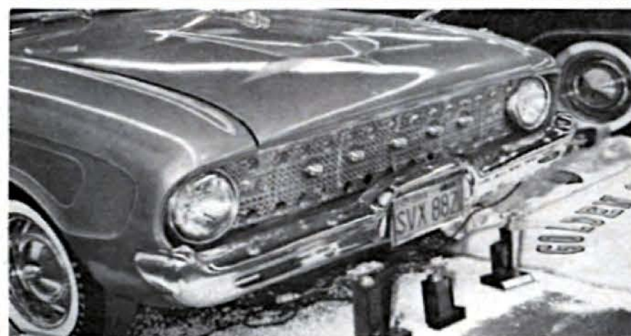
An aluminum mesh fills grille cavity of this 1960 Falcon. The mesh, costing $1.49 a sheet, has a clover leaf design. Small wheel bullets are installed in a row along the center and two rows of drawer pulls and a pair of directional lights complete the unusual installation.
