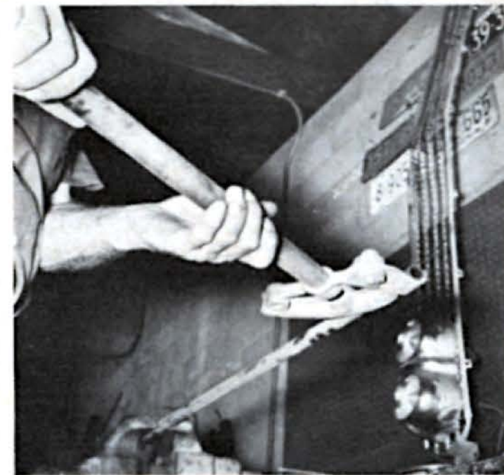
With the tube or bar stock placed securely in a vise, bend the material to the desired shape. In the case of tubular raw stock, a tube bender may be used, as shown, to obtain any number of curves in the material, depending on the design.
