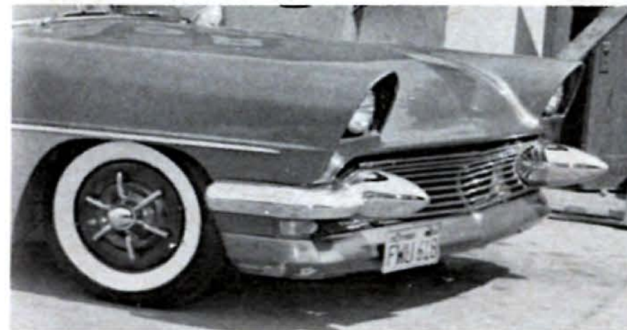
This '55 Mercury uses '55 Buick bumper bullets welded onto Mercury stock bumper end sections. Round rod, concaved and mounted horizontally, form the center grille.
