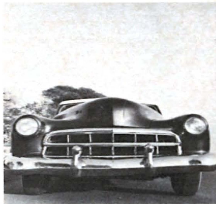
Here's an 18-year-old car, a '42 Buick which has been customized nicely by inserting a '49 Cadillac grille center section with the end sections cut and molded into the two front fenders and aligned with the hood. Note the frenched lights.
