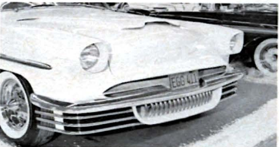
This 1954 Mercury has a reformed front bumper attached to front end. Tubes run horizontally and wrap-around. Note vertical tubes in center lower section.
