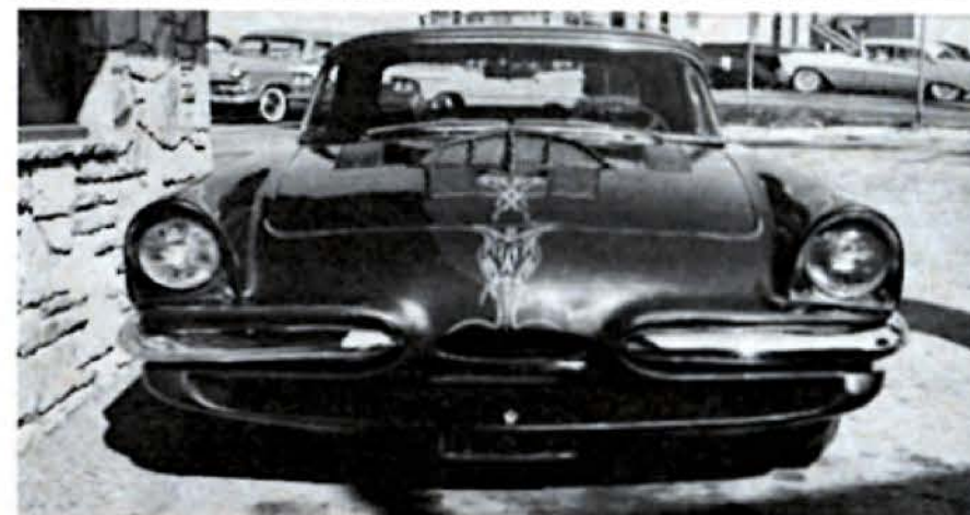
This 1955 Thunderbird has '55 Pontiac bumpers inset in the '55 Pontiac shell openings. A Studebaker lower pan is used. All metalwork has been molded in to provide one-piece look.
