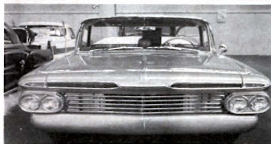
This is a full-tube grille in a 1959 Chevrolet, showing how a purchased custom grille can be used with a rolled grille pan.
