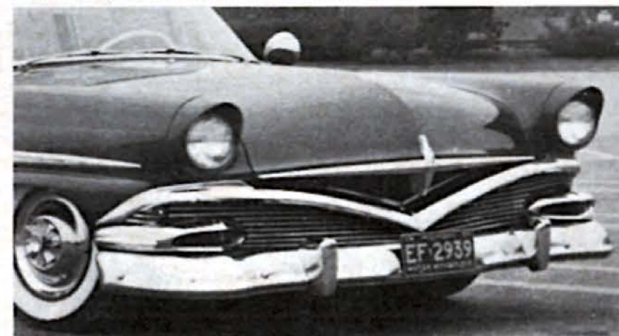
Creating a radical appearance, this '56 Ford has a '56 Ford Canadian Meteor grille fitted into the cavity with an upper grille ornament mounted on the hood.
