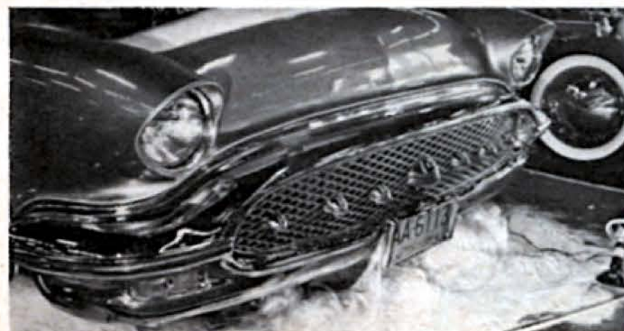
This 1956 Oldsmobile with its standard bumper-grille assembly makes for a natural setup for styling changes, if desired. The owner has inserted gate-type expanded metal in the grille cavity onto which he has installed two sizes of chrome bullets horizontally.
