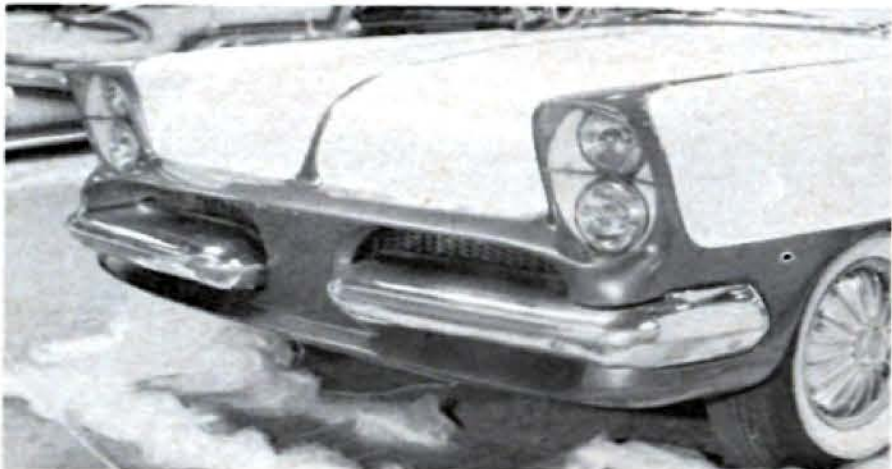
Here's a 1957 Chevrolet which features a front end with '58 Dodge front bumpers installed into a grille shell formed from a '53 Studebaker pan. Note split grille opening.
