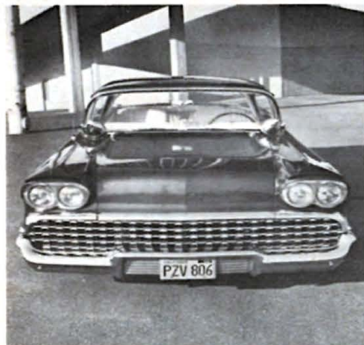
On this '58 Chevrolet, the grille cavity has been filled with a '59 Buick center section. The front-end of this particular custom has also been enhanced by special molded air scoops above the dual headlights. The scoops are non-functional.
