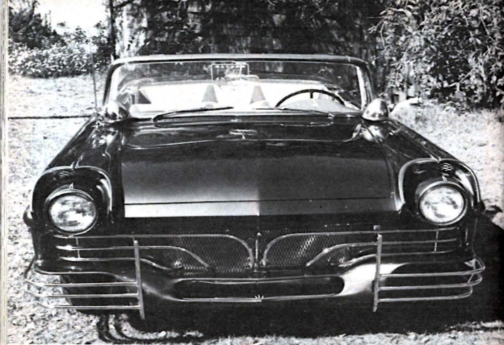
This handmade grille is from the radical school of design, an excellent example of how far out one can go in making up from raw stock a completely different grille. The car is a 1957 Ford convertible. Note how the grille cavity has been reshaped.
