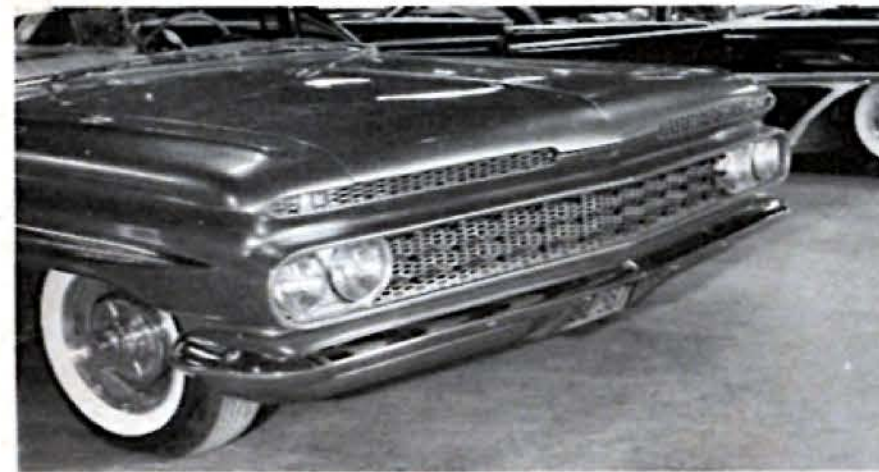
'59 Chevrolet features a \frac{3}{8} " by 1" oblong hole, 18-gauge, cold-roll expanded metal grille. Note the triple roll of pronged metal tubes extending out from grille.
