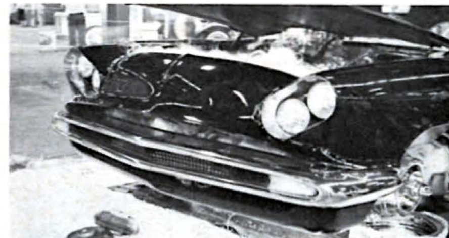
Here's a 1956 Oldsmobile which has the popular '57 DeSoto bumper unit. In its center expanded metal is used. A late-model pan is used on bottom side of the bumper.
