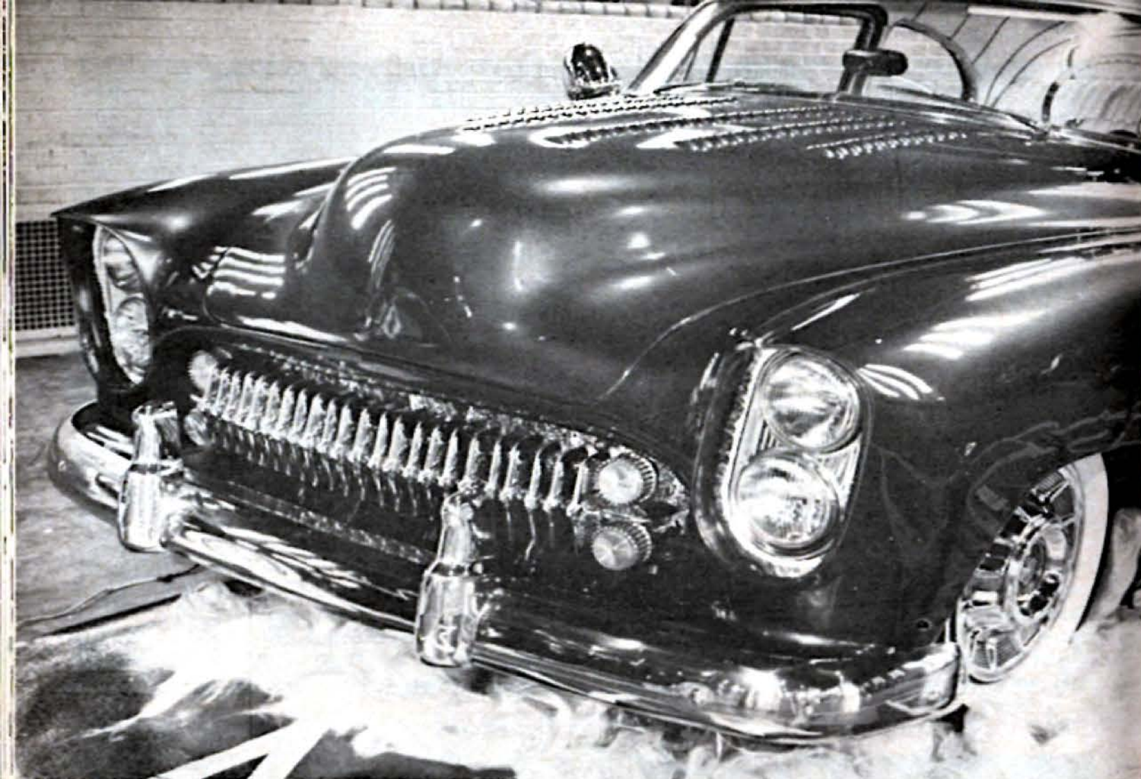
This 1950 Chevrolet has a '50 Mercury grille shell frenched into the fenders. The center floating grille bar is a '57 Corvette with three times as many vertical teeth added than on the original design. Four directional lights, taken from '59 Cadillac taillights, have been installed at either end. The white reflectors are used only, not the red.
