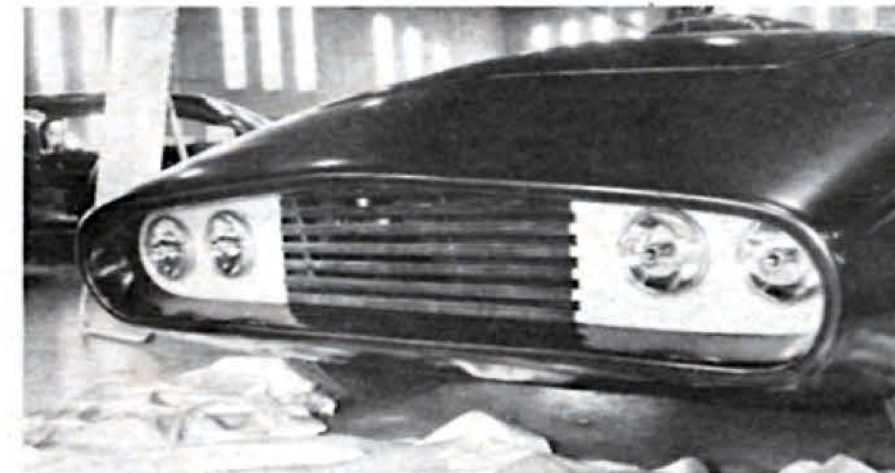
Plastic frosted sheets have been used around the twin headlights within a newly designed grille cavity in this unusual Thunderbird. Note the 3/4-inch round plastic grille bars in the center.
