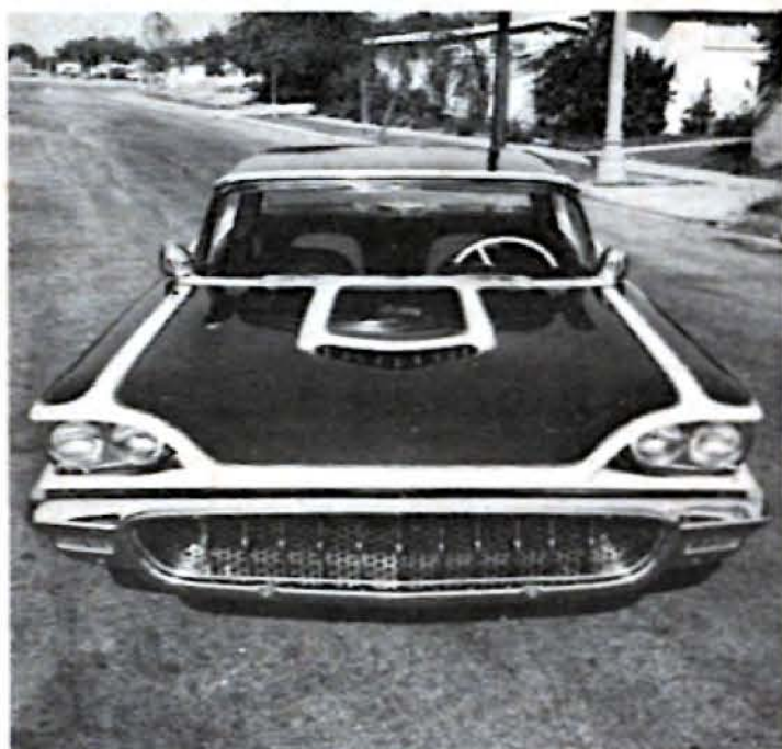
This '58 Thunderbird is not only distinctive because of the redesigned grille but also because of the unusual painting. The grille has vertical uprights taken from a '57 Corvette attached to the original Thunderbird mesh-type grille.
