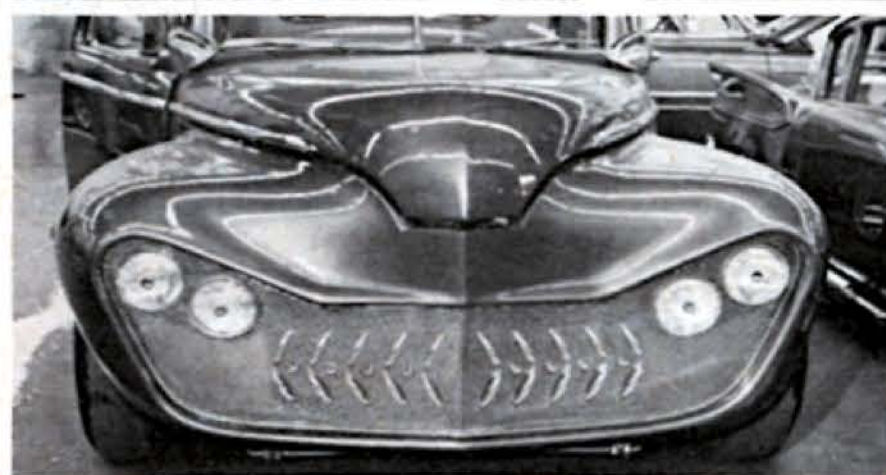
This 1948 Plymouth has an unusually shaped grille cavity in which 1/4-inch expanded metal has been installed. Gold-plated drawer pulls are used in a V design with smaller round drawer pulls inserted between the longer pulls.
