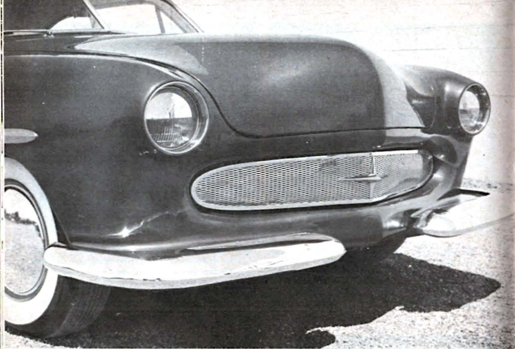
This 1949 Ford has been nicely customized by using a '50 Mercury grille shell which has been neatly frenched into a pleasing oval shape. The expanded metal center section is called offset type, \frac{1}{4} -inch by \frac{3}{4} -inch openings. A \frac{1}{2} -inch metal band has been welded onto the expanded metal. The complete unit is chromed and floated in shell.
