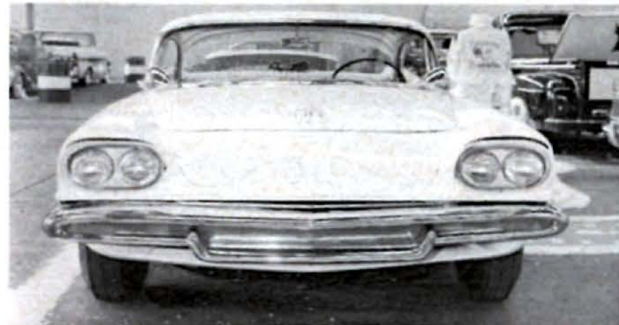
This 1956 Chevrolet has a '57 Dodge front bumper. Note pancaked hood. Lower section has small Studebaker pan.
