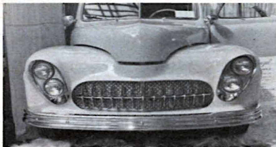
Here's an old one, a '46 Ford that's been customized rather radically. It has a frenched grille shell with aluminum expanded metal backing with a '56 Corvette grille installed in front, a nice design.
