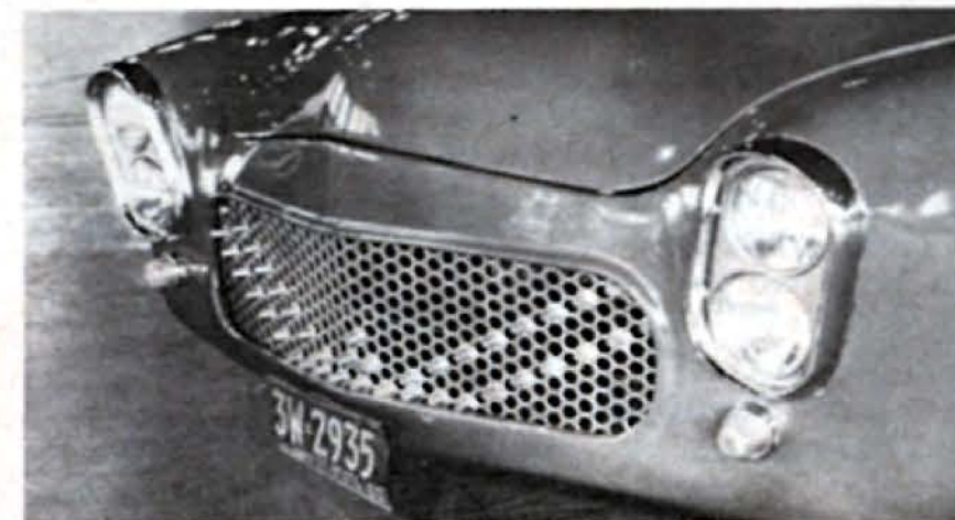
Here's a case of a rather old car, a '49 Ford, being modernized completely by a new front-end treatment. The grille center section is from a '58 T-Bird with small bullets from a '58 Cadillac and installed on mesh.
