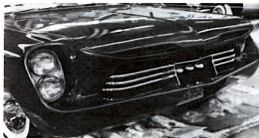
This is a 1959 Chevrolet, radically restyled on the front end with multi-contoured shapes. The frenched grille shell cavity features \frac{1}{4} -inch center plate made into a box in which three bullets sit horizontally.
