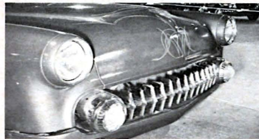
This '52 Mercury has been modified nicely by the use of '55 Ford parking lights and '56 Corvette grille center to which additional vertical blades have been installed.
