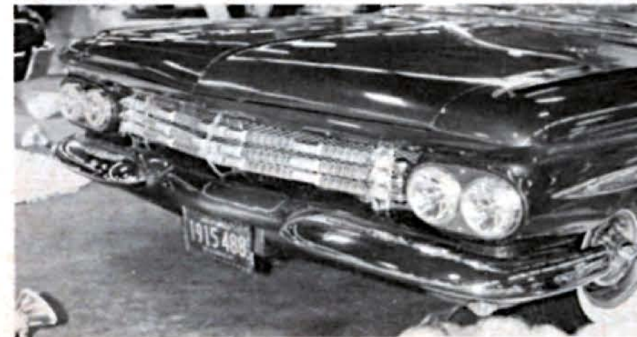
This 1959 Chevrolet features horizontal plastic tubes that have a rainbow of colors laminated onto each. This unusual grille represents a lot of work by the owner.
