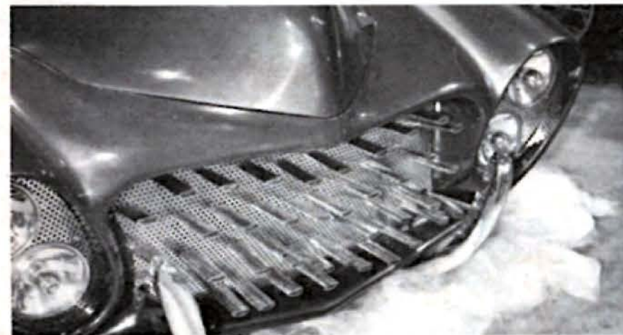
The expanded metal here is 20-gauge cold roll with \frac{1}{4} -inch holes. The car is a '40 Ford. The flattened tubular prongs add interest to the unusual grille design that has been created. Note headlights.
