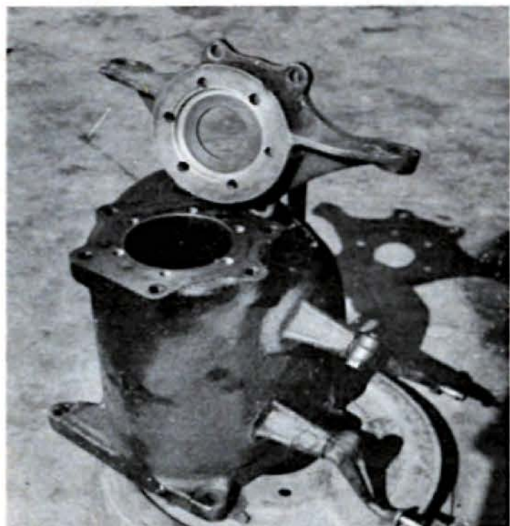
Holes have been drilled and threaded in the rear flange of this Cad trans case for a Ford torque tube connector flange.
