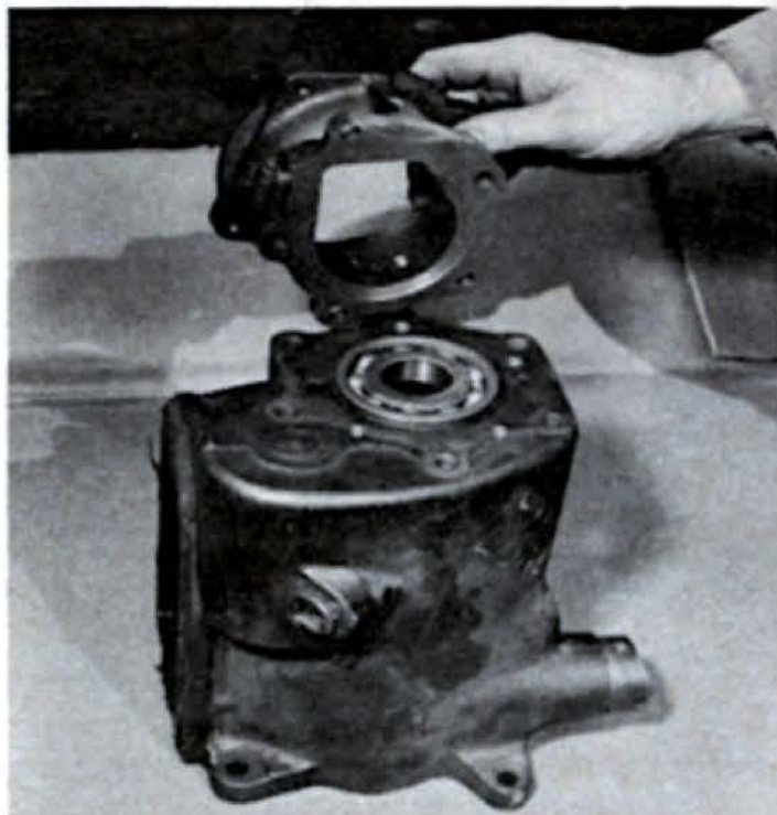
The rear flange in this Cad transmission case has been drilled to enable a Chevy torque tube connector to be bolted to it.
