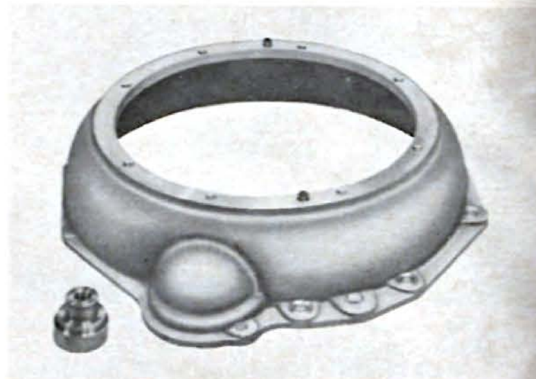
This adaptor is one of many for '32-'48 Ford and similar transmissions and a long list of engines used for swaps.
