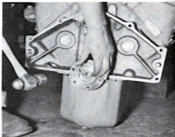
This ring adapts a Ford pilot bearing to a Chevy crankshaft. A pilot bearing must be installed to support the clutch shaft.
