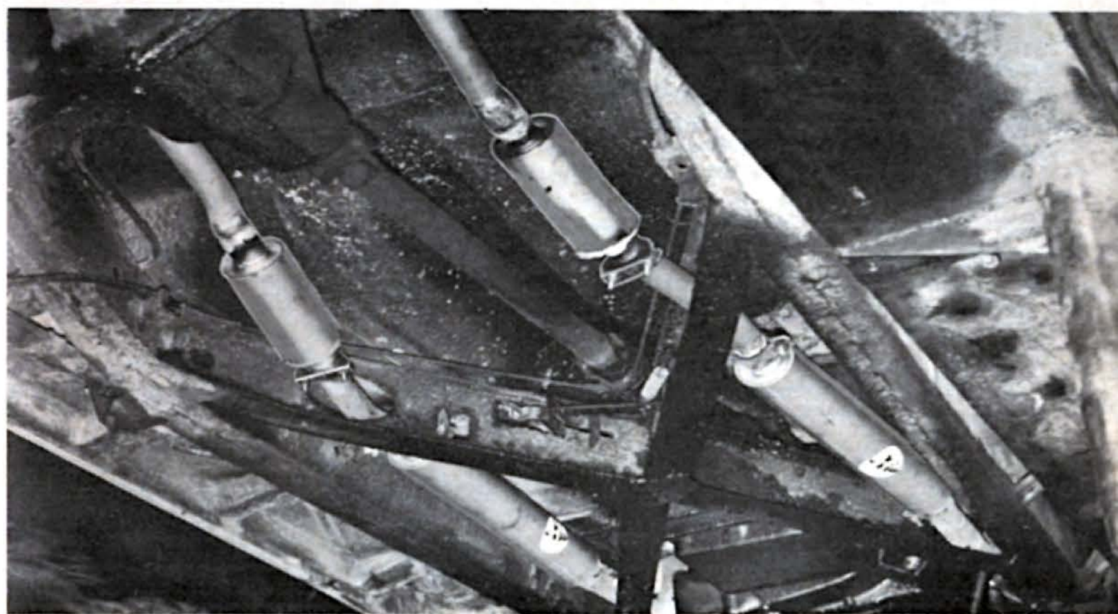
The dual exhaust system on this car has four glass-packed mufflers instead of the usual two to guarantee that it will be quiet under all conditions. Noisy exhaust system does not make sense if the car is to be driven in town because of the trouble it can cause.
