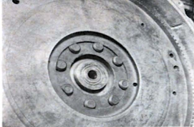
The adaptor in a Chrysler Windsor crankshaft flange holds the pilot bearing for a Cad-LaSalle concentric with the shaft.
