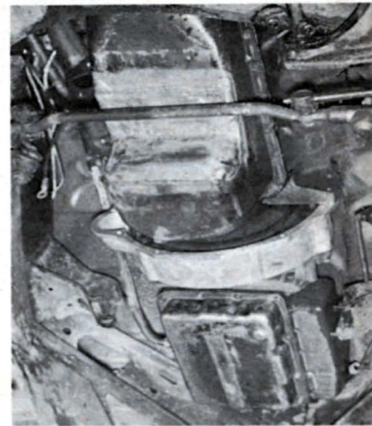
Clearance for a '56 Chevy's steering linkage was gained by shortening the sump on the pan of Cad engine installed in it.
