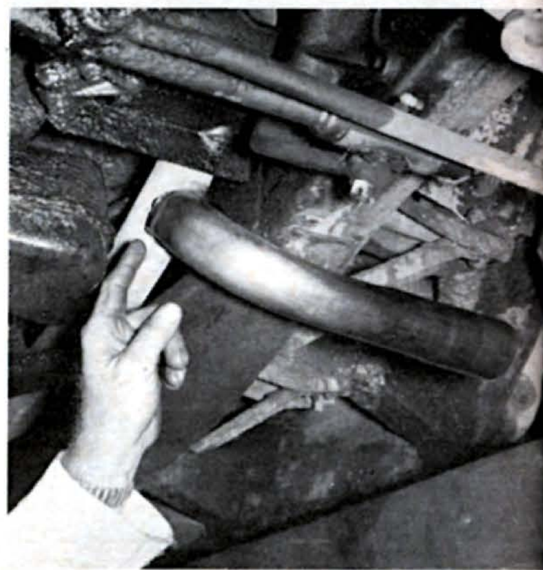
Lakes pipes are welded to the stock headpipes over an opening of the correct diameter. The flow of exhaust gases through them is controlled with caps on their ends.
