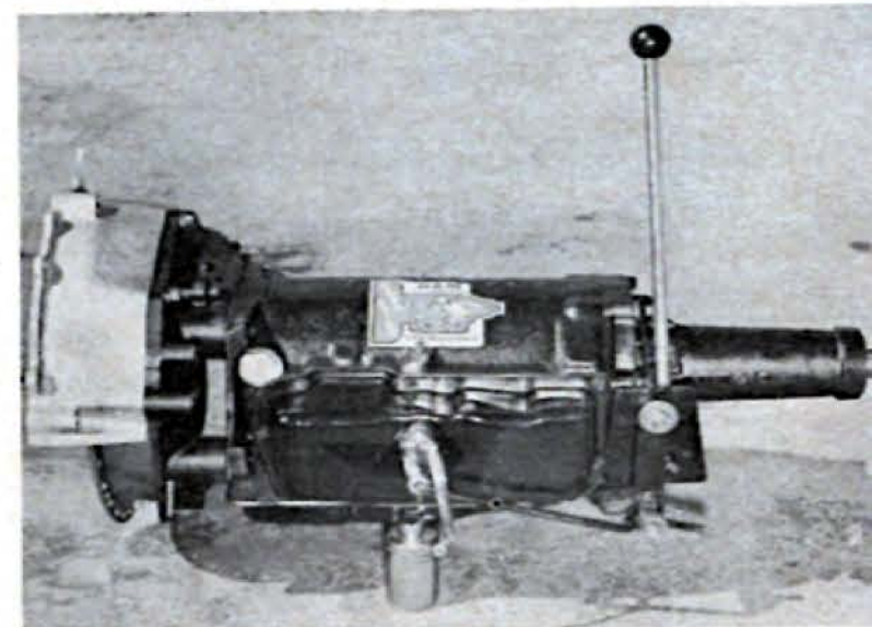
One of the best things to ever happen for hot rodders is the B&M Hydro-Stick transmission. This is a reworked Hydra-matic that takes the guesswork out of shifting.
