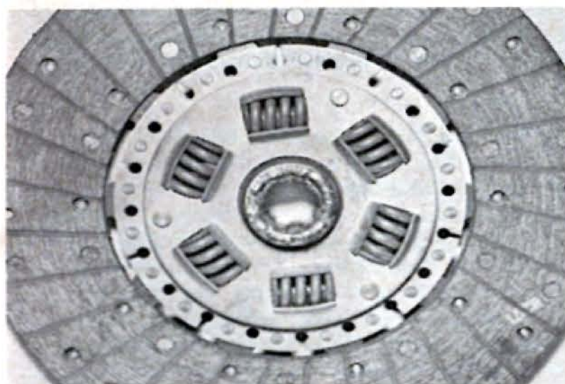
This clutch disc was adapted to a transmission of a different make by welding a spline from another disc inside its hub.
