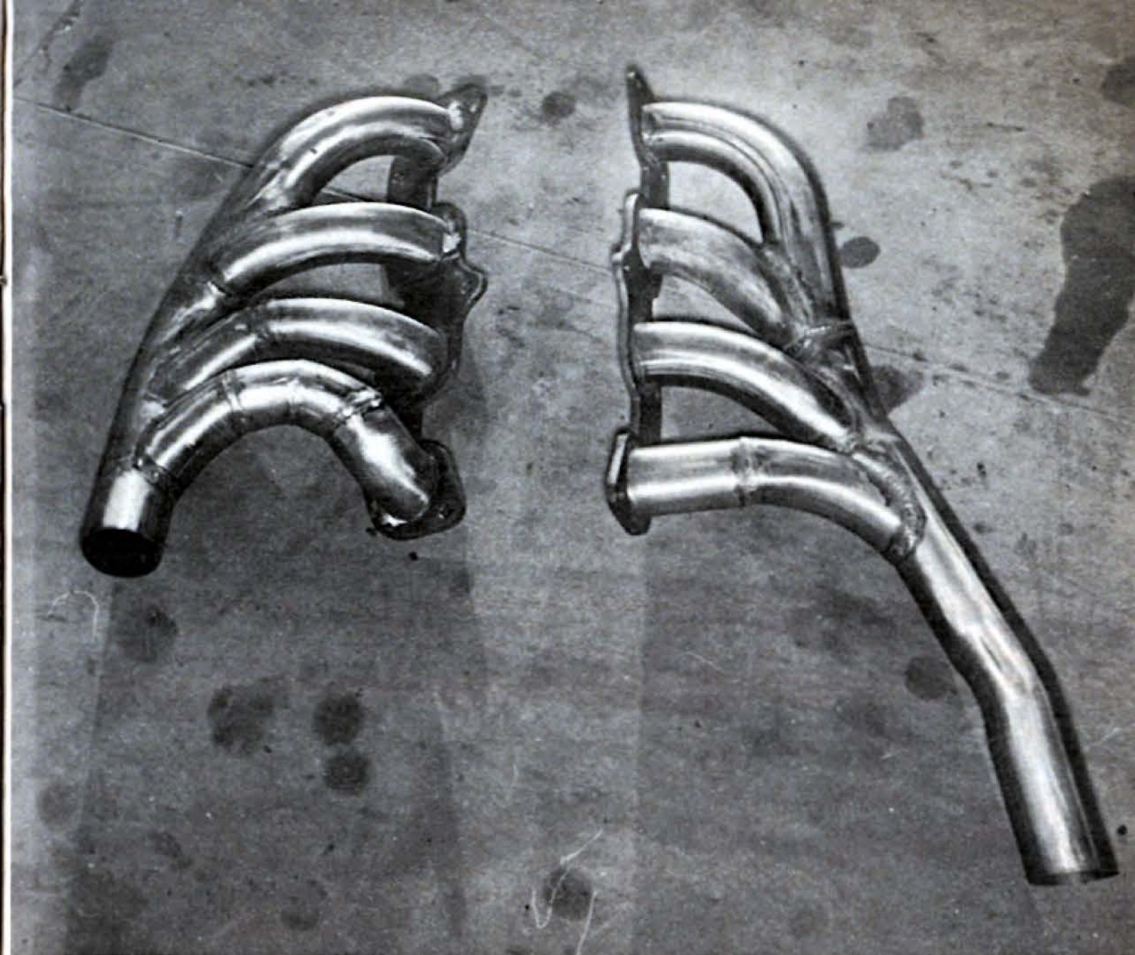
These headers were made for a 300-D Chrysler engine, installed in a '56 Mercury. Headers are often necessary for engine swaps because chassis members won't let an engine be installed with its stock exhaust manifolds. Headers aren't easy to build.
