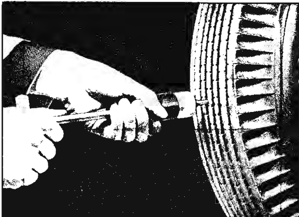
Fig. 36—Filling Hole with Sealing Gun
