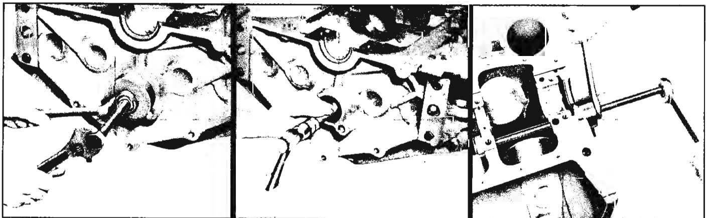
Fig. 149—Removing No. 4 Camshaft Bearing
