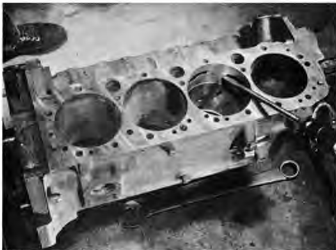
Use a screwdriver to remove the remaining sections. The cylinder walls' remarkable consistency of thickness is a tribute to Chevrolet's casting practice.
