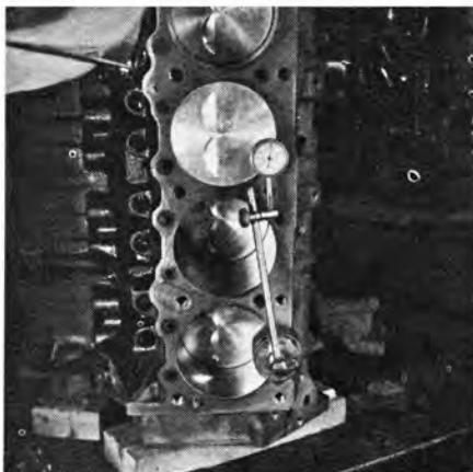
Piston-to-top deck clearance must be checked with dial indicator. It forms part of combustion chamber volume and must be included in when cleaning, checking, combustion chamber volumes.
