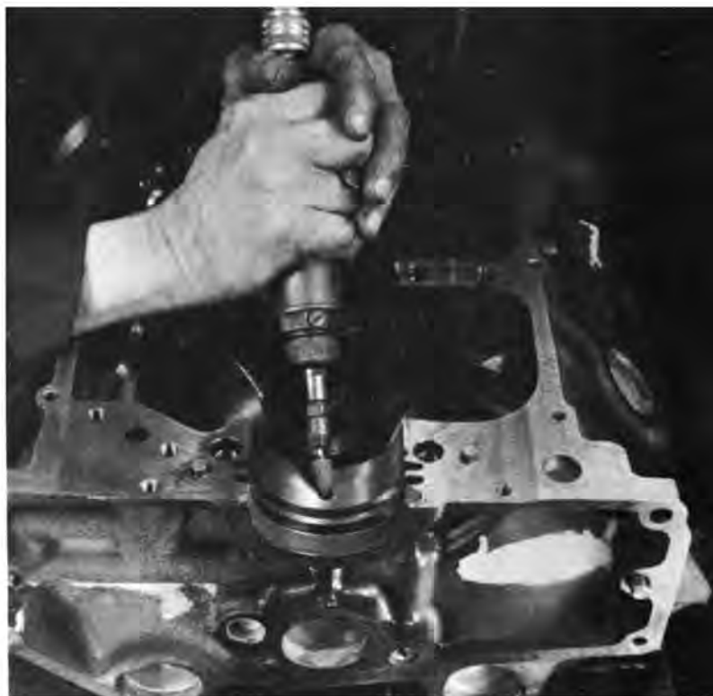
Chamfer oil passage edge in block. Remove only marked section. All-around chamfer exposes bearing underside.
