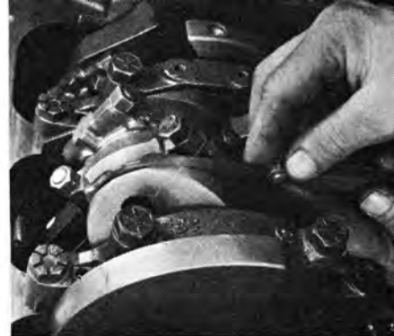
Check rod side clearance with feeler gauge. Opening clearance a bit improves oil flow through bearings.
