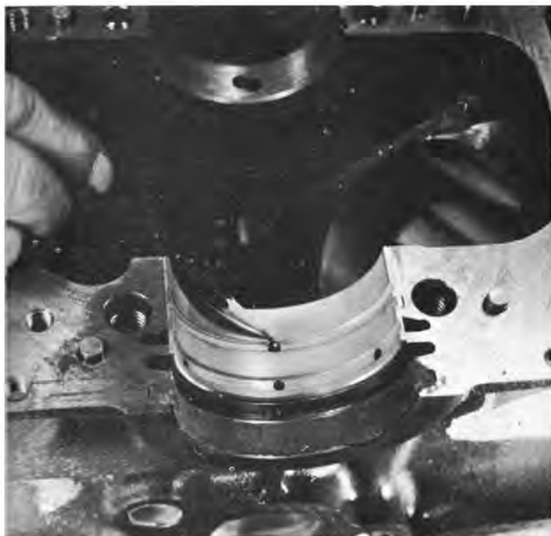
Misalignment between oil holes in main bearing and block must be corrected so oil supply won't be partly strangled.
