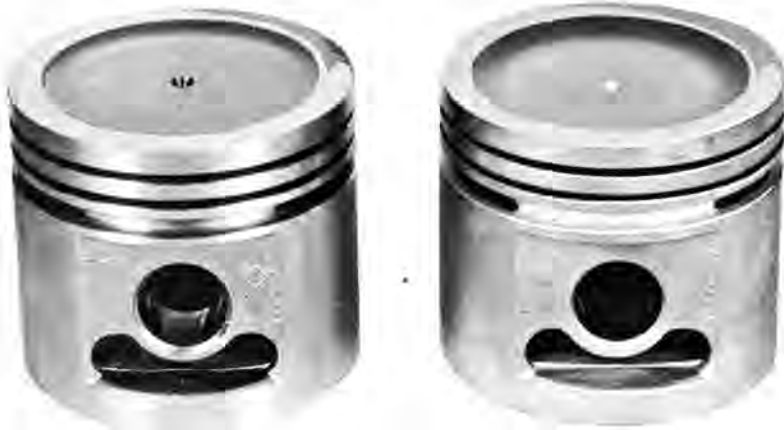
Pistons have dished tops, are all-aluminum. Switch to flat top pistons ups compression from 8.8 or 10.25 to 11-to-1. Full skirt at bottom offers better resistance to piston slap. Cast iron main bearings (above) control both expansion at mains and cut down clearance changes. Block's inside and water jackets are sand core-cast while its exterior is permanent mold-cast. Note that there is ample room for a stroker shaft here.
