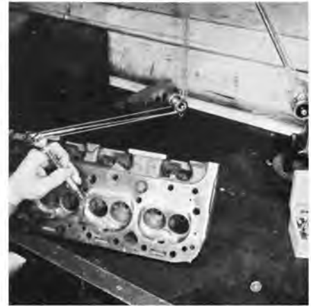
High speed toolmaker's grinder (also used by your favorite dentist) helps unpocket valves, round out corners.
