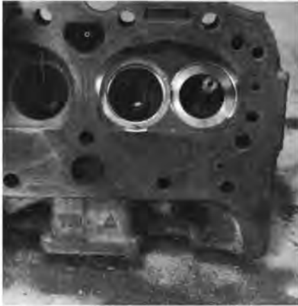
Next valve seat's ready for installation. All excess metal in bowl is removed with hand grinder.
