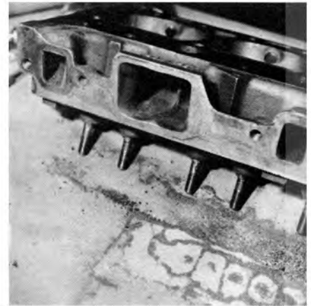
Carve ports for maximum breathing at high rpm. Port dividers are almost completely removed for peak hp.
