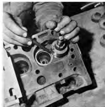
Place seats, valves closely so cut for next seat overlaps first. This draws maximum power from engine.
