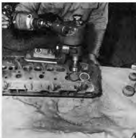
Cutter piloted on same shaft now cuts deep groove for inserting valve seats. They'll be faced-off with head.
