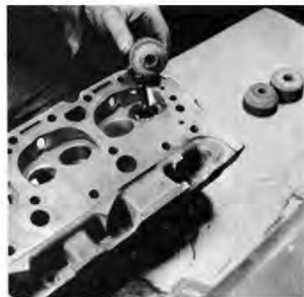
Place seats, valves closely so cut for next seat overlaps first. This draws maximum power from engine.
