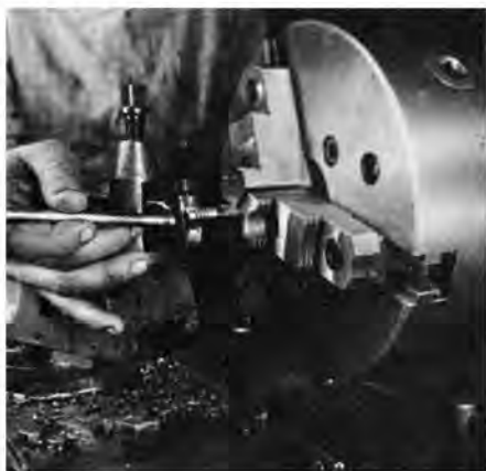
Cutter piloted on same shaft now cuts deep groove for inserting valve seats. They'll be faced-off with head.
