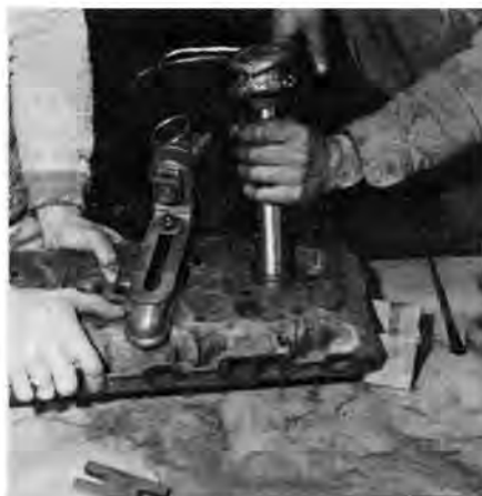
Install seat into newly cut groove with driver. Minimum interference fit will avoid distortion.
