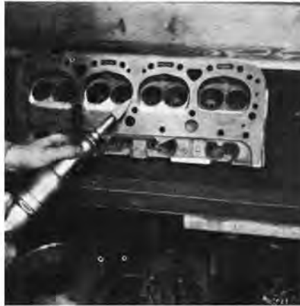
Use blueing on head for reference lines. Remove sharp edge across squish area for smooth gas flow.
