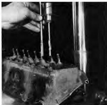
Install seat into newly cut groove with driver. Minimum interference fit will avoid distortion.
