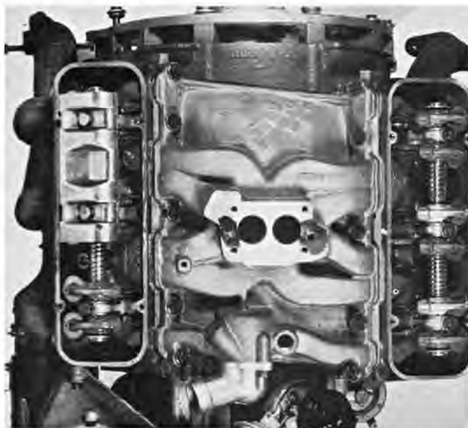
The spark plugs have been angled to clear the exhaust ports, and the rockers are aluminum die castings with steel inserts at the push rod and valve ends. Most valve train parts are interchangeable with the V8's.
