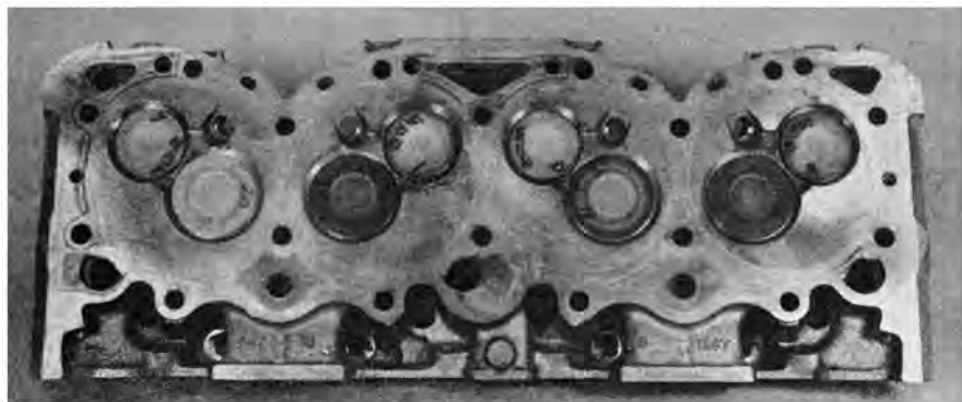
409's cylinder head has same number of valves as 348's, certainly ample. Larger bores, redesigned pistons, have unpocketed valves.
