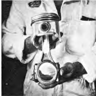
Groove in pistons, above rings, serves as heat dam; prevents heat from reaching top ring.
