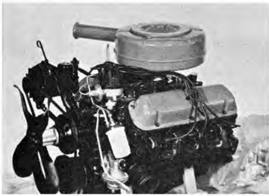
Exhaust manifold is cast iron version of header. Note how angled plugs clear the ports.
