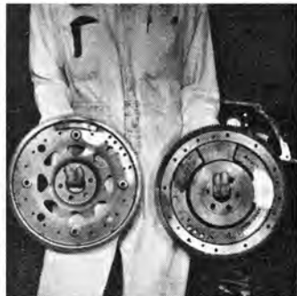
At left is automatic's flywheel with counterweight at periphery. Clutch's flywheel is right.
