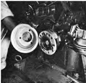
External counterweighting supplements counterweights of crank, itself. One is next to the pulley.
