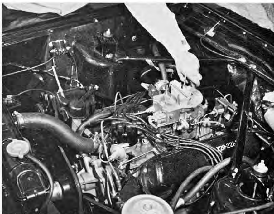
Engine has been designed to fit between spring towers of a unit-bodied car. With cast iron block, it weighs just 459 pound with starter, clutch.
