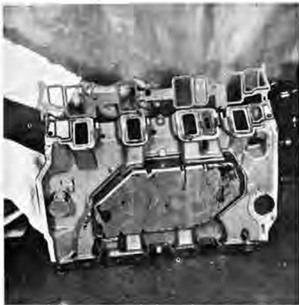
Special intake manifold gasket is available for blocking-off heat riser passage. This has effect of allowing a small gain in total horsepower.
