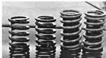
Stiffer valve springs with flat wound dampen return big valves help return big valves of 405 hp option.
