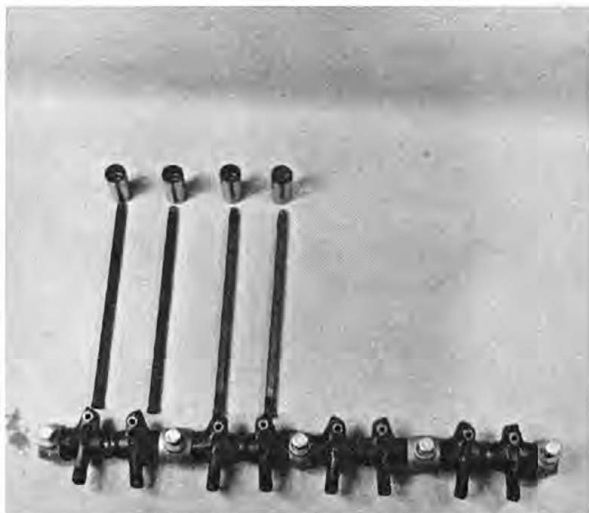
Beefy pushrods and adjustable cast rocker arms (above) are used with mechanical lifter. Shown at left, these parts were available through Chrysler Marine, but are now available from Chrysler car dealers as options,
