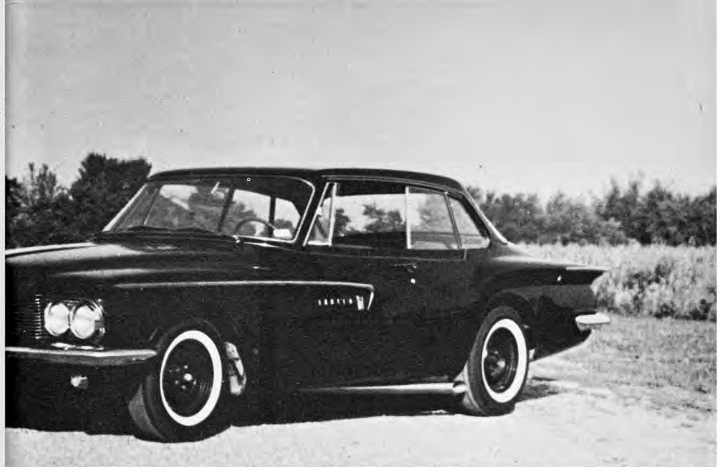
This Valiant looks almost stock . . . unless you note its partially concealed lakes pipes and a pair of oversized rear tires.
