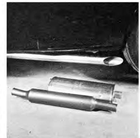
Either a Dodge Sono Ramic or two truck-type, straight-through mufflers may be used in souping.
