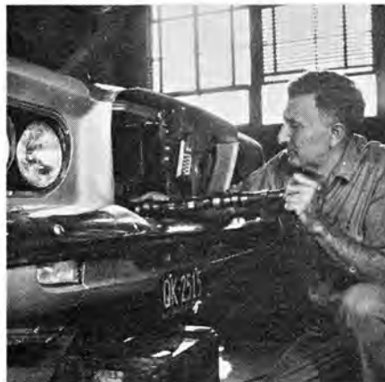
Cam may be changed, without removing engine, by pulling grille. Timing on Kuhl cam is about same as on the Hyper Pak.
