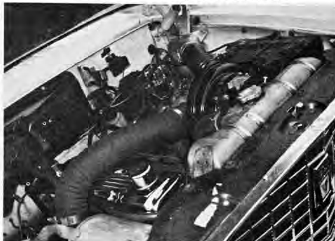
Large plenum chamber of intake manifold (left) leads to branches tuned for peak torque at given rpm. You'll save money by making your own. Paxton blower installation (below) delivers air to a pressurized plenum chamber over the carb. Volumetric efficiency, torque are improved throughout.
