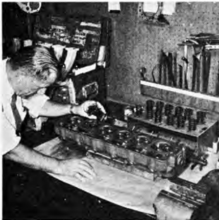
Measure combustion chamber volumes with a burette and equalize them by grinding. Take into account piston-to-deck clearance variations.
