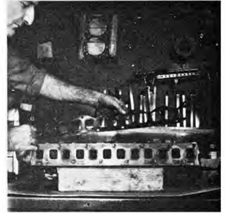
Use manifold gasket as pattern in laying out ports. Deposit traces show amount of mismatch on stock parts.
