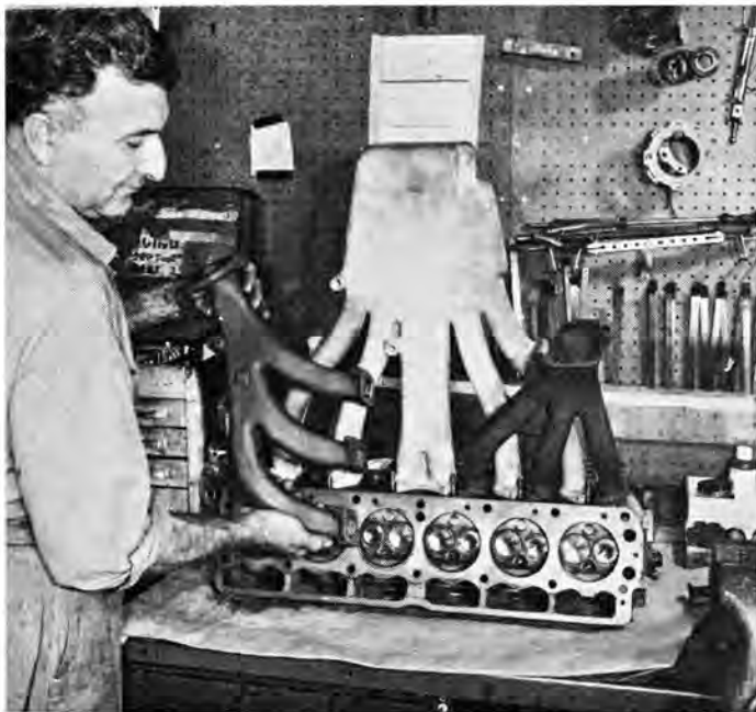
Large plenum chamber of intake manifold (left) leads to branches tuned for peak torque at given rpm. You'll save money by making your own. Paxton blower installation (below) delivers air to a pressurized plenum chamber over the carb. Volumetric efficiency, torque are improved throughout.
