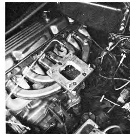
Long studs fasten adapter to a milled surface on the manifold, opened to match adapter plate.
