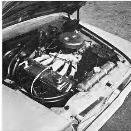
Completed Hyper Pak installations have earned owners many trophies. Long branch exhausts require reworking of starter, movement of parts.
