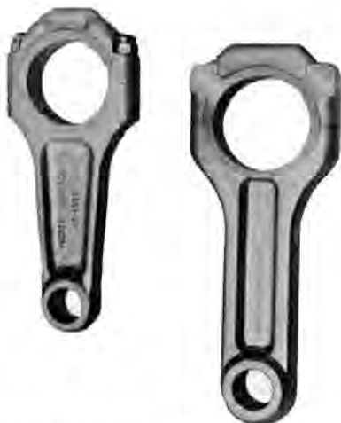
Forged aluminum rods offer considerable weight saving. Leave ample shoulders at the journals' sides.
