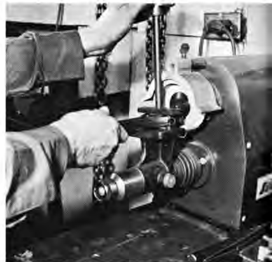
Cap and rod distort and stretch lengthwise under pounding in high speed engine operation. Parting faces, rod bores must be trued.
