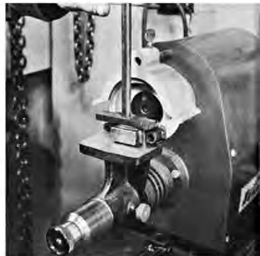
Caps and rods are clamped in handle, swung back and forth past grinding wheel with very fine grit. Micrometer feed controls cut.
