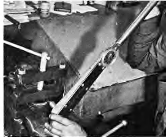
Clamp the rod flat at its big end and torque it accurately. Never clamp a rod at the web and twist. The rod will deflect in competition use.
