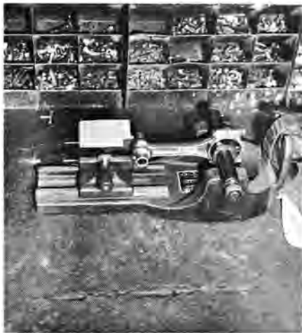
Check for bends and twists. Straightening a rod is bad; it will always return to shape after running. Alignment boring is the only proper cure.
