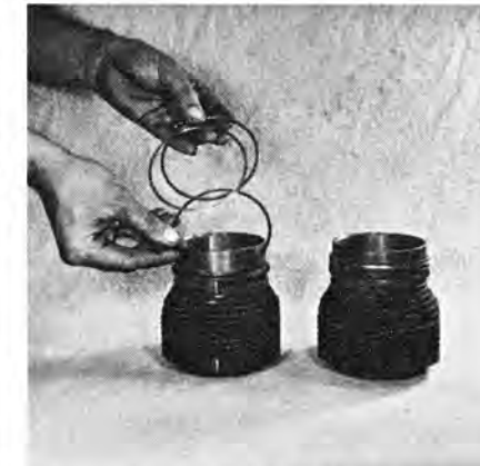
Spacer rings under cylinder barrels allow avoiding special piston cost.
