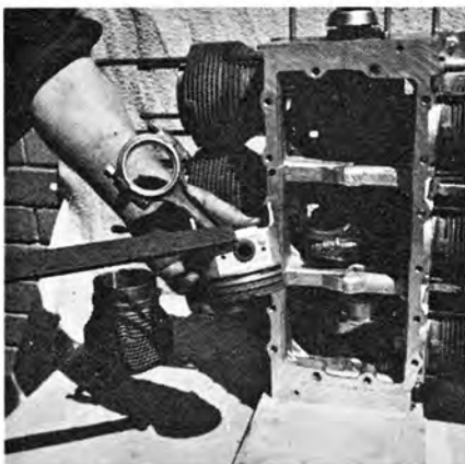
Bottoms of pistons must be touched up with file for adequate clearance.
