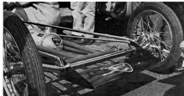
The wind can be used to do many things, as demonstrated by this airfoil on front of the 170-mph Adams-McEwen drag machine. Angle of wing puts pressure on front end at speed.
