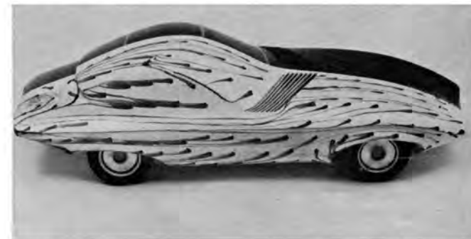
Potential automotive designers at Art Center school in Los Angeles perform air flow studies by spotting scaled models with liquid dye and subjecting them to strong blast of air.
