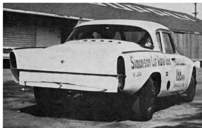
Photos above show technique used by John Simonson on his 188-mph Stude. Air is scooped from high pressure area under car, discharged at negative pressure point behind the rear window to reduce drag and lift. Center photos show ducting: engine compartment air is exhausted to the negative pressure areas behind the doors, where pressure differential is beneficial; underbody air is ducted up behind seat. Bottom photos show fender vents for trapped air, hood streamlining for blower.
