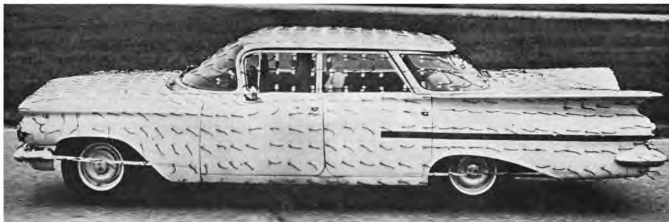
A 1959 Chevrolet performing a tuft study. The hood and top seem to have attached flow, but other areas show various degrees of turbulence and eddying. We see that the open wheel areas are also being checked with tufts attached to special bar.
