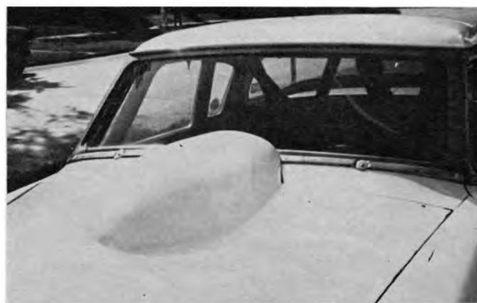
Photos above show technique used by John Simonson on his 188-mph Stude. Air is scooped from high pressure area under car, discharged at negative pressure point behind the rear window to reduce drag and lift. Center photos show ducting: engine compartment air is exhausted to the negative pressure areas behind the doors, where pressure differential is beneficial; underbody air is ducted up behind seat. Bottom photos show fender vents for trapped air, hood streamlining for blower.
