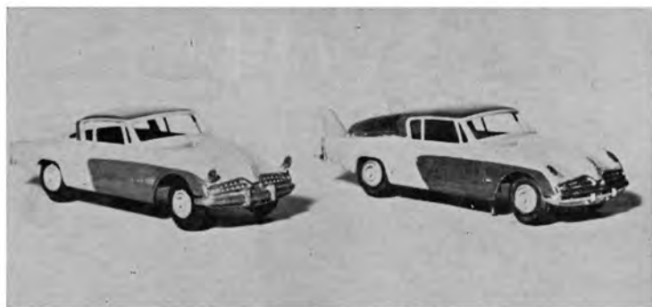
Two 1/25 scale '53 Studebakers used in wind tunnel experiments at Davidson Laboratory of Stevens Institute of Technology. Note body extension and fins used to reduce air drag. Also shown is Dr. Kamm's K-5 model undergoing tuft studies. Attached flow is visible on top and sides. This model has neutral lift, excellent performance and fuel economy. The C_d is about .25.
