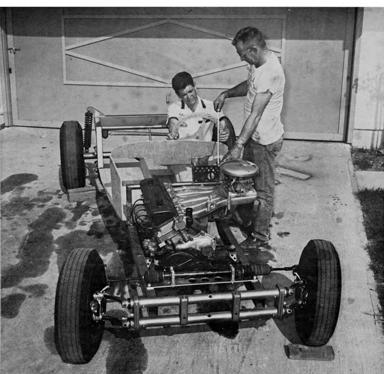
ABOVE — LeRoi Smith and his father, Carlos, do preliminary measuring prior to mounting steering wheel in the XR-6. A wood expert, Carlos is building special steering wheel, inlaid pickup bed. The sketches on the facing page were drawn up by designer Steve Swaja. FAR LEFT—Cal Automotive fiberglass '27 'T' body is channeled the width of frame. When finished it will be quick-disconnect from the chassis and cockpit. LEFT — Morris Minor rack and pinion steering gear is bolted to \frac{1}{4} -inch aluminum plate between frame rails. MG extensions were fitted to stretch tie rod ends to the Volkswagen steering arms. RIGHT — Lancer rear end supports the package with plenty of clearance. With pattern plywood cockpit panels in place, body is tried on for fit. Speed Improvements built the reversed rear wheels.
