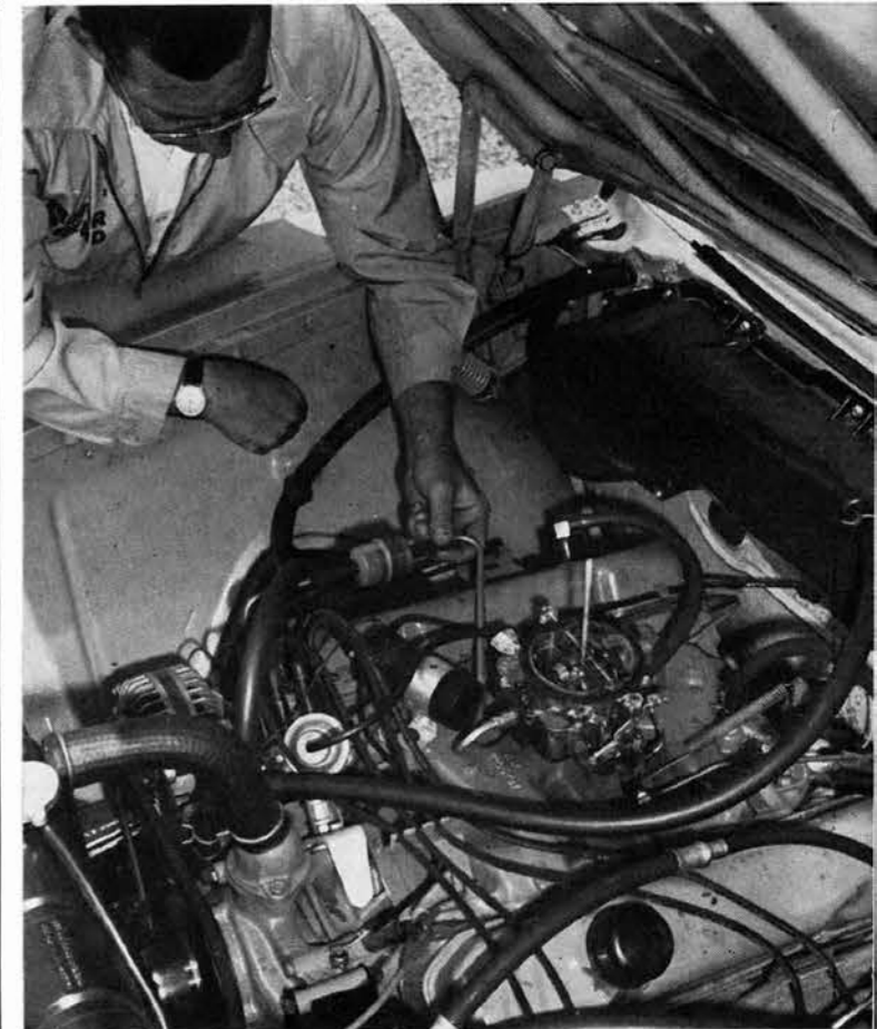
Engine performance is above average, considering the 361-cubic-incher is breathing through a two-barrel carburetor and has only a nine-to-one compression ratio.
