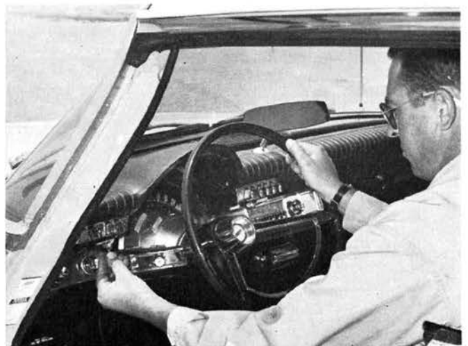
Dash-mounted turn indicator is inconvenient and seems to be prone to failure. Instrumentation is complete but layout is poor and daytime visibility is bad.
