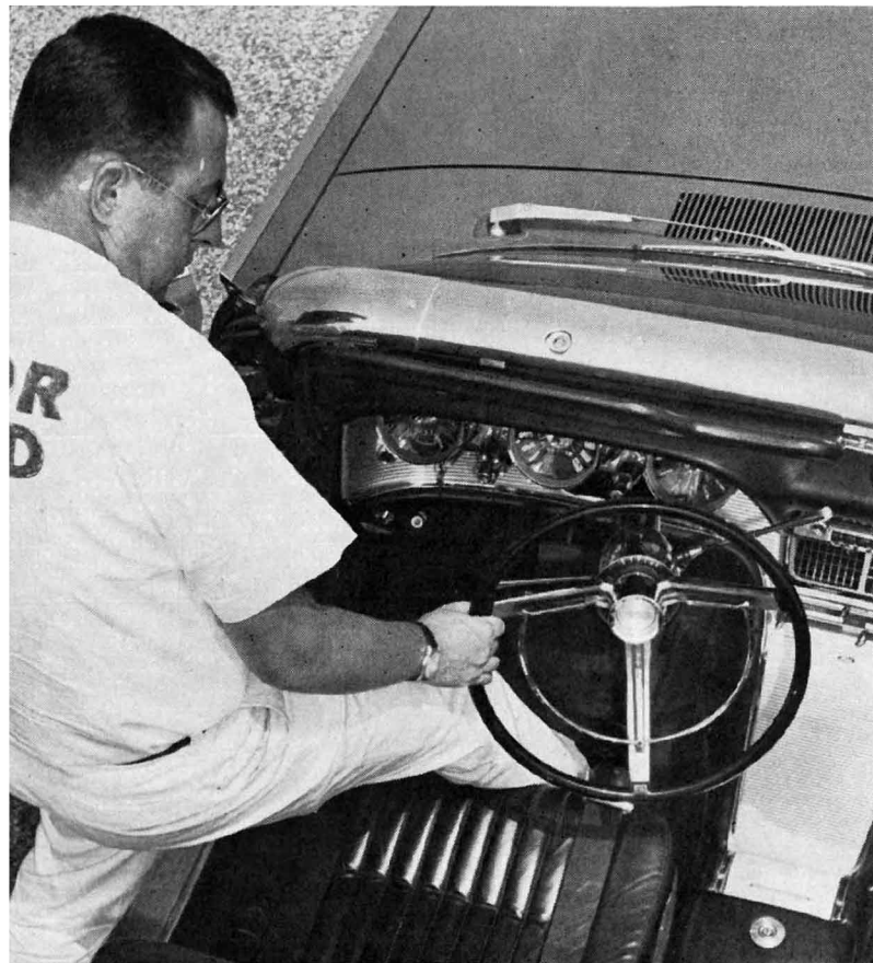
Swing-away steering wheel is now offered as standard equipment. Unit makes for easier entry but would be more effective if it were also adjustable fore and aft.
