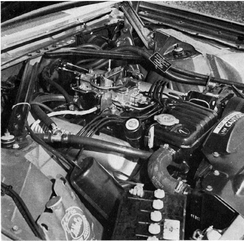
Power accessory plumbing, radiator header tank and spring towers limit engine accessibility and hamper simple servicing.
