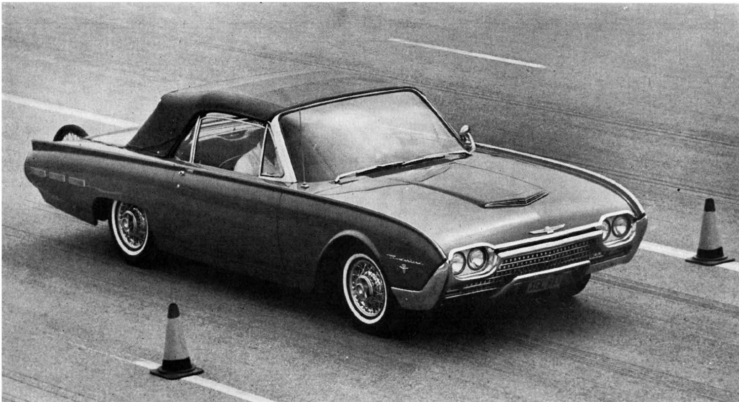
WIRE WHEELS HELP PROMOTE MORE EFFECTIVE BRAKE COOLING, BUT ONCE FADED, THE BRAKES STILL REQUIRE TOO LONG A COOL-DOWN PERIOD.
