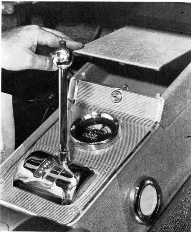
Shift lever is well located and has a positive feel to it. A simple vacuum/pressure gauge would be more effective than the "tell-nothing" economy/power gauge.
