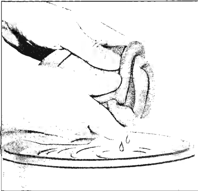
Fig. 37—Cleaning Polyurethane Element
