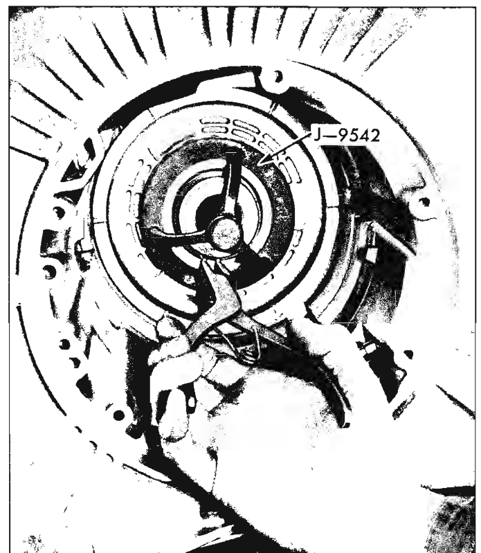
Fig. 13—Removing Rear Piston Spring Retainer Snap Ring
