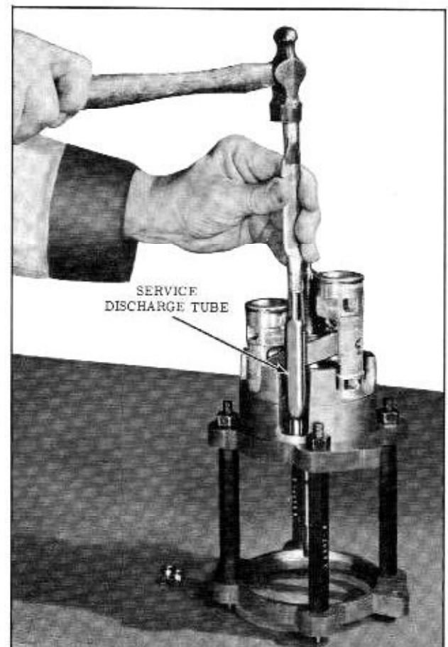
Fig. 14-54 Installing Discharge Tube
