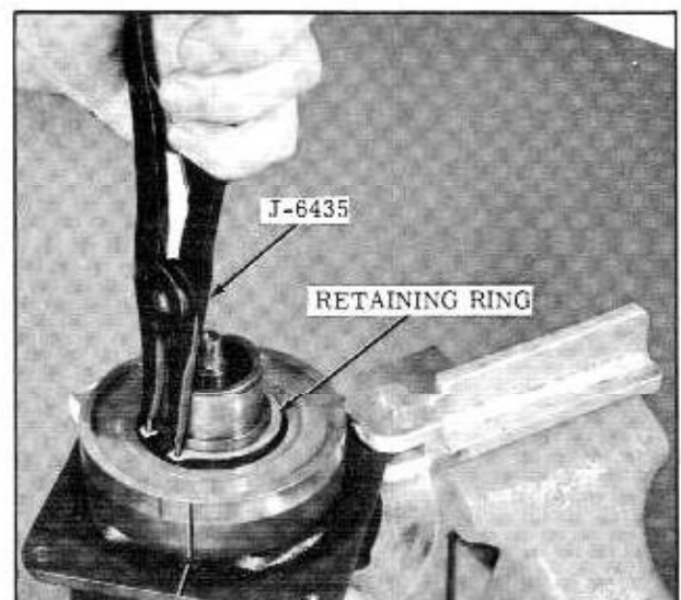
Fig. 14-28 Removing Coil Housing Retaining Ring
