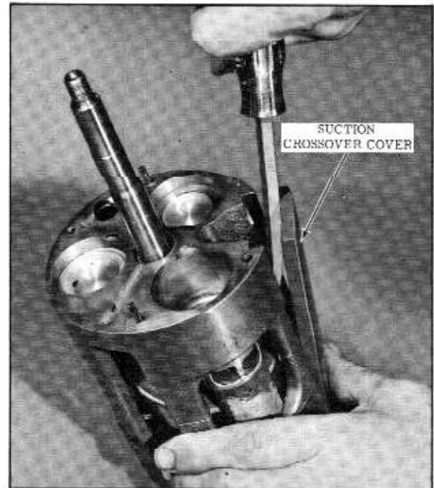
Fig. 14-45 Removing Suction Crossover Cover
