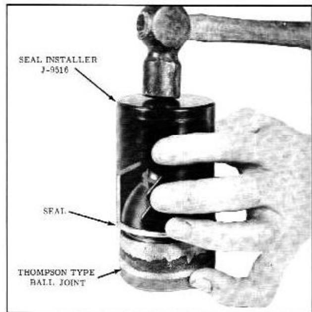
Fig. 5-6 Installation of Thompson Type Seal
