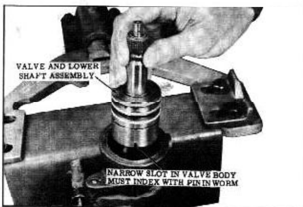
Fig. 4-28 Installing Valve and Lower Shaft
