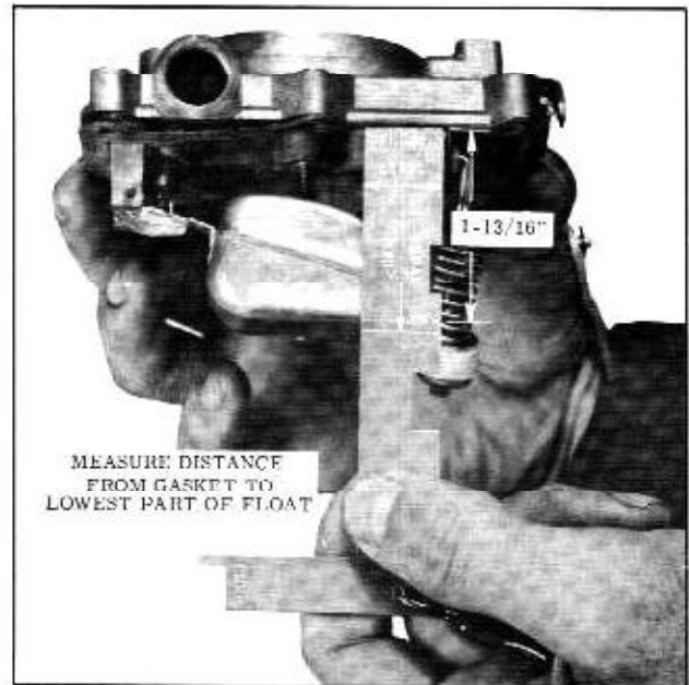
Fig. 8-110 Float Drop Adjustment
