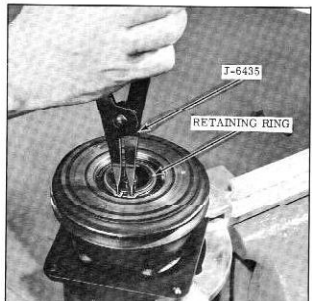
Fig. 14-24 Removing Pulley Retaining Ring
