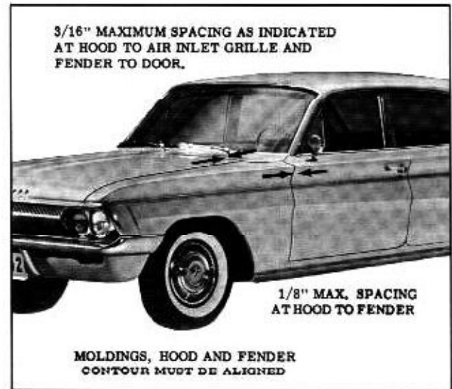
Fig. 11-3 Hood and Fender Clearances
