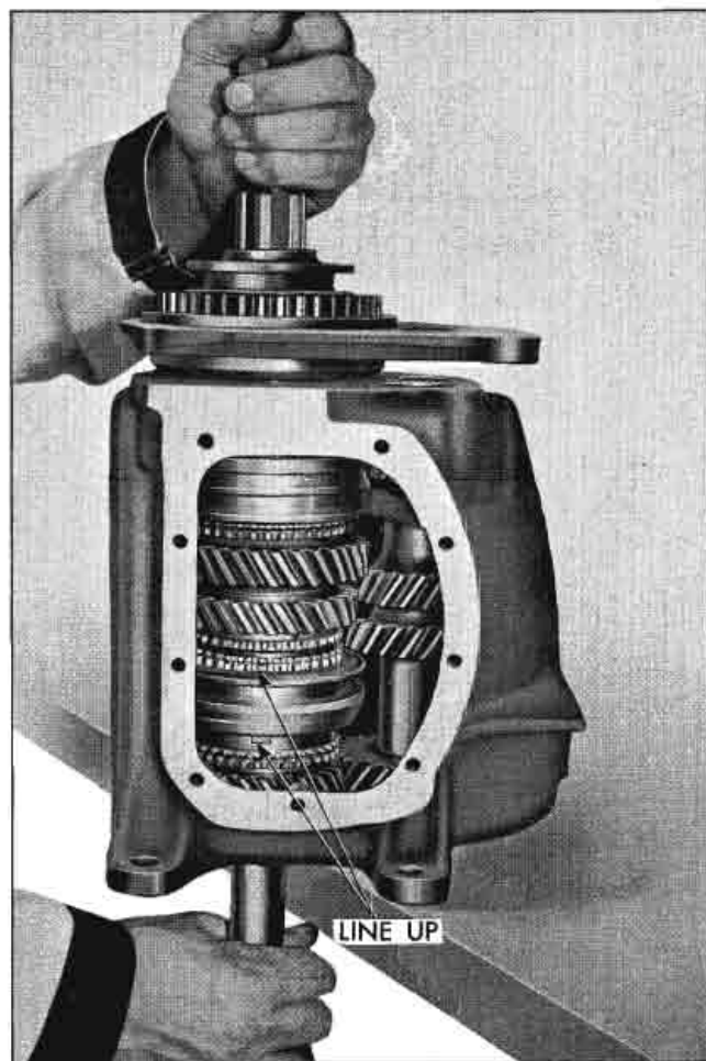
Fig. 7B-30 Installing Mainshaft Assembly
