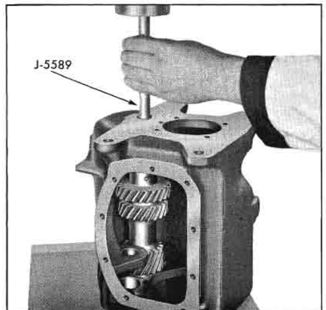
Fig. 7B-15 Removal of Countershaft
