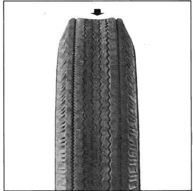
Fig. 3A-5 Wear from Overinflation
