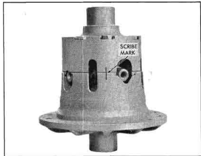
Fig. 4-63 Alignment Marks on Differential Case Halves
