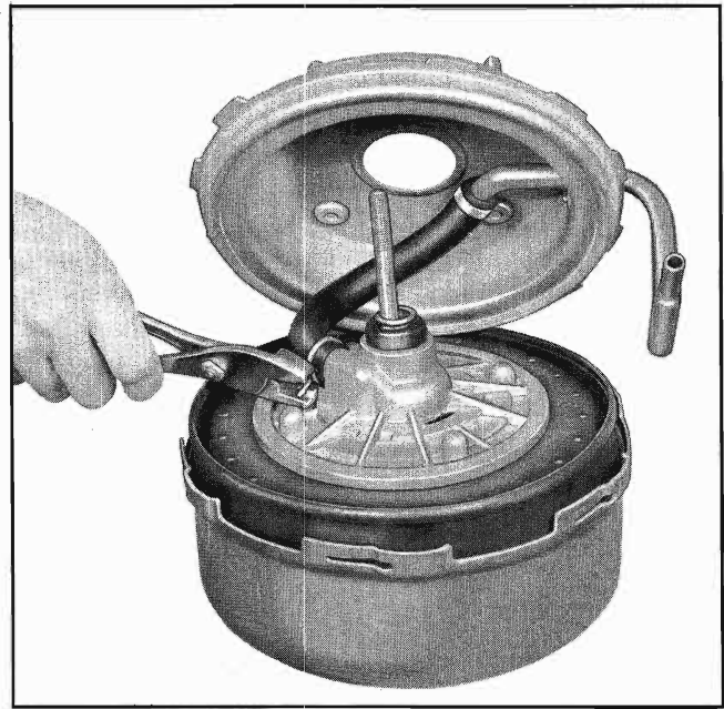
Fig. 5-M-21 Connecting Exhaust Hose
