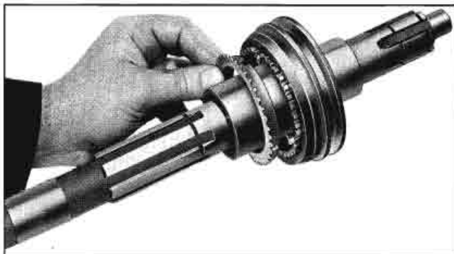
Fig. 7B-22 Installing Synchronizer Ring
