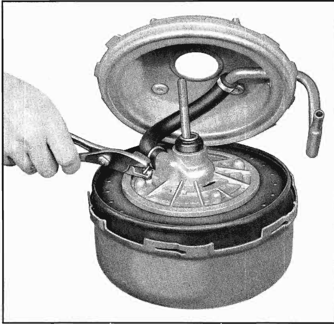
Fig. 5-M-7 Disconnecting Exhaust Hose
