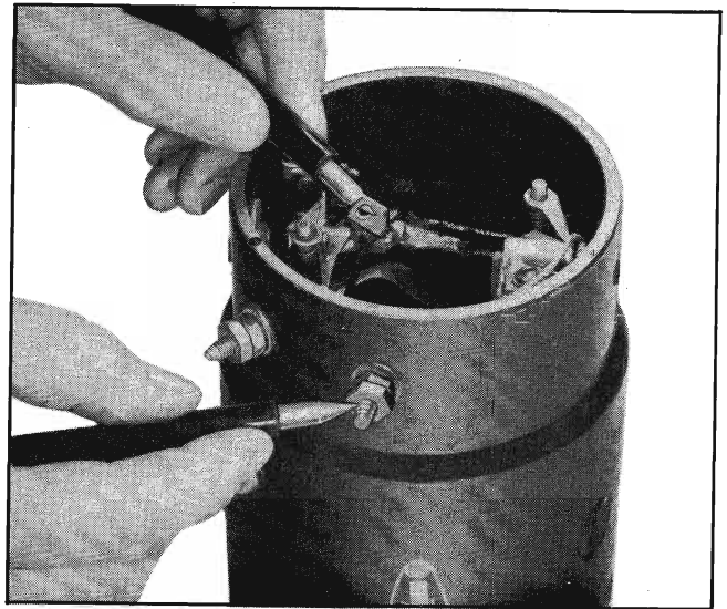
Fig. 11-14 Testing Field Coils for Open Circuit
