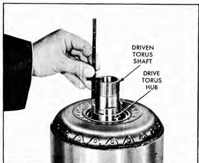
Fig. 163 Measuring Wear of Coupling Thrust Washer
