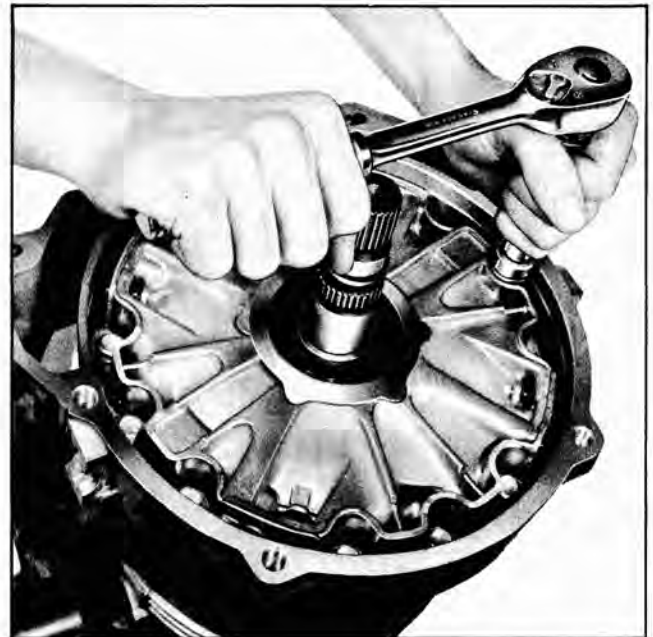
Fig. 54 Removing Torus Cover Bolts
