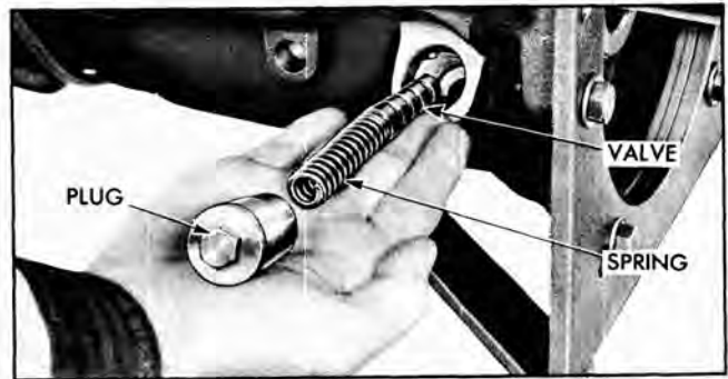
Fig. 162 Installing Pressure Regulator
