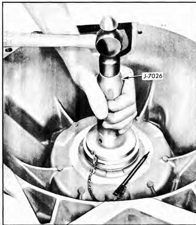
Fig. 142 Installing Flywheel Housing Oil Seal
