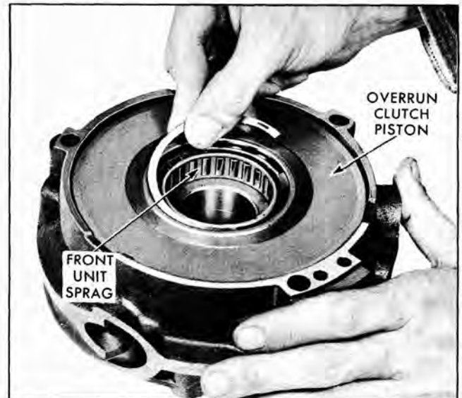
Fig. 104 Removing Front Sprag Retaining Ring
