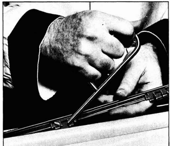
Fig. 14-4 Sealing Strip Removal
