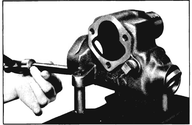
Fig. 9-25 Removing Upper Bearing Seal
