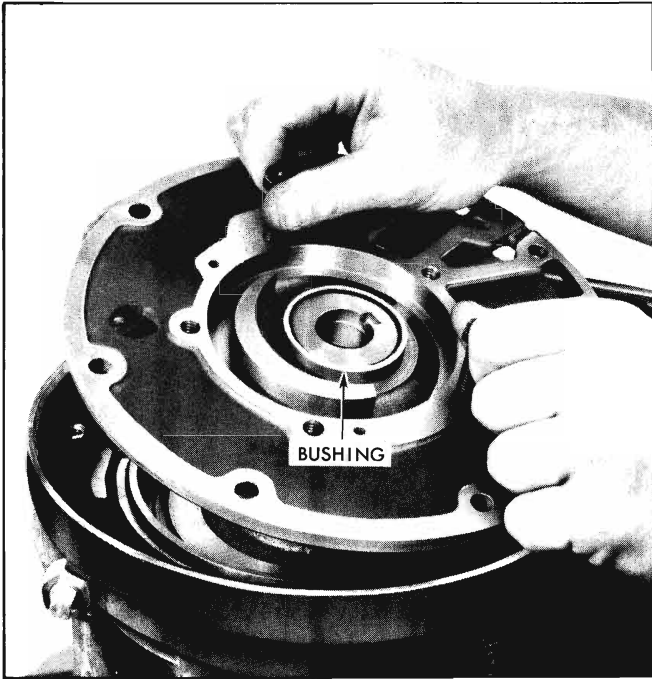
Fig. 7A-35 Removing Pump Body
