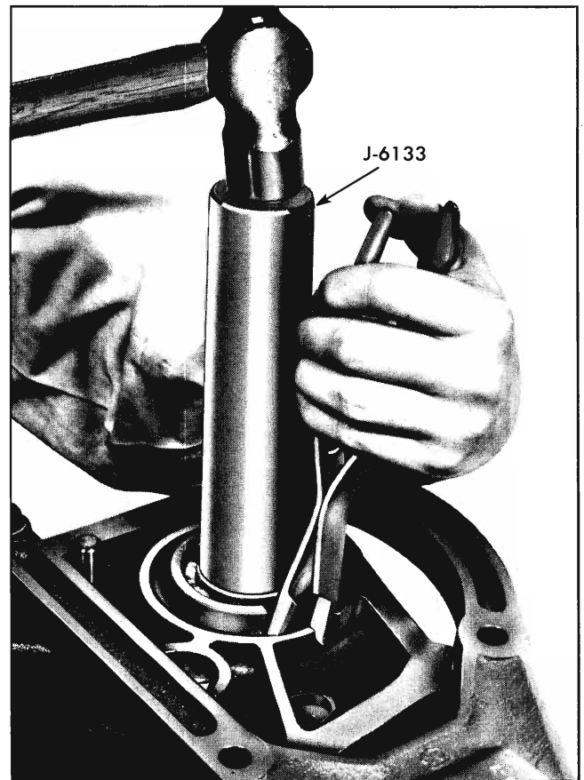
Fig. 7-51 Installing Mainshaft Bearing
