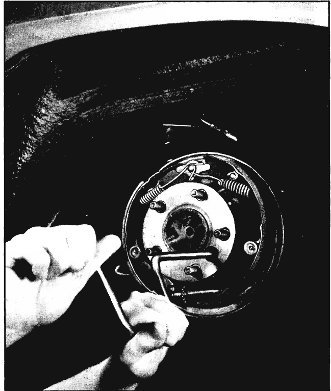
Fig. 4-5 Removing Nuts from Axle Shaft Bearing Retainer
