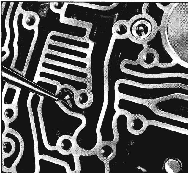
Fig. 7A-25 Removing Front Pump Air Bleed Ball
