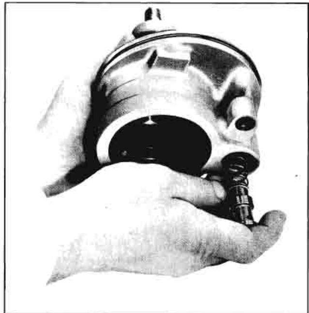
Fig. 9A-10 Removing Flow Control Valve
