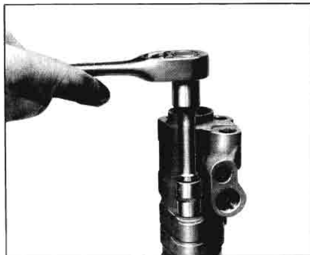
Fig. 9A-30 Removing Valve to Adapter Bolts
