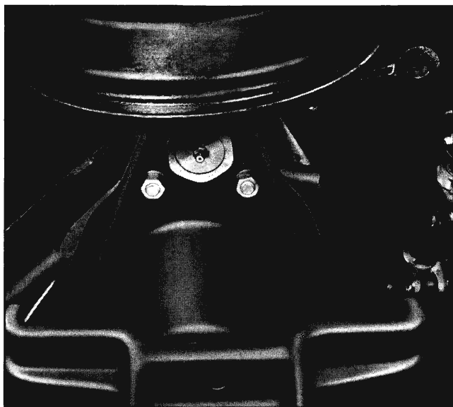
Fig. 3-16 Strut Rod Front Retaining Nuts
