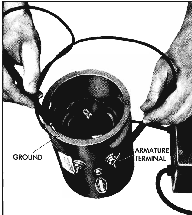
Fig. 11-27 Testing Armature Terminal for Ground on 35 Amp Generator
