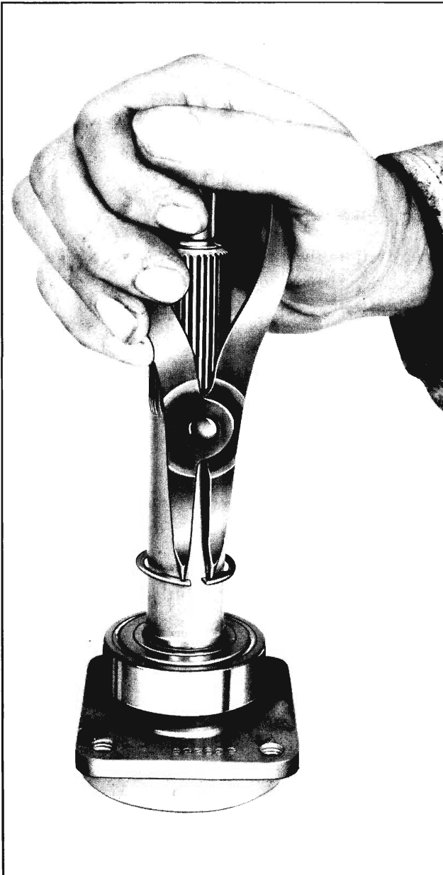
Fig. 6D-8 Removing Drive Shaft Bearing Retainer
