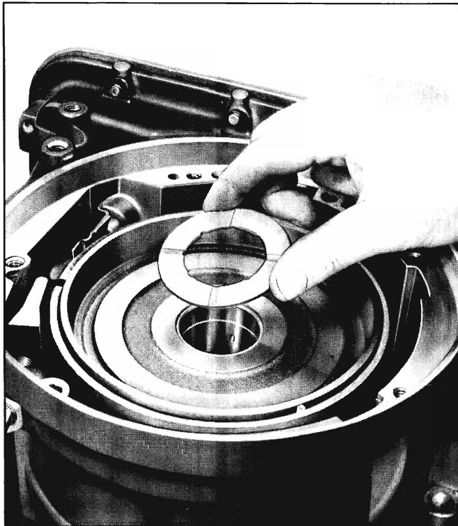
Fig. 7A-36 Removing Clutch Drum Thrust Washer
