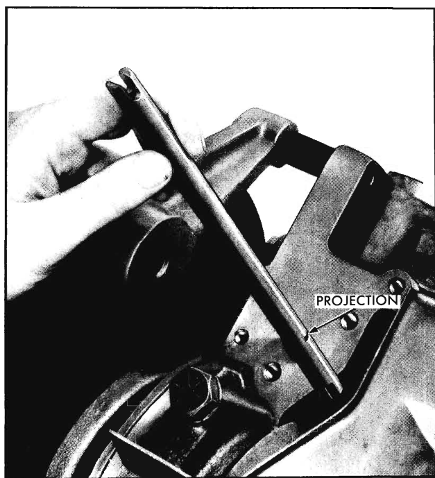
Fig. 6A-13 Positioning 4 Cylinder Engine Pump Drive Shaft
