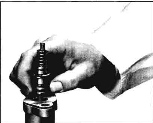
Fig. 9A-33 Removing Reaction Components
