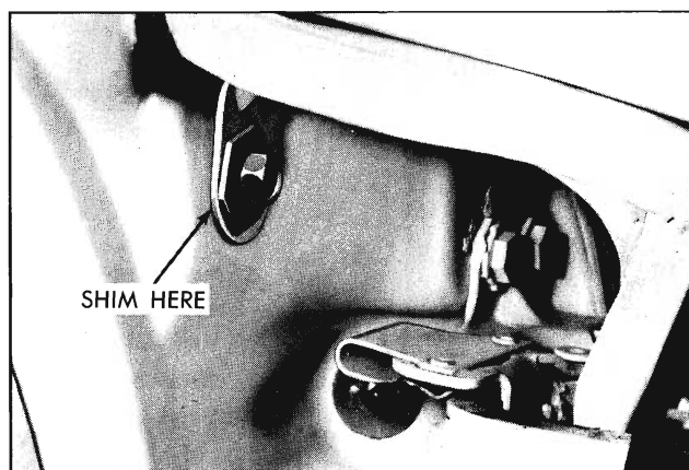
Fig. 10-1 Upper Fender Adjusting Bolt
