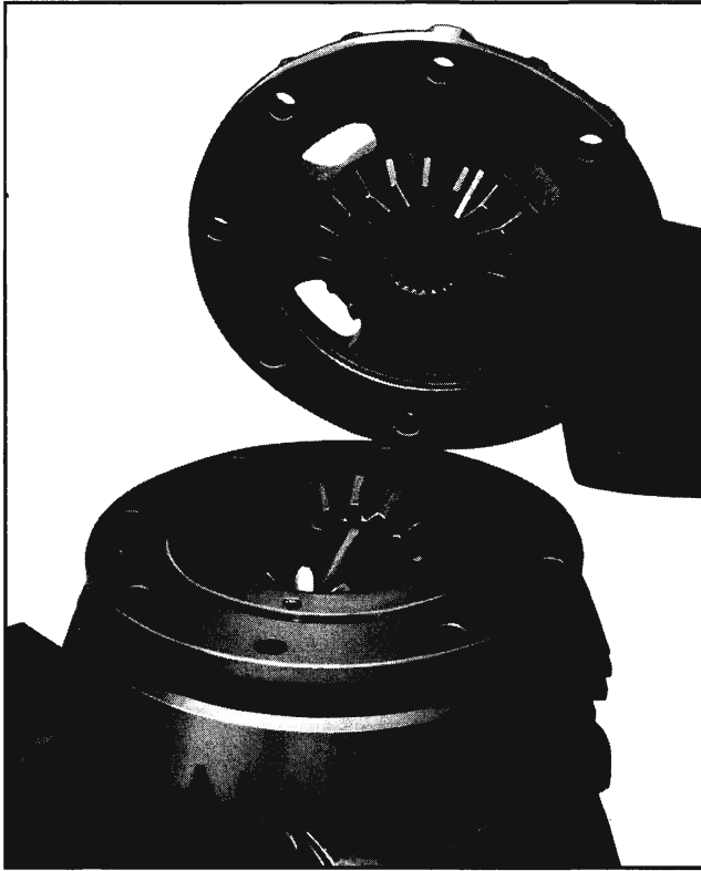
Fig. 4-32 Separating Cover and Case
