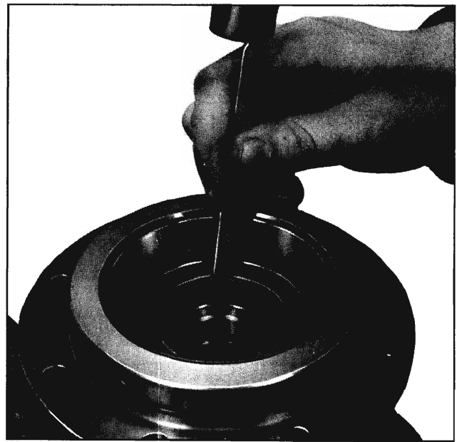
Fig. 4-47 Removing Rear Pinion Oil Seal
