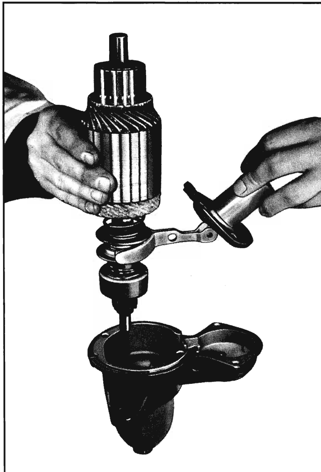
Fig. 11-13 Installing Armature and Plunger
