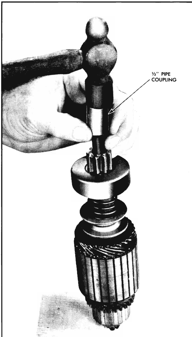
Fig. 11-8 Driving Retainer Off Snap Ring
