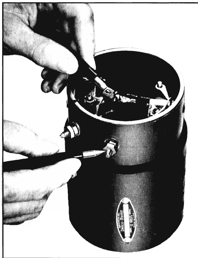
Fig. 11-22 Testing Field Coils for Open Circuit on 30 Amp. Generators
