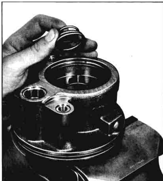
Fig. 9A-21 Installing Pressure Plate Spring
