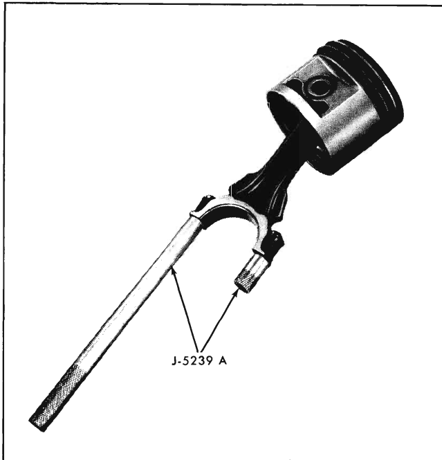
Fig. 6-107 Connecting Rod Bolt Set
