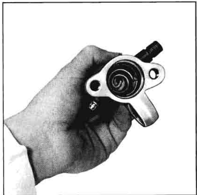
Fig. 9A-43 Ball Seat Spring Installed
