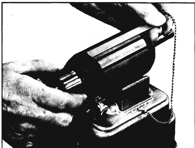
Fig. 11-19 Testing Armature for Shorts
