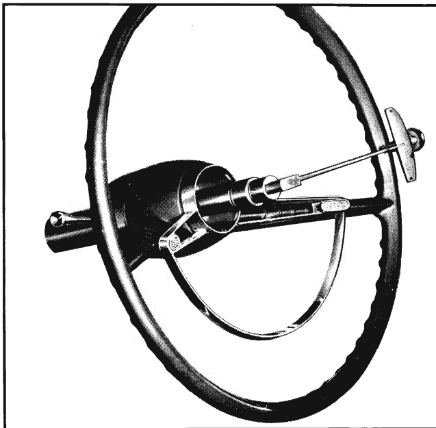
Fig. 9-18 Checking Pull at Wheel
