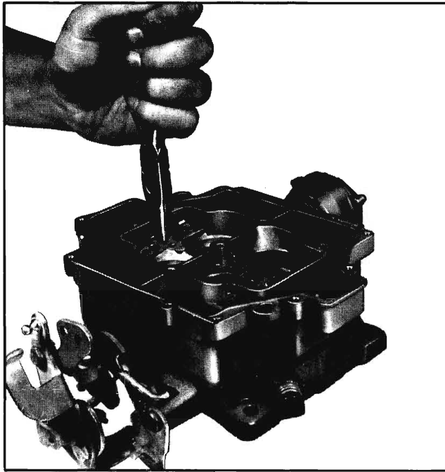
Fig. 6B-56 Removing Pump Discharge Spring
