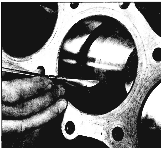
Fig. 6-111 Checking Ring Gap
