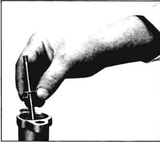
Fig. 9A-36 Removing Plug to Sleeve Key
