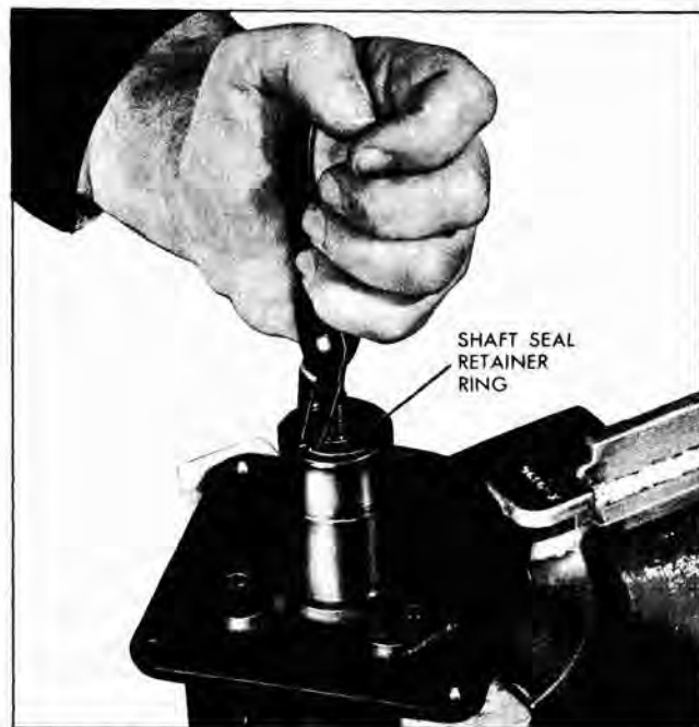
Fig. 5-64 Removing Shaft Seal Retainer
