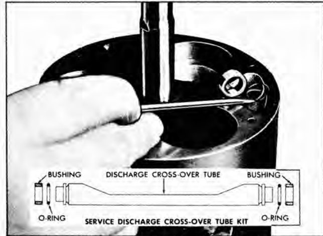
Fig. 5-91 Installing Service Discharge Crossover Parts
