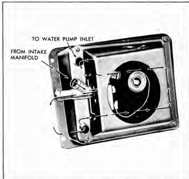
Fig. 2-6 Flow of Engine Coolant Through Valve and Core
