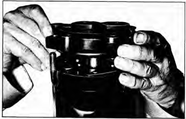
Fig. 5-97 Installing Rear Head
