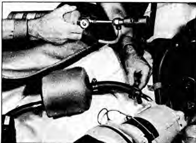
Fig. 6-20 Searching for Leaks
