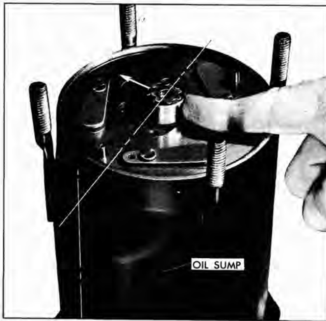
Fig. 5-96 Positioning Oil Pump Outer Gear
