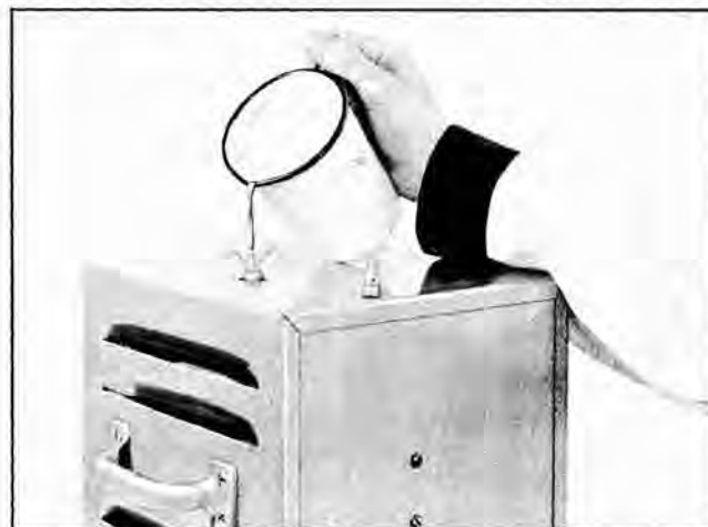
Fig. 4-7 Adding Oil To Pump
