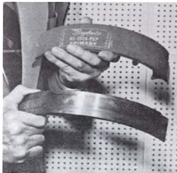
Standard brake lining, top, alongside Raybestos copper lining at bottom.
