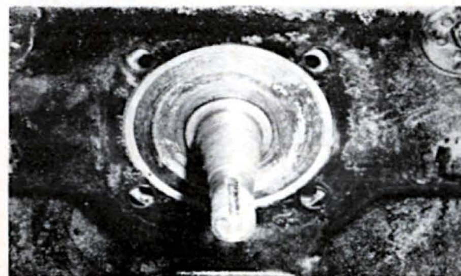
Large center positioning hole in hydraulic backing plates is larger than early brakes. Spacer ring must be used.
