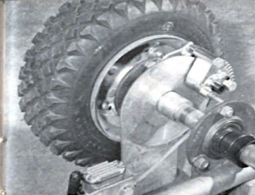
New Airheart disc brake for karts is small, has been used on lightweight Formula Junior racers.
