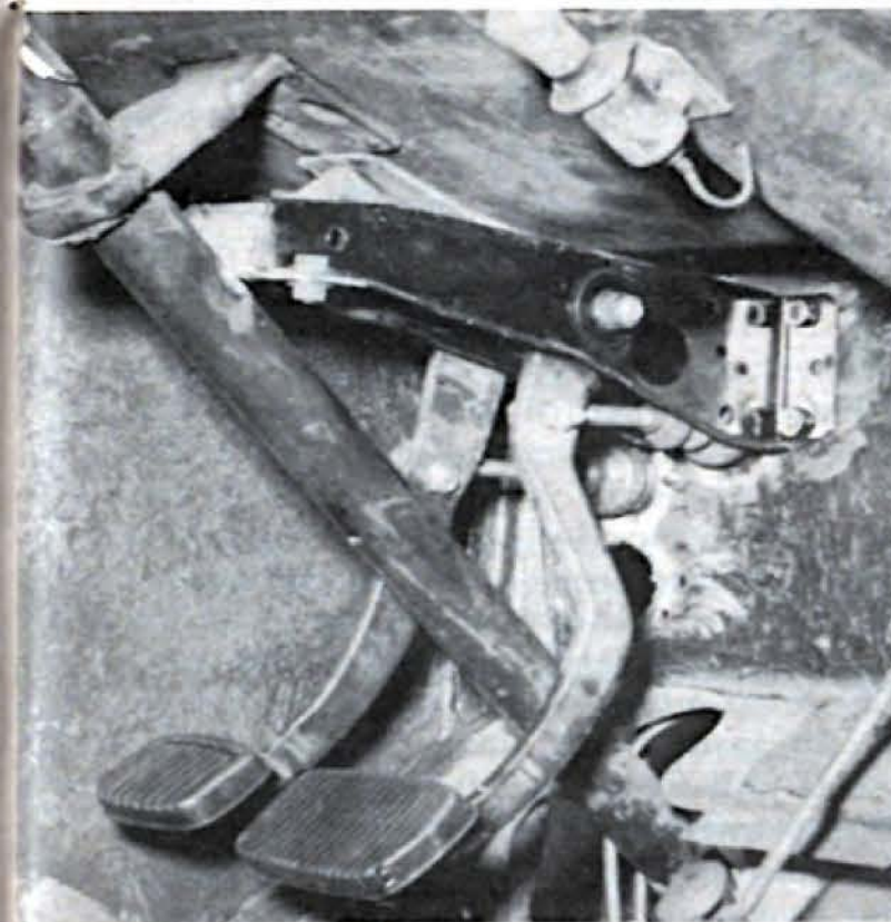
Swinging brake and clutch pedals from late model cars easily fit older vehicles, like the Model A, with minimum mount problems.
