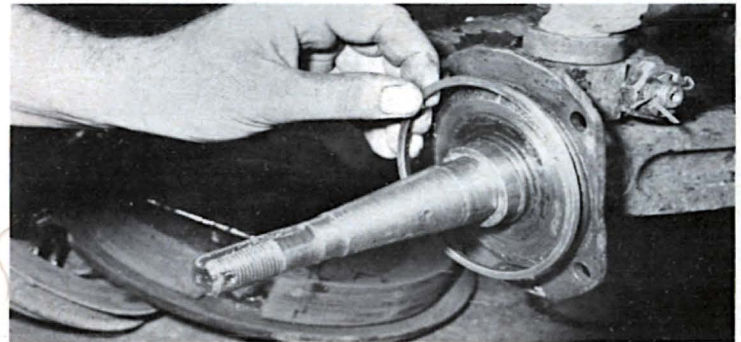
Large center positioning hole in hydraulic backing plates is larger than early brakes. Spacer ring must be used.
