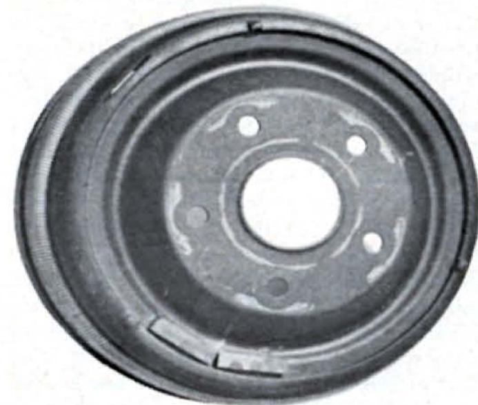
The Lincoln brake drum used during mid-1950's had cast-iron friction surface and steel center section. Heavy outer springs help to control drum distortion. Photo at the left shows a typical ratchet brake adjusting mechanism being contacted through backing plate by tool.
