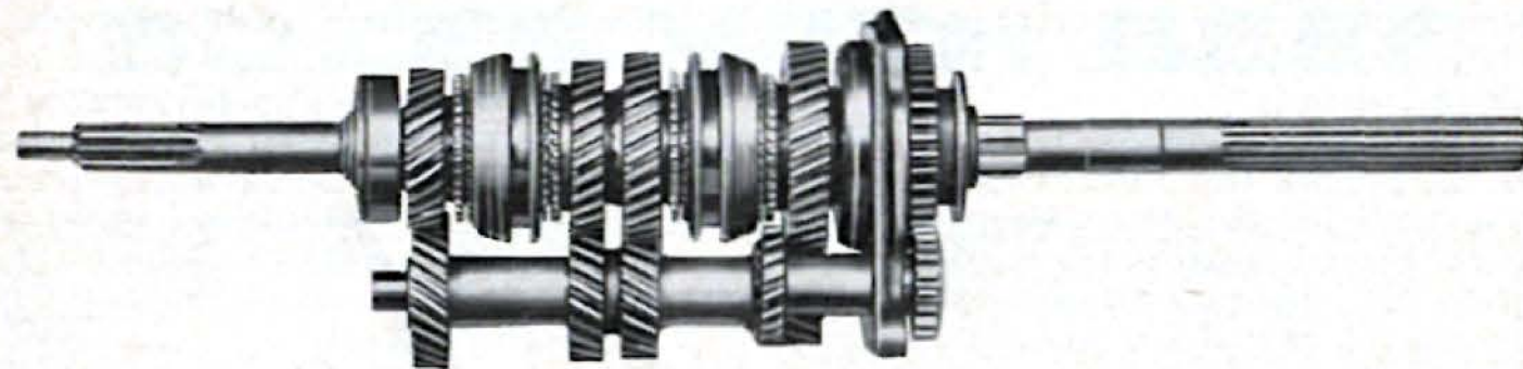
Warner 4-speed originally developed for Corvette is now offered on a total of eight different makes. Gears shown above are wider ratio set designed for big car use.
