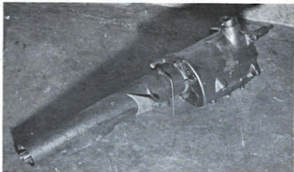
The original Cad-La Salle unit has an extremely long tail shaft that must be cut down to fit most other cars. Compare this box with the Cad-La Salle modified for a Chevy, shown on page 15.
