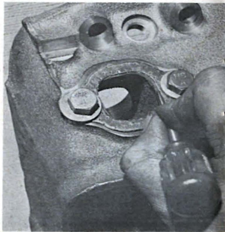
A gasket and a scribe are used to mark an exhaust port as a guide for enlarging.
