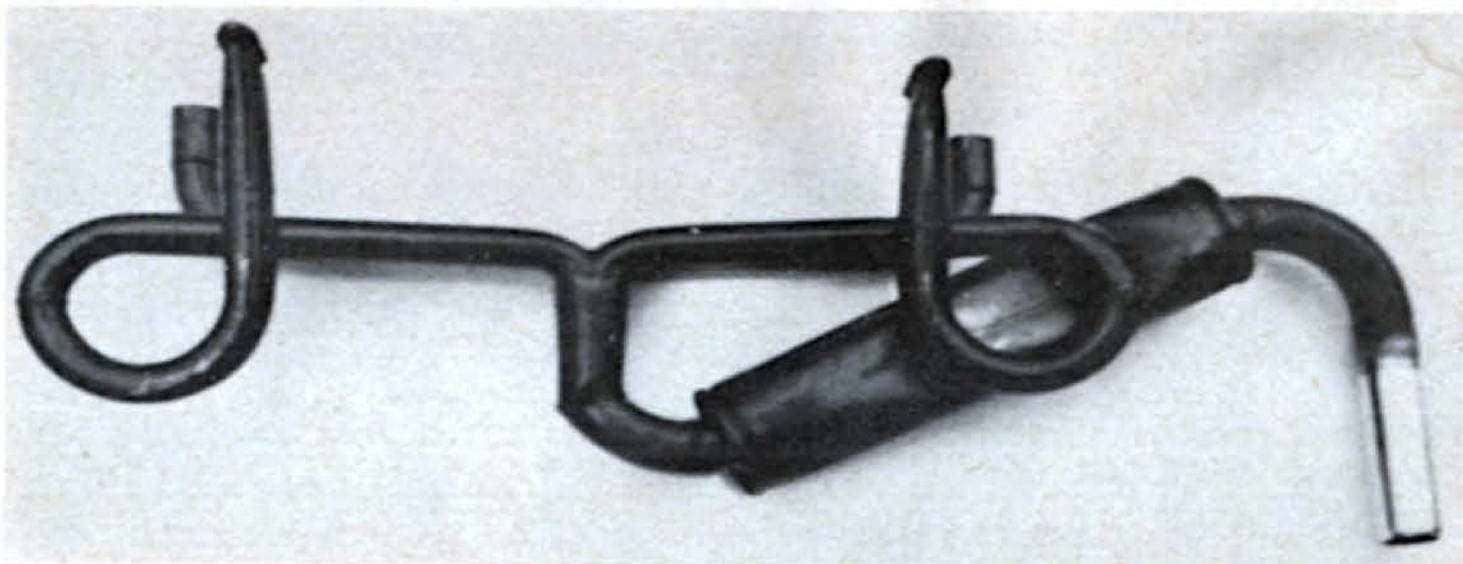
Each cylinder in a Porsche has a pipe of equal length with this Horse Power Eng. setup.
