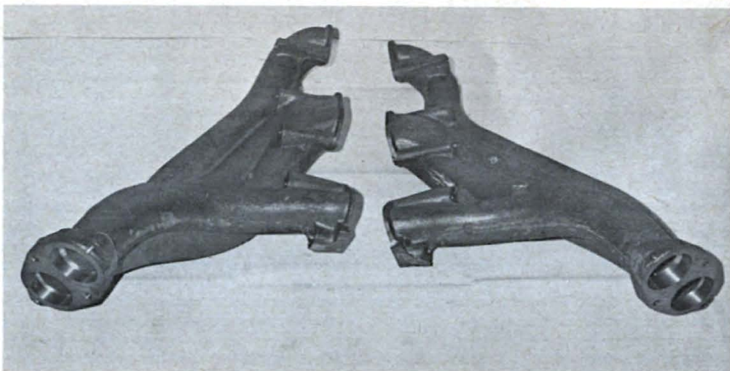
The best of Pontiac's heavy-duty manifolds are cast-iron headers, with dual outlets.
