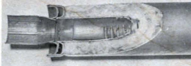
Visible in this cutaway display muffler are the innards of an Advance glass-pack.
