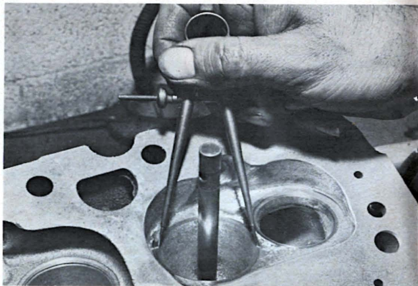
Valve seat diameters to match the new valve heads are easily established with dividers.
