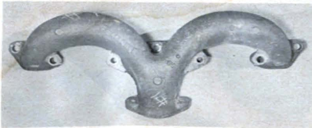
Another manifold of ram's horn design is this one from a racing kit for a 312-inch Ford.
