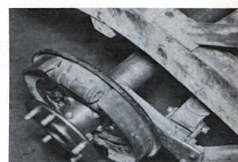
These housings were reversed to place spring ahead of axle, plate added alongside hangers to hold the modified radius rods. Tube axles are featured here.
