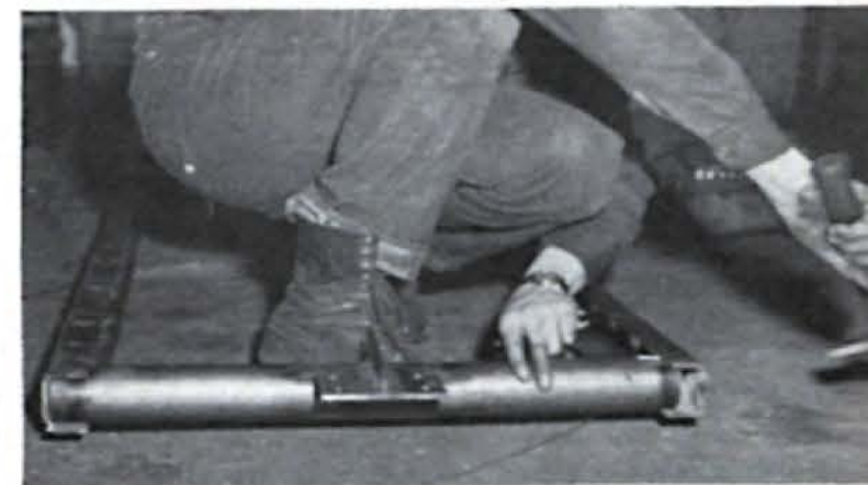
Front crossmember with bulldog perch is placed between 'A' rails, welded.
