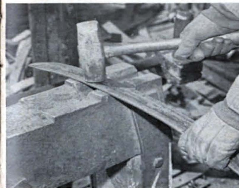
Pound main leaf with heavy hammer to flatten and curve the opposite direction. Go slowly, do not heat any spring leaf.
