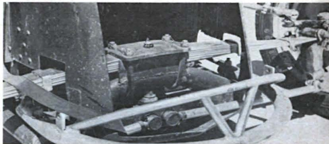
Unusual front end on early lakes rod had spring mounting above two locator bars. Idea is remotely similar to Studebaker front suspensions of the 1930-40 era.
