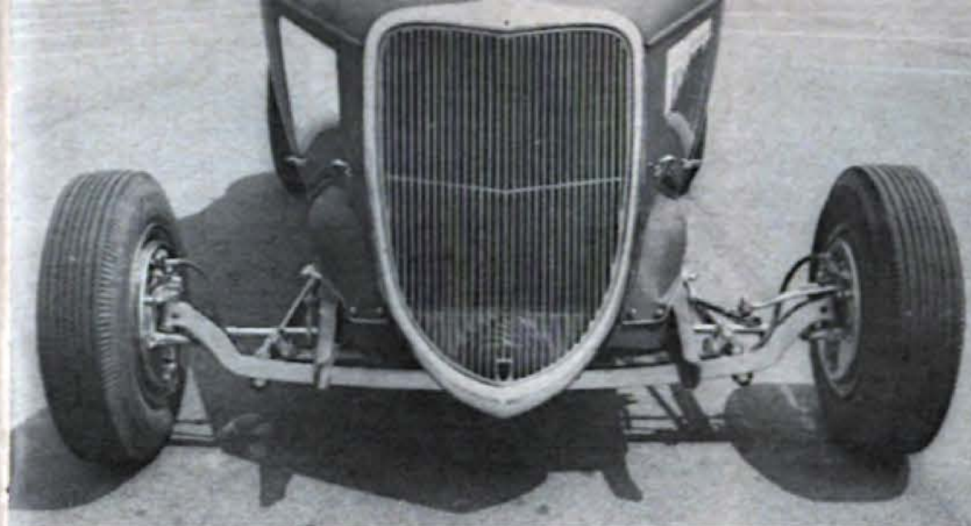
Unusual dropped axle has been filled clear across its length, gives good appearance.
