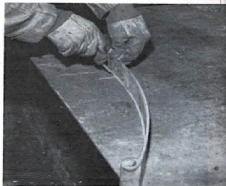
In de-arching, first mark contour of main leaf on fixed surface before starting to do any reshaping of the leaf.
