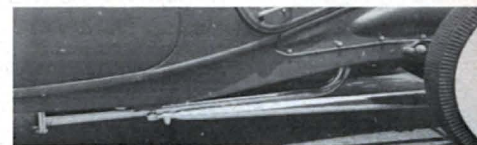
Tube front axle on this race car is located by individual radius rods, making caster adjustment easy. Note shock mounting plate.
