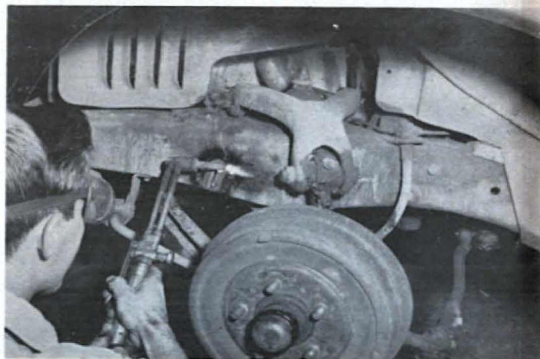
If lowered front end bottoms, mark area 2 in. deep and as wide as lower A-frame on bottom of frame. Cut with torch.
