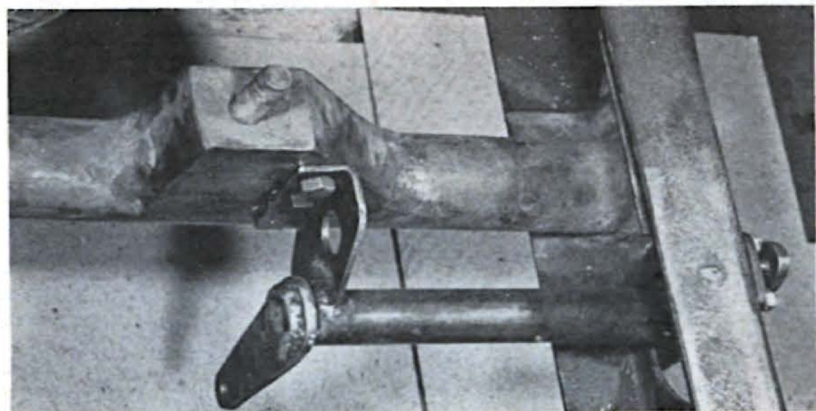
Tubing crossmember with transmission mounts bolts to 'A' frame.
