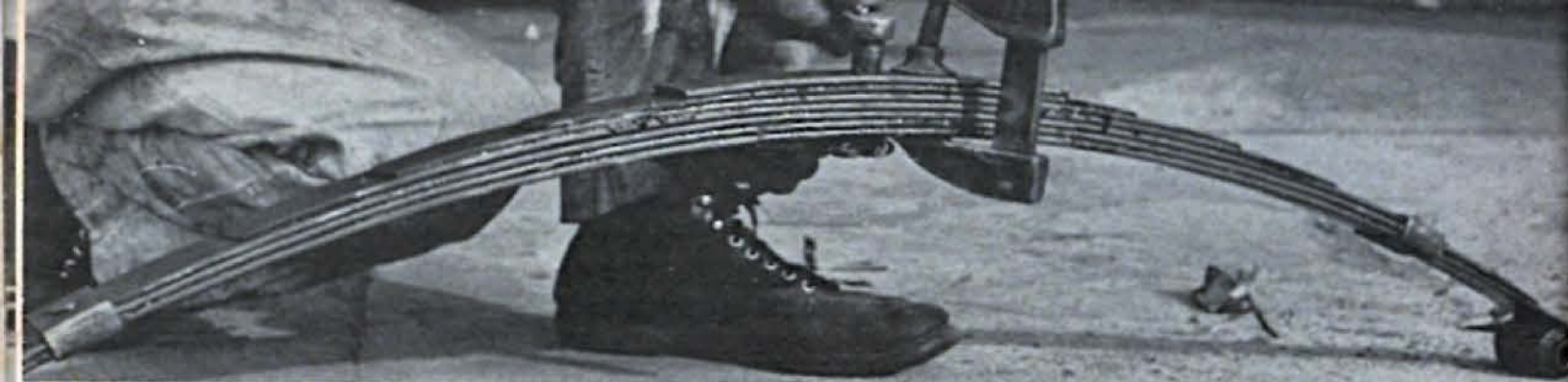
When dismantling and assembling a spring, always use a good C-clamp or vise. Clips at ends of the springs keep leaves in proper alignment. Replace broken leaves.
