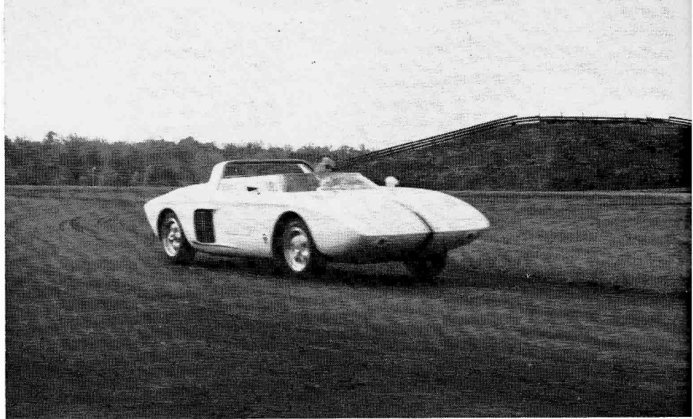
The combination of lightweight cast magnesium disc wheels from Lotus, braced-tread Pirelli Cinturatos and rack-and-pinion gave truly sporting cornering.
