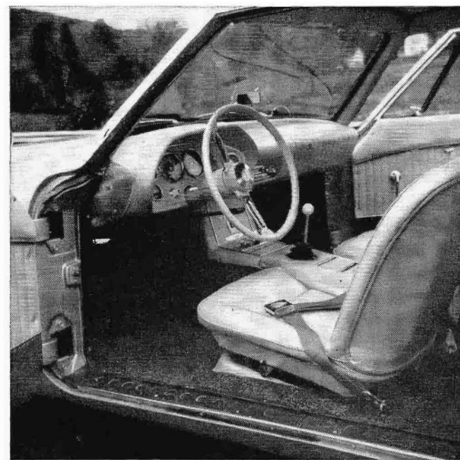
Cockpit incorporates many lessons from aviation, and areas you might come in contact with in accidents are all padded.
