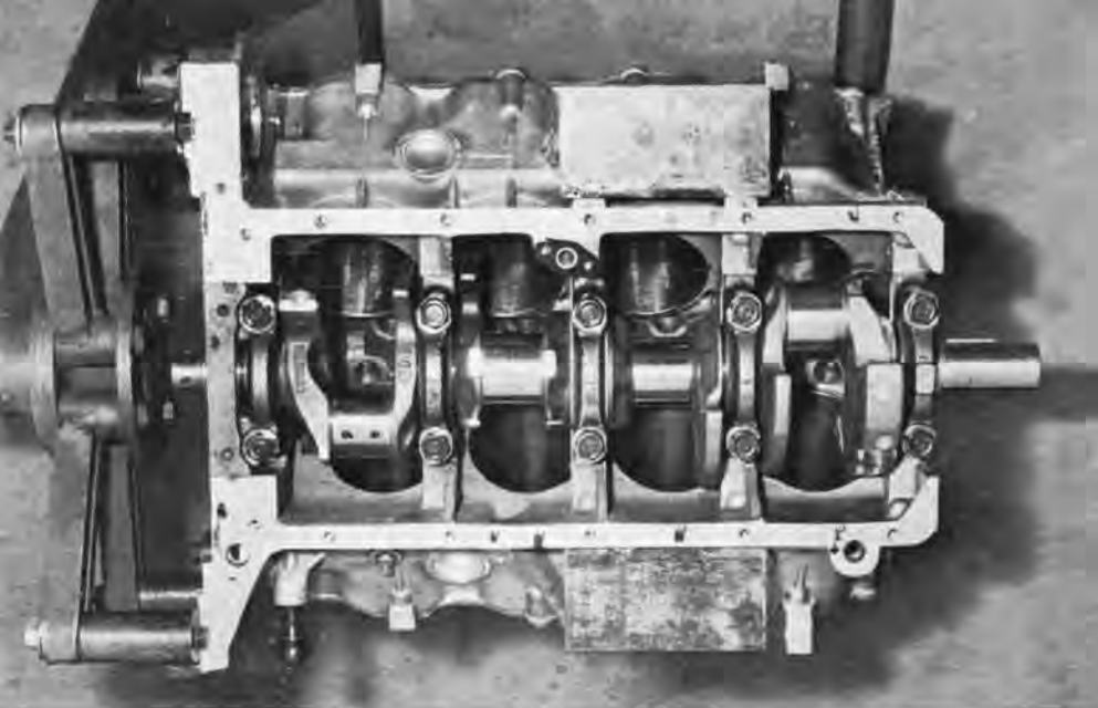
Despite lightweight block, bottom end is rugged enough for strong increase in power.
