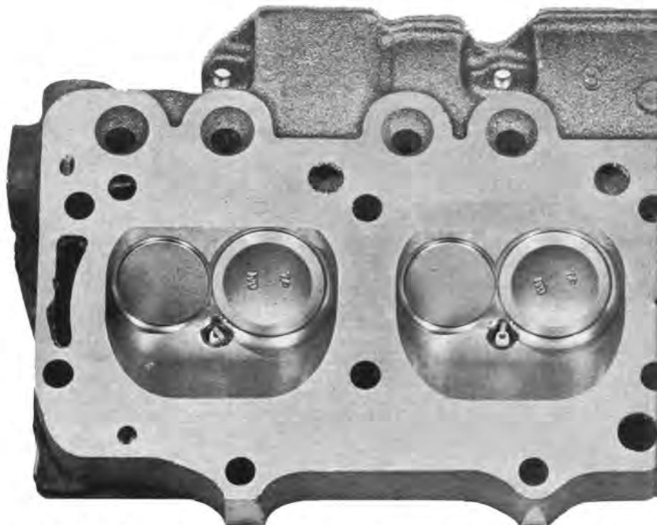
Characteristic Buick combustion chambers, shown in 425 head, are semi-hemispherical.
