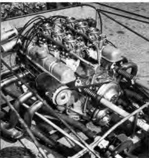
Buick engine in Balchowsky's Mark IV has 430 cu. in., develops 350 hp at 5800 rpm.
