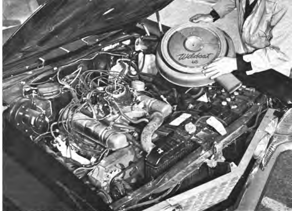
Big 401 produces 325 hp at 4400 rpm and hefty 445 lb/ft of torque at 2800 rpm.
