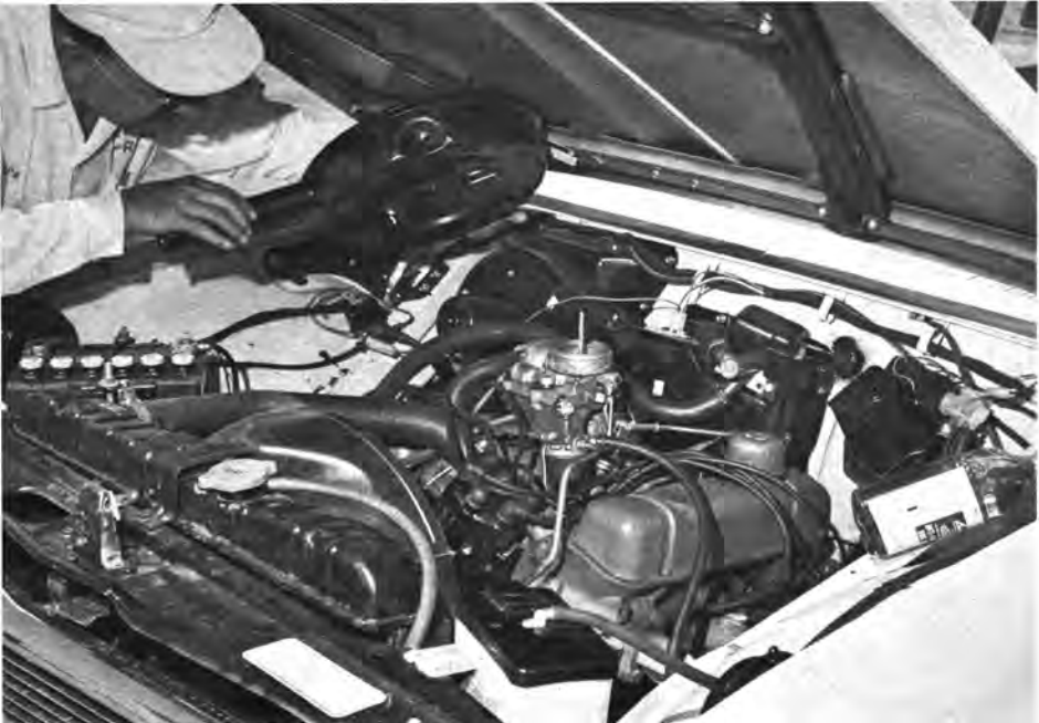
For '63, 401-cu.-in. engine is used in Wildcat (above) and in Riviera (opposite page).
