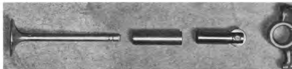
Reworked Pontiac Six valve, roller tappet, stock Buick rocker are used in Scarab-Buick.
