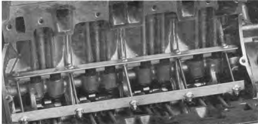
Scarab's roller tappet assemblies are kept securely in place by longitudinal carriage.
