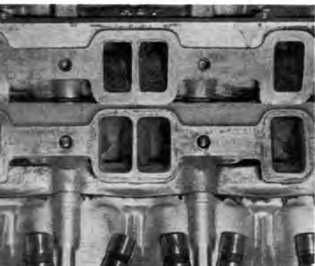
Flow bench was used as guide to breathing improvement in Reventlow motor. Porting of stock Buick (top), Scarab are compared.
