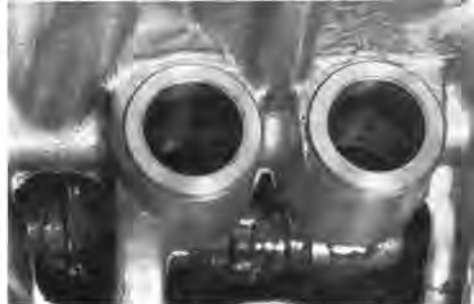
Existing tappet holes were bored to take bronze guides for roller tappet assembly.
