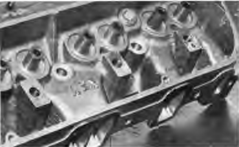
Aluminum-bronze alloy guides were fitted to accommodate Scarab's special valves.
