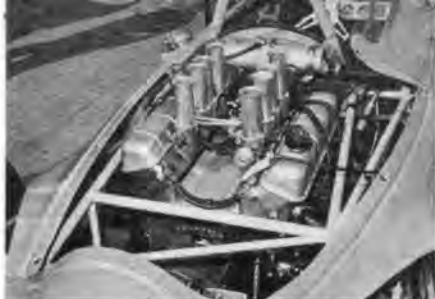
Rear-mounted Thompson Buick displaces 255 cu. in. to meet Indy regulations.
