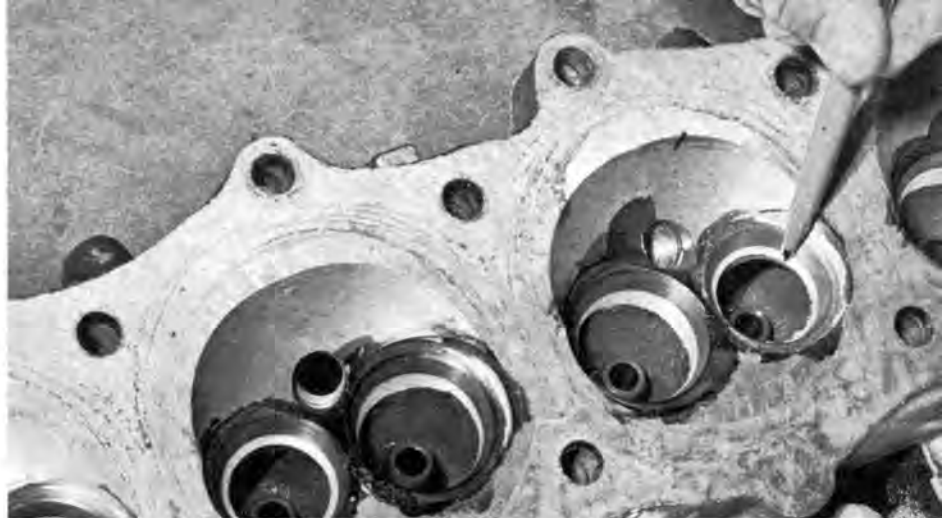
Intake and exhaust pockets were trimmed in Scarab to allow for 1/8-in. larger valves.
