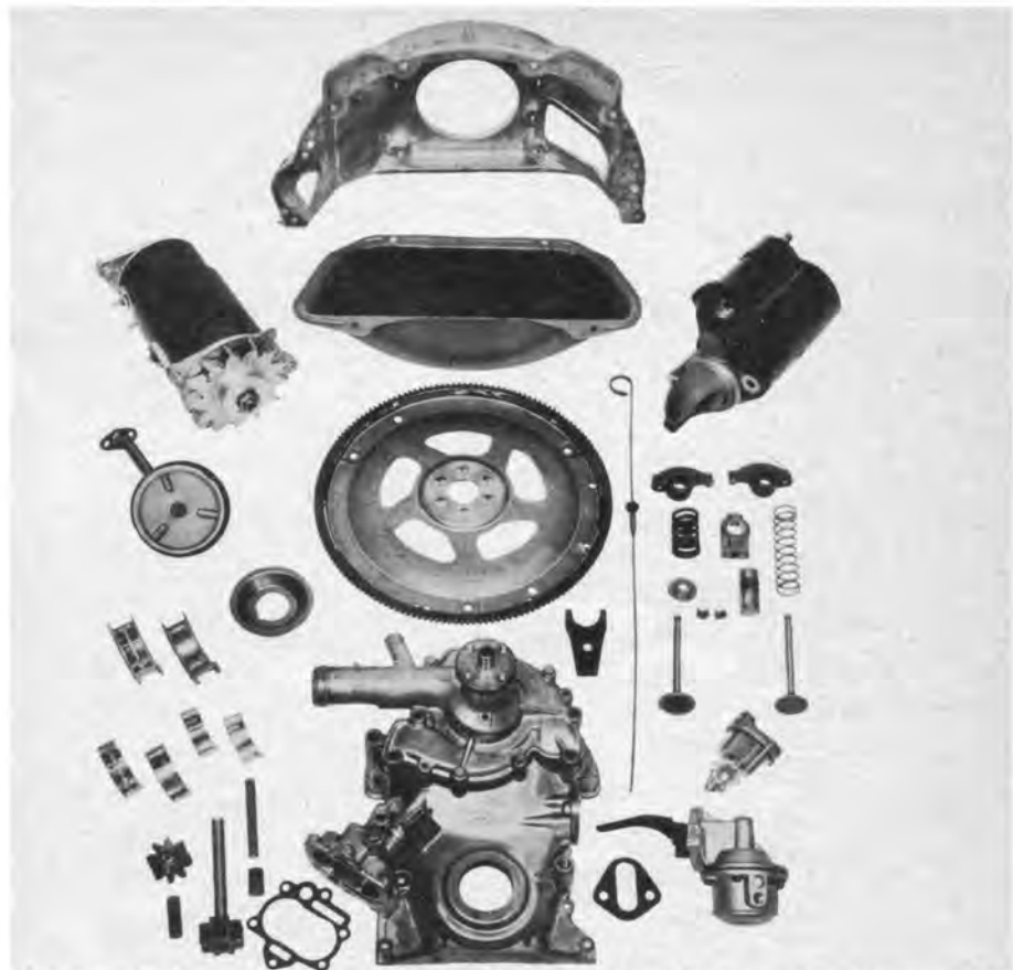
Despite shorter, cast-iron block, V6 is able to borrow parts shown from aluminum V8.
